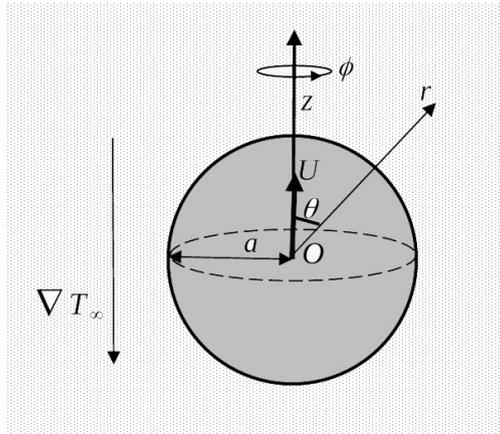
FIG. 1. Physical representation of thermophoresis motion of an aerosol sphere embedded in a porous medium saturated by micropolar fluid.
