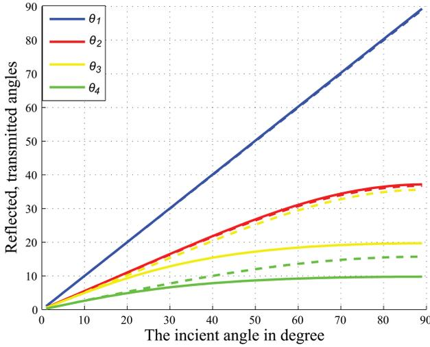
FIG. 7. Phase angles for presence and absence of the initial stress.
