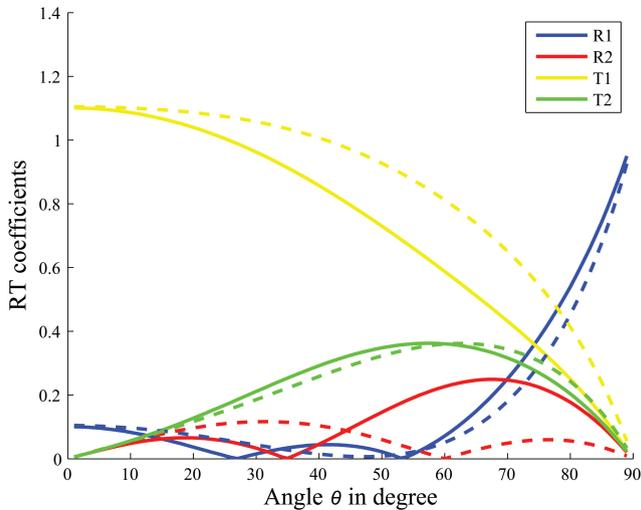
FIG. 3. The effect of the initial stress on the RTCs for the case of the perfect interface.
