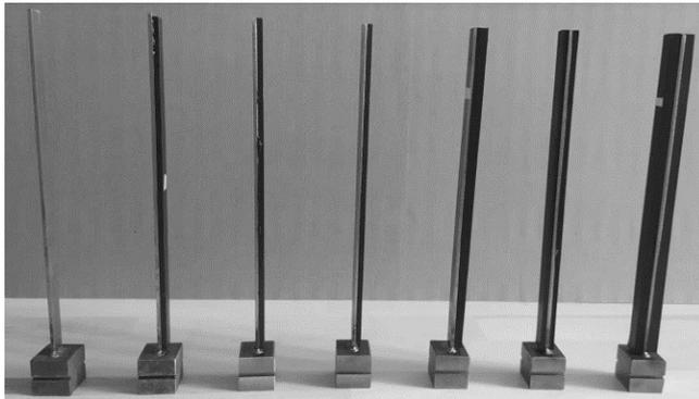
FIG. 5. Examples of the tested steel-core composites.
