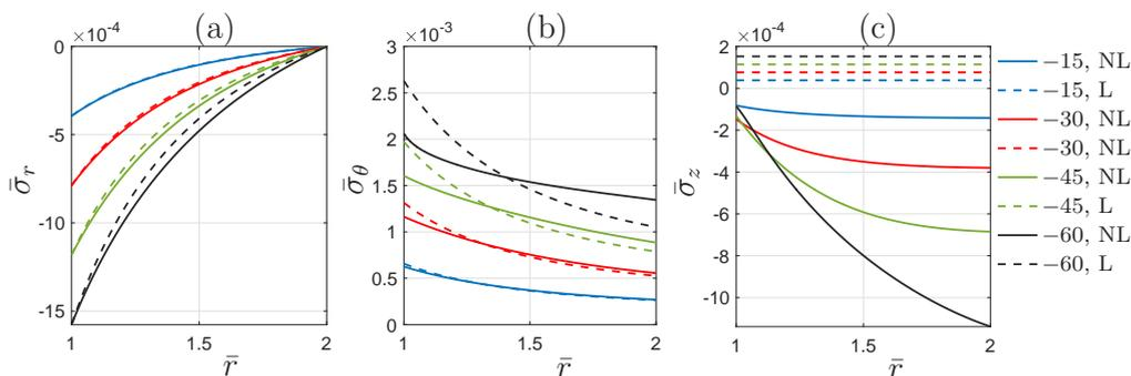
FIG. 14. Results for the dimensionless components of the stress tensor versus the dimensionless radial position for the modelling of concrete. Results are shown for different values of  $P$  [MPa]. The results obtained with (3.4) are denoted ‘NL’, and the results obtained using (3.10) are denoted ‘L’.
