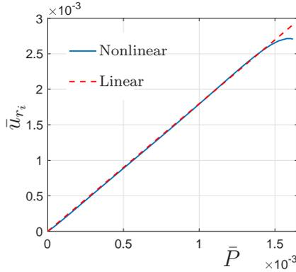
FIG. 16. Modelling of concrete. Behaviour of the dimensionless radial displacement at  $r = r_i$  versus the dimensionless load  $\bar{P}$ .
