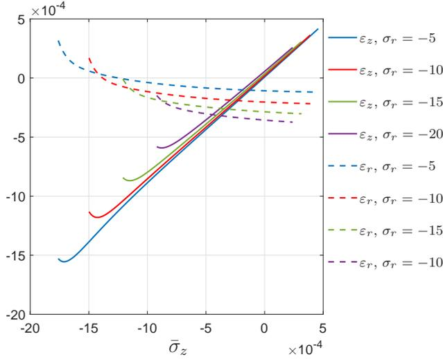
FIG. 4. Results for the triaxial compression of a cylinder considering the model for concrete (4.11), (4.12) and (5.3), (5.4). Case  $f^{(2)} = 0.01f^{(1)}$ ,  $f^{(1)} = 1$  for four values for  $\sigma_r$ . In the different cases  $\sigma_r$  is in [MPa].
