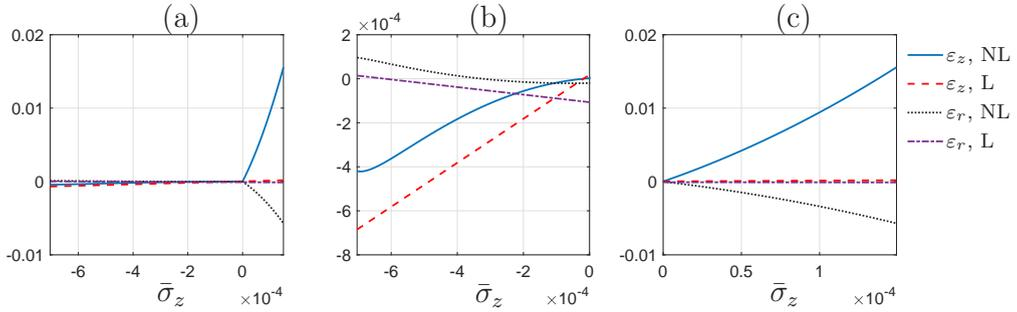
FIG. 11. Predictions for the non-linear model (5.1), (5.2), (5.6), (5.7), (3.4) denoted ‘NL’, and comparison with the predictions of the linearized model (3.10) that is denoted ‘L’, for the problem of triaxial load of a cylinder.
