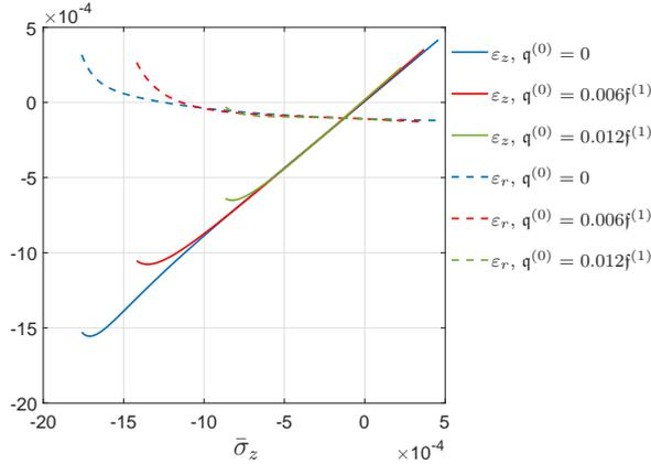
FIG. 6. Results for the triaxial compression of a cylinder considering the model for concrete (5.3), (5.4) and (3.4). Case where it is assumed that  $f^{(2)} = 0.01f^{(1)}$ ,  $f^{(1)} = 1$  and  $\sigma_r = -5$  [MPa]. Case  $h^{(0)} = 0$  and different values for  $q^{(0)}$ .
