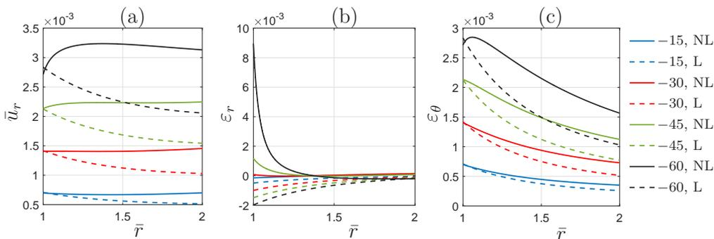
FIG. 15. Results for the dimensionless radial displacement and the components of the strain tensor versus the dimensionless radial position for the modelling of concrete. Results for different values of  $P$  [MPa]. The results obtained using (3.4) are denoted by ‘NL’, and the results obtained using (3.10) are denoted by ‘L’.
