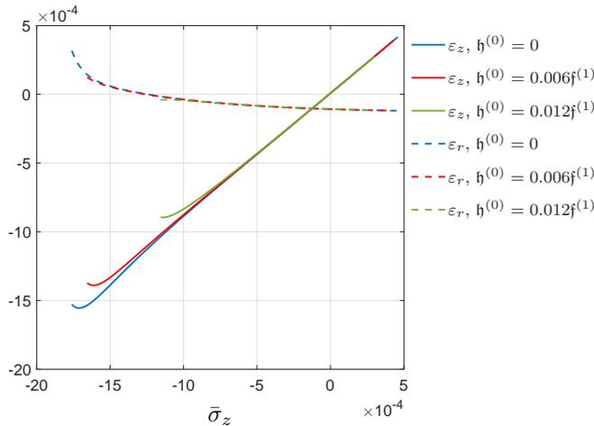
FIG. 5. Results for the triaxial compression of a cylinder considering the model for concrete (5.3), (5.4) and (3.4). Case where it is assumed that  $f^{(2)} = 0.01f^{(1)}$ ,  $f^{(1)} = 1$  and  $\sigma_r = -5$  [MPa], for different values of  $h^{(0)}$  and  $q^{(0)} = 0$ .
