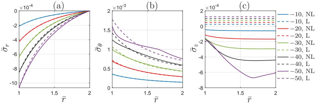
FIG. 17. Results for the dimensionless components of the stress tensor versus the dimensionless radial position in the case of rock. Results for different values of  $P$  [MPa]. The results obtained with (3.4) are denoted ‘NL’, and the results obtained using (3.10) are denoted ‘L’.
