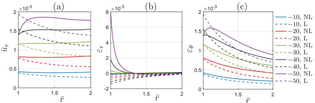
FIG. 18. Results for the dimensionless radial displacement and the components of the strain tensor versus the dimensionless radial position in the case of rock. Results for different values of  $P$  [MPa]. The results obtained with (3.4) are denoted ‘NL’, and the results obtained using (3.10) are denoted ‘L’.
