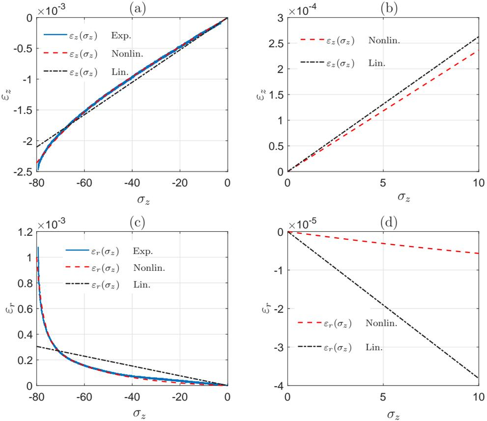
FIG. 1. Comparison of the predictions for the behaviour of concrete, considering the nonlinear model (5.3), (5.4) called ‘Nonlin.’, the linear model (3.10) called ‘Lin.’, with the experimental data from [10], called ‘Exp.’. The axial stress  $\sigma_z$  is in [MPa]. (a,b): results for the axial component of the strain, (c,d): results for the radial component of the strain.
