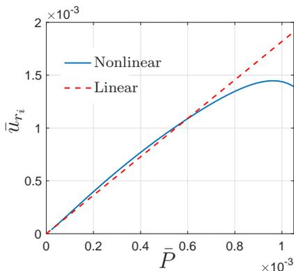
FIG. 19. Modelling of rock. Behaviour of the dimensionless radial displacement at  $r = r_i$  versus the dimensionless load  $\bar{P}$ .
