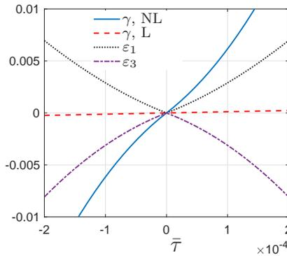
FIG. 12. Predictions for the non-linear model (5.1), (5.2), (5.6), (5.7), (3.5) denoted ‘NL’, and comparison with the predictions of the linearized model (3.10) that is denoted ‘L’, for the problem of simple shear stress of a slab.
