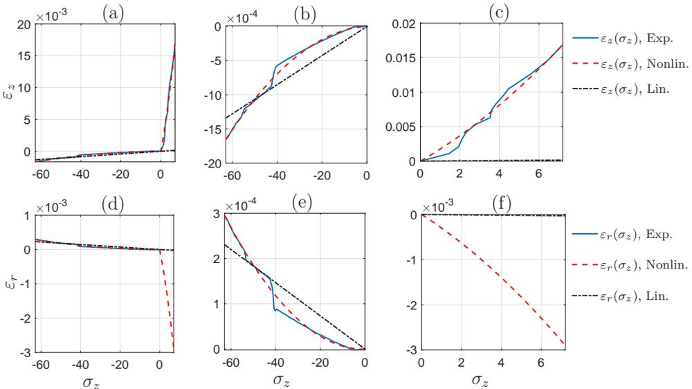
FIG. 8. Comparison of the predictions for the behaviour of rock, for the non-linear model (5.6), (5.7) called ‘Nonlin.’, the linear model (3.10) called ‘Lin.’, with the experimental data from [17], called ‘Exp.’. The axial stress  $\sigma_z$  is in [MPa]. (a, d) Comparison for the whole range of values for  $\sigma_z$ . (b, e) Comparison for the case  $\sigma_z \leq 0$ . (c, f) Comparison for the case  $\sigma_z \geq 0$ .
