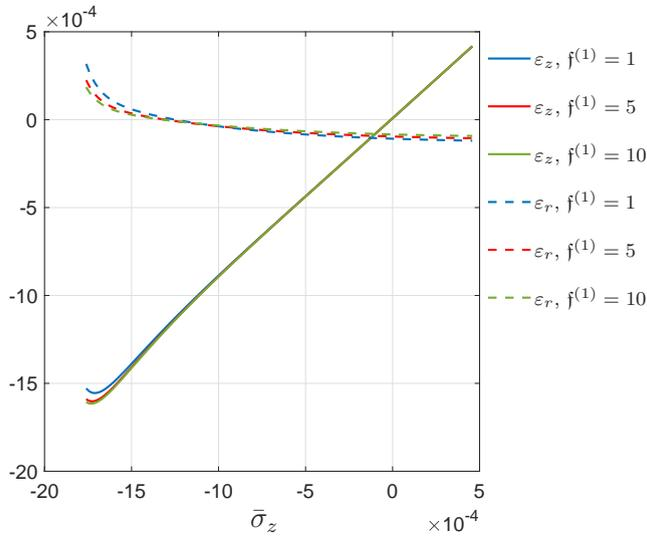
FIG. 3. Results for the triaxial compression of a cylinder considering the model for concrete (4.11), (4.12) and (5.3), (5.4). Case  $f^{(2)} = 0.01f^{(1)}$ ,  $\sigma_r = -5$  [MPa] and considering three values for  $f^{(1)}$ .
