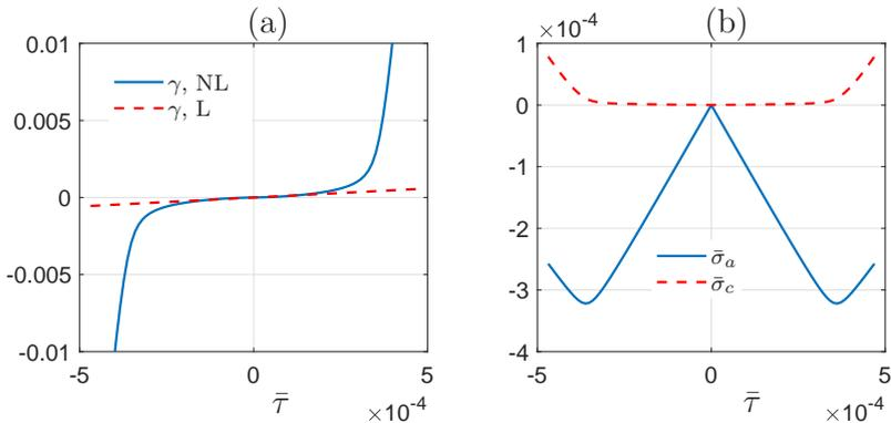
FIG. 13. Predictions for the non-linear model (5.1), (5.2), (5.6), (5.7), (3.5) denoted ‘NL’, and comparison with the predictions of the linearized model (3.10) that is denoted ‘L’, for the problem of simple shear strain of a slab.
