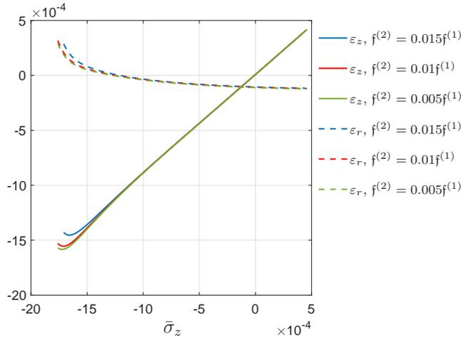
FIG. 2. Results for the triaxial compression of a cylinder considering the model for concrete (4.11), (4.12) and (5.3), (5.4). Case  $f^{(1)} = 1$ ,  $\sigma_r = -5$  [MPa] and different values for  $f^{(2)}$ .
