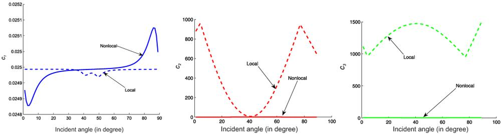
FIG. 10. Comparison of phase velocities with respect to the incident angle  $\theta_0$  for local ( $\epsilon = 0$ ) and nonlocal ( $\epsilon > 0$ ) medium.
