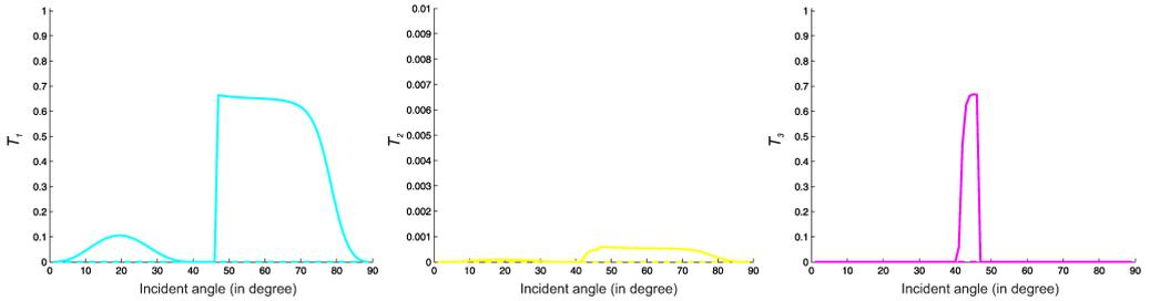
FIG. 5. The transmission coefficients  $T_1, T_2, T_3$  for inhomogeneous and homogeneous incident wave; solid line represents  $D = 2$ , dashed line for  $D = 0$ .
