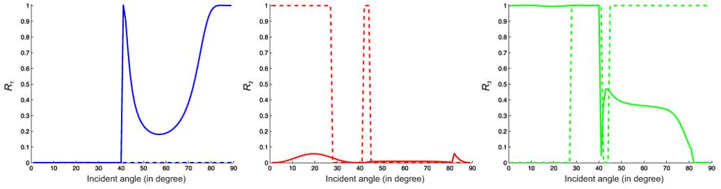
FIG. 4. The reflection coefficients  $R_1, R_2, R_3$  for inhomogeneous and homogeneous incident wave; solid line represents  $D = 2$ , dashed line for  $D = 0$ .
