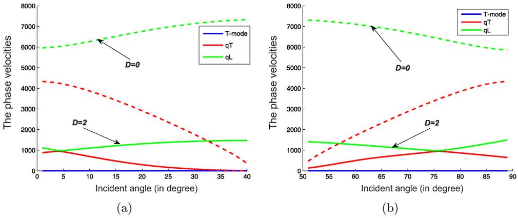
FIG. 2. Variations in phase velocities of incident waves with phase direction  $\theta_0$  for two cases:  $D = 2$  and  $D = 0$ .
