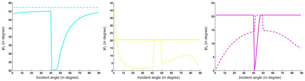
FIG. 9. The attenuation angle of transmitted waves for inhomogeneous and homogeneous incident wave; solid line represents  $D = 2$ , dashed line for  $D = 0$ .
