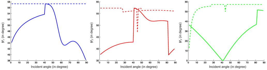
FIG. 8. The attenuation angle of reflected waves for inhomogeneous and homogeneous incident wave; solid line represents  $D = 2$ , dashed line for  $D = 0$ .
