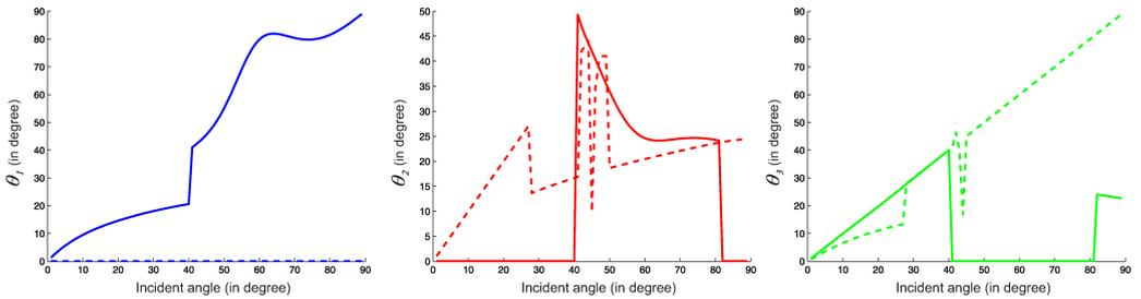
FIG. 6. The phase direction of reflected waves for inhomogeneous and homogeneous incident wave; solid line represents  $D = 2$ , dashed line for  $D = 0$ .
