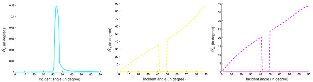
FIG. 7. The phase direction of transmitted waves for inhomogeneous and homogeneous incident wave; solid line represents  $D = 2$ , dashed line for  $D = 0$ .
