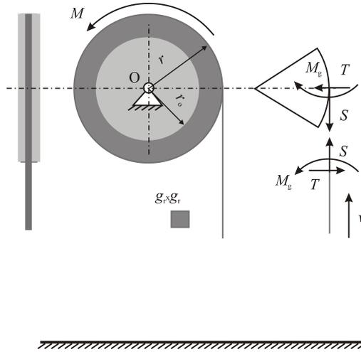
FIG. 7. Illustration for Example 3 along with the internal forces in the rope.
