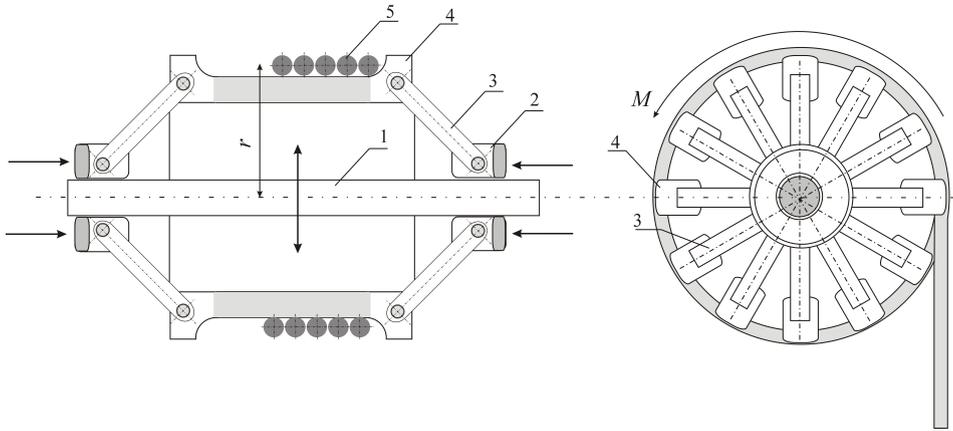
FIG. 12. Illustration of the drum with regulated radius.
