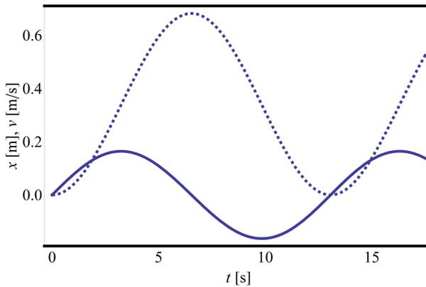
FIG. 11. The case with the radial winding up of the rope – the variation of  $x$  (dashed line) and velocity  $v$  (continuous line) in time for  $g_r = 4.4$  cm when  $M_g$  is taken into account.
