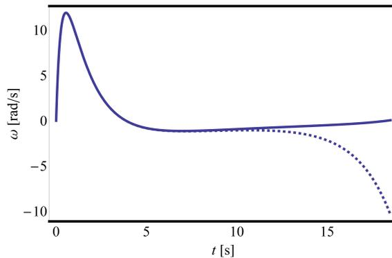
FIG. 14. The drum with the regulated radius – the variation of drum angular velocity  $\omega$  in time for  $M = 40.254$  Nm (continuous line) and  $M = 40.25$  Nm (dashed line).
