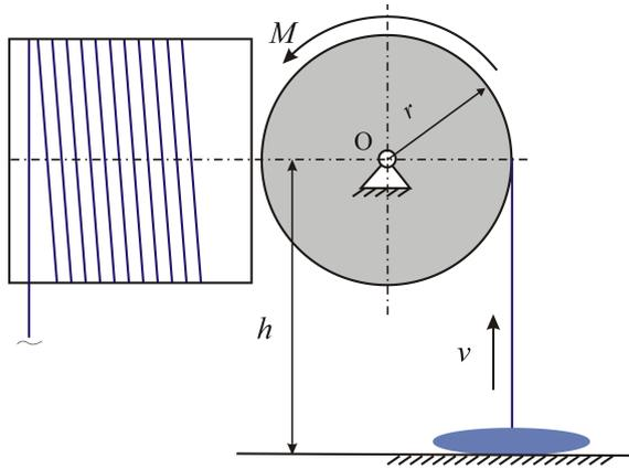
FIG. 4. Scheme of the system in Example 2 with circumferential winding of the rope onto the winch drum.
