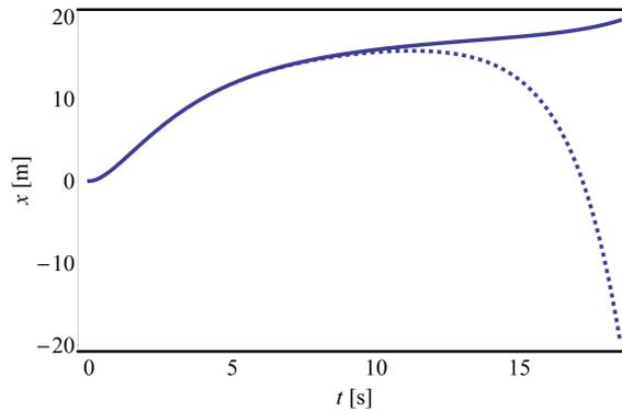
FIG. 13. The drum with the regulated radius – the variation of  $x$  in time for  $M = 40.254$  Nm (continuous line) and  $M = 40.25$  Nm (dashed line).
