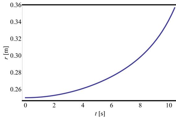
FIG. 10. The case with the radial rope winding – the variation of the drum radius in time for  $g_r = 2$  cm when  $M_g$  is taken into account.
