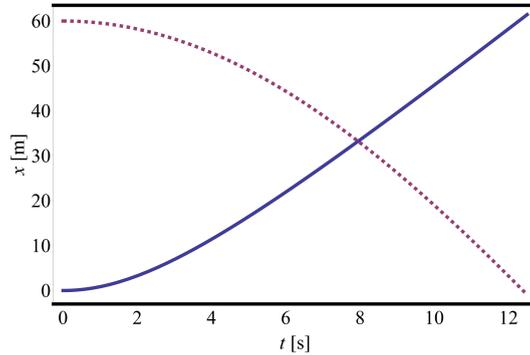
FIG. 5. The solution when the rope is wound up onto the drum (continuous line) and when the rope is unwound from the drum (dashed line).
