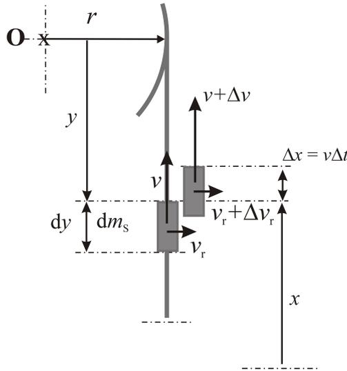
FIG. 8. The illustration for derivation of the angular momentum term corresponding to the horizontal motion of the rope.
