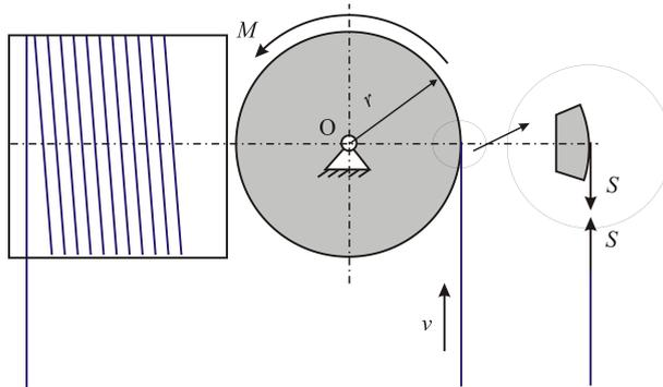
FIG. 2. The scheme of the system in case 1 with circumferential winding of the rope onto the winch drum.
