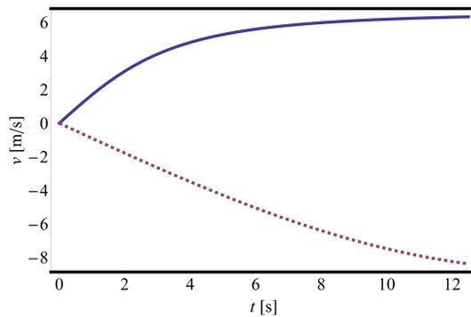
FIG. 6. The rope velocity when the rope is wound up onto the drum (continuous line) and when the rope is unwound from the drum (dashed line).
