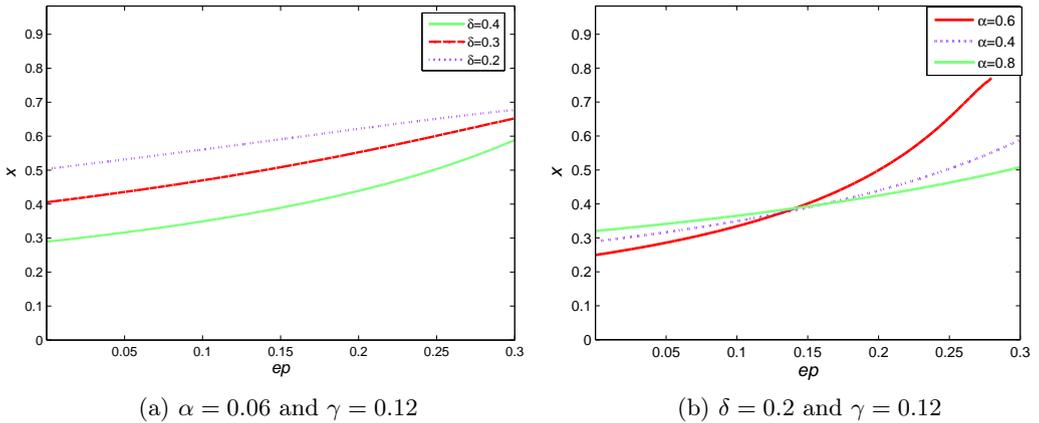
FIG. 7. Variation of non-dimensional speed  $x$  of Rayleigh wave against non-dimensional constant  $ep$ .
