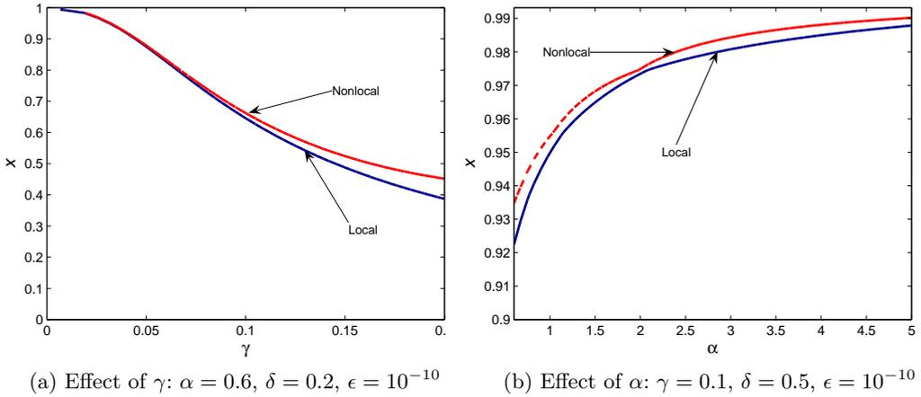
FIG. 5. Effect of  $\gamma, \alpha$  parameter on the non-dimensional speed of Rayleigh wave  $x$  for nonlocal and local orthotropic half-space.
