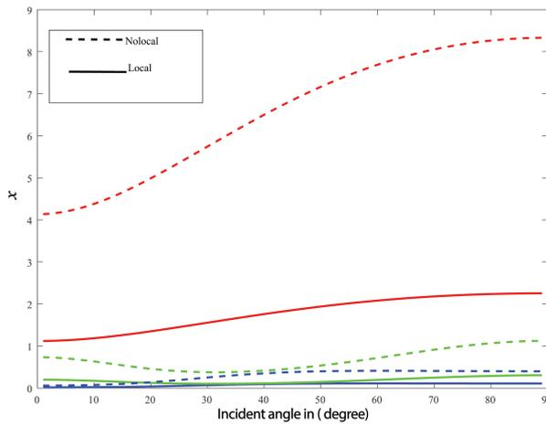
FIG. 1. Variation of the non-dimensional speeds of Rayleigh wave  $x$  on the incident angle  $\theta_0$  for the local micropolar, nonlocal micropolar.
