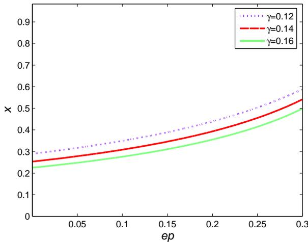
FIG. 8. Variation of non-dimensional speed against non-dimensional constant  $ep$  when  $\alpha = 0.06$  and  $\delta = 0.2$ .
