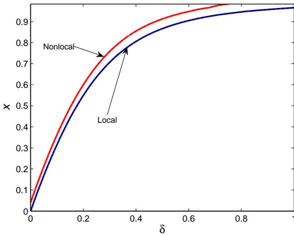
FIG. 6. Effect of  $\delta$  parameter on the non-dimensional speed of Rayleigh wave  $x$  for nonlocal and local orthotropic half-space with  $\gamma = 0.1, \alpha = 0.3, \epsilon = 10^{-10}$ .
