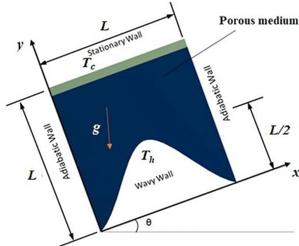
FIG. 1. Schematic of inclined cavity.
