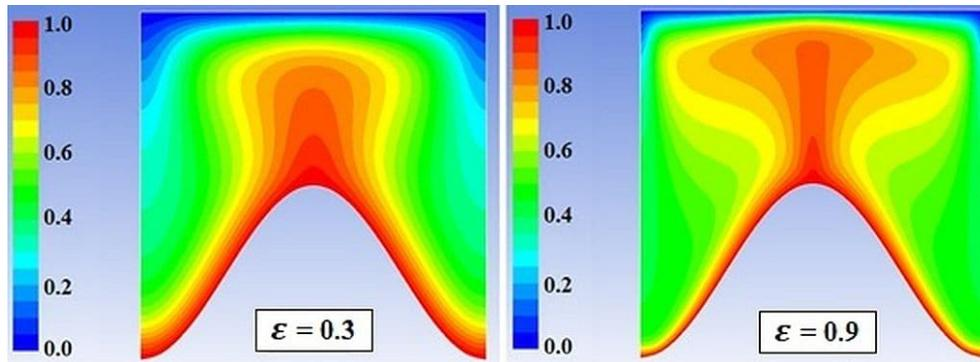
FIG. 8. Comparison of isothermal contours ( $T^*$ ) for porosities of 0.3 and 0.9 at the Rayleigh number of  $10^4$ .
