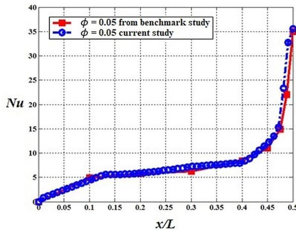
FIG. 4. Comparison of the numerical and empirical Nusselt number profiles for the Rayleigh number of  $10^5$  and volume fraction of 0.05% Cu-Water nanofluid with the benchmark study [33].
