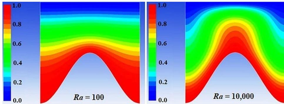
FIG. 6. Isothermal contours ( $T^*$ ) for 0.25% mixture of Cu-Water nanofluid at different Rayleigh numbers.
