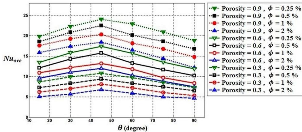
FIG. 10. Effect of inclination angle on the averaged Nusselt number for a range of volume fractions from 0.25% to 2% and for different porosities.
