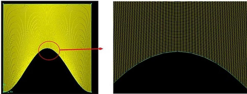
FIG. 2. Generated mesh for solution domain.
