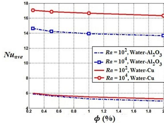
FIG. 5. Variation of the averaged Nusselt number along the centerline of the cavity with volume fraction of nanofluids for two nanofluids at different Rayleigh numbers.
