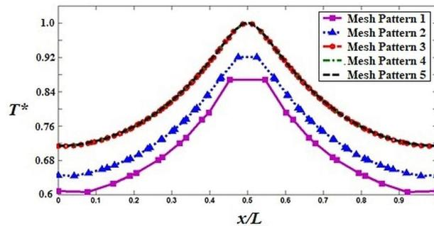
FIG. 3. The temperature profile for different mesh patterns at  $y = L/2$ .
