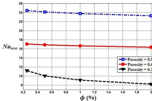
FIG. 7. Effect of porosity on the heat transfer rate for Cu-Water nanofluid at the Rayleigh number of  $10^4$ .
