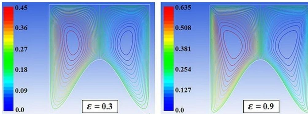
FIG. 9. Comparison of stream function contours for porosities of 0.3 and 0.9 at the Rayleigh number of  $10^4$ .
