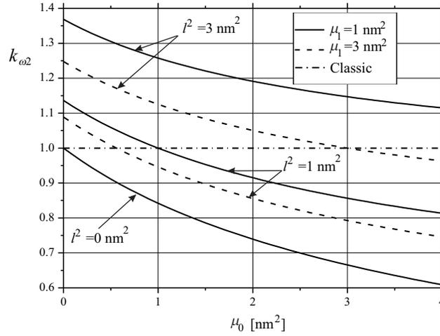
FIG. 7. Variation of the frequency ratio for the second nondimensional frequency of the SS FG nanobeam with respect to the nonlocal parameter  $\mu_0$  for different values of  $\mu_1$  and  $l^2$  and LNR ( $p = 1$ ,  $L/h = 20$ ).
