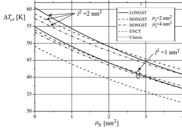
FIG. 2. Variation of the critical buckling temperature of the SS FG nanobeam with respect to the nonlocal parameter  $\mu_0$  for different values of the nonlocal parameter  $\mu_1$ , the strain length scale  $l$  and LNR ( $p = 1$ ,  $L/h = 50$ ).
