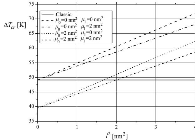
FIG. 4. Variation of the critical buckling temperature of the SS FG nanobeam with respect to the strain length scale  $l$  for different values of the nonlocal parameter  $\mu_0$ , nonlocal parameter  $\mu_1$  and LNR ( $p = 1$ ,  $L/h = 50$ ).
