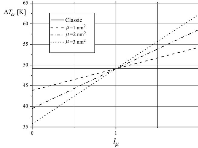
FIG. 5. Variation of the critical buckling temperature of the SS FG nanobeam with respect to ratio  $l_\mu$ , strain length scale for different values of the nonlocal parameters and LNR ( $p = 1, L/h = 50, \mu_0 = \mu_1 = \mu$ ).
