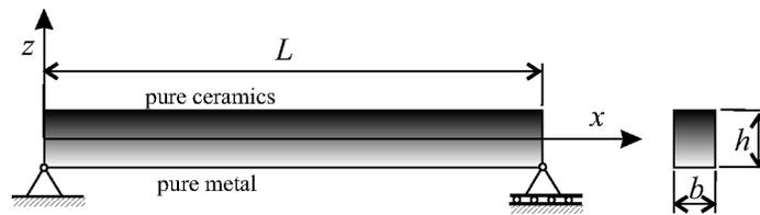
FIG. 1. Geometry and coordinates of the functionally graded beam.
