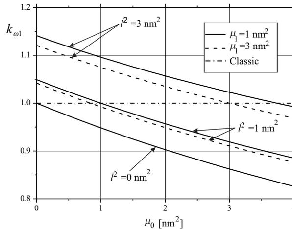
FIG. 6. Variation of the frequency ratio for the first nondimensional frequency of the SS FG nanobeam with respect to the nonlocal parameter  $\mu_0$  for different values of  $\mu_1$  and  $l^2$  and LNR ( $p = 1$ ,  $L/h = 20$ ).
