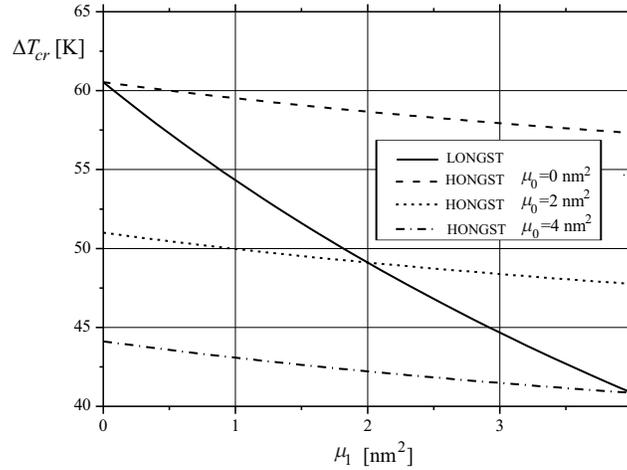
FIG. 3. Variation of the critical buckling temperature of the SS FG nanobeam with respect to the nonlocal parameter  $\mu_1$  for different values of nonlocal parameter  $\mu_0$  and LNR ( $l^2 = 2 \text{ nm}^2$ ,  $p = 1$ ,  $L/h = 50$ ).
