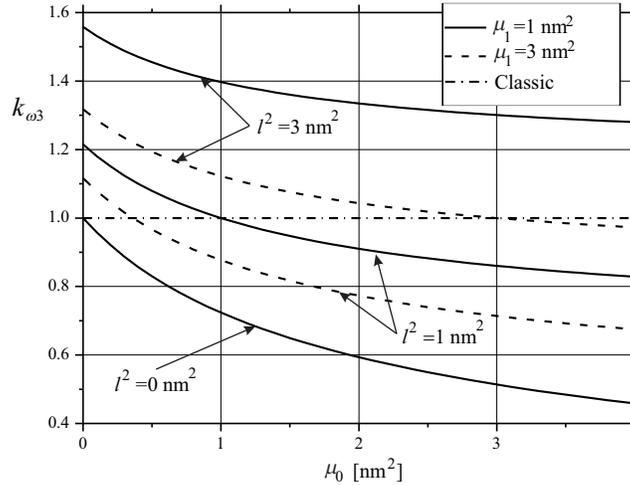
FIG. 8. Variation of the frequency ratio for the third nondimensional frequency of the SS FG nanobeam with respect to the nonlocal parameter  $\mu_0$  for different values of  $\mu_1$  and  $l^2$  and LNR ( $p = 1$ ,  $L/h = 20$ ).
