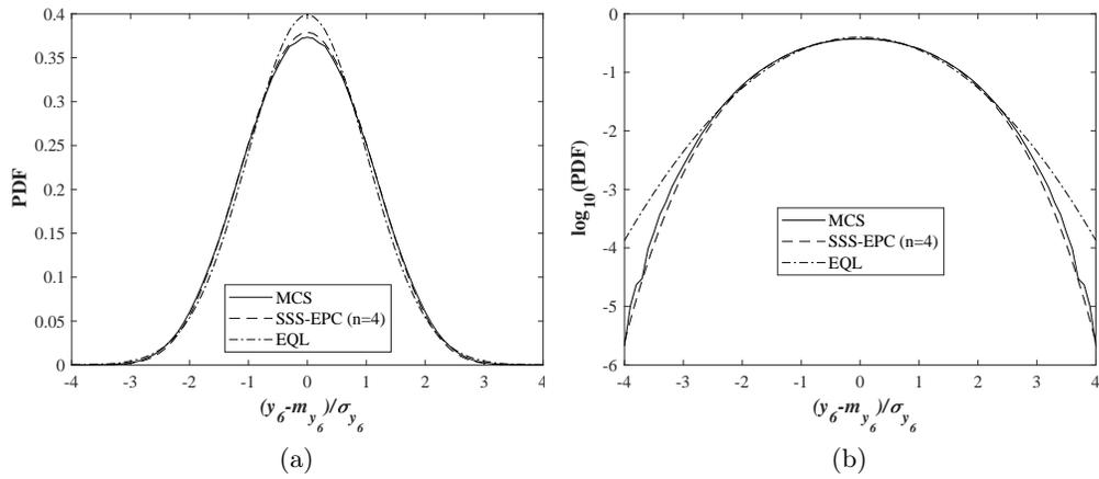
FIG. 8. (a) The PDFs of the deflection  $Y_6$  under uniformly distributed load over the whole beam. (b) The logarithm of PDFs of the deflection  $Y_6$  under uniformly distributed load over the whole beam.
