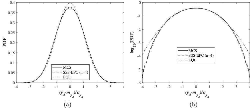
FIG. 6. (a) The PDFs of the deflection  $Y_4$  under uniformly distributed load over the whole beam. (b) The logarithm of PDFs of the deflection  $Y_4$  under uniformly distributed load over the whole beam.
