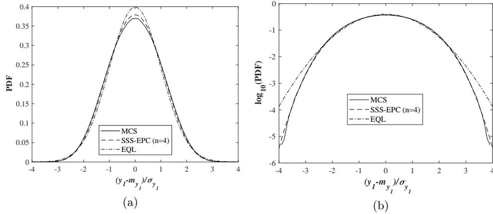
FIG. 11. (a) The PDFs of the deflection  $Y_1$  under partially distributed load over the whole beam. (b) The logarithm of PDFs of the deflection  $Y_1$  under partially distributed load over the whole beam.
