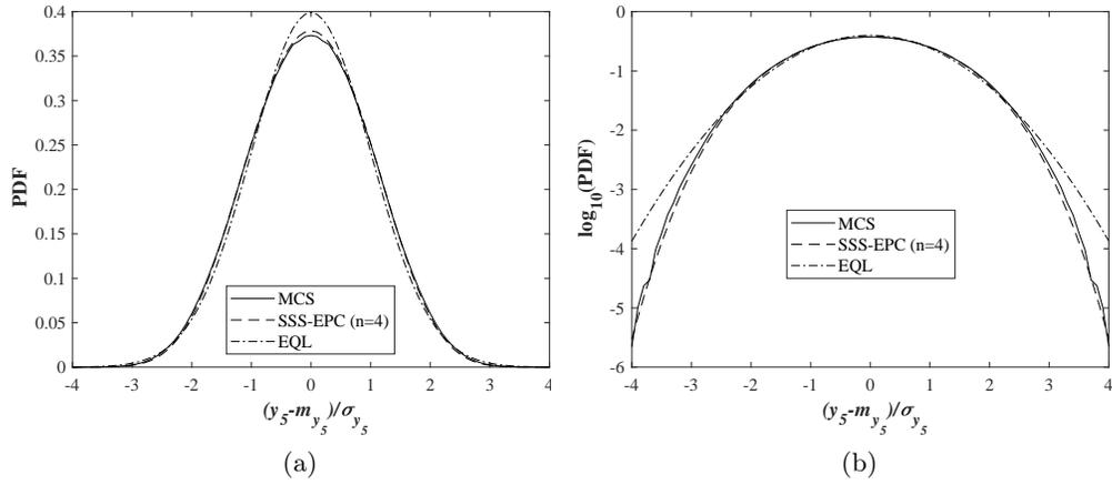
FIG. 7. (a) The PDFs of the deflection  $Y_5$  under uniformly distributed load over the whole beam. (b) The logarithm of PDFs of the deflection  $Y_5$  under uniformly distributed load over the whole beam.
