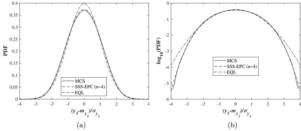
FIG. 13. (a) The PDFs of the deflection  $Y_3$  under partially distributed load over the whole beam. (b) The logarithm of PDFs of the deflection  $Y_3$  under partially distributed load over the whole beam.
