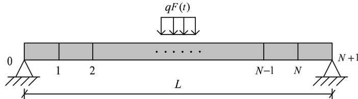
FIG. 10. Finite difference model of beam under partially distributed load in the middle of the beam.
