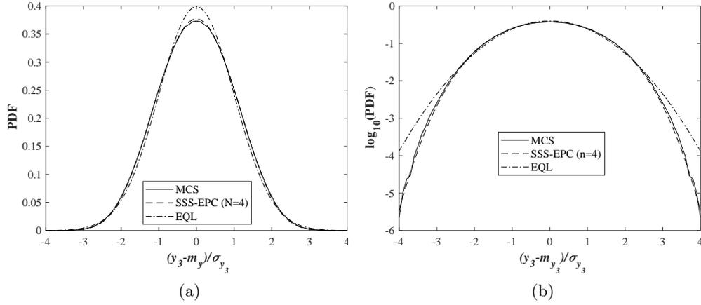
FIG. 5. (a) The PDFs of the deflection  $Y_3$  under uniformly distributed load over the whole beam. (b) The logarithm of PDFs of the deflection  $Y_3$  under uniformly distributed load over the whole beam.
