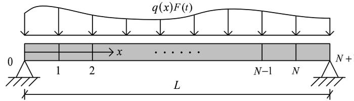
FIG. 1. Finite difference model of the stretched beam under distributed random force.
