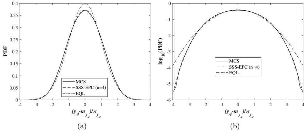
FIG. 14. (a) The PDFs of the deflection  $Y_4$  under partially distributed load over the whole beam. (b) The logarithm of PDFs of the deflection  $Y_4$  under partially distributed load over the whole beam.
