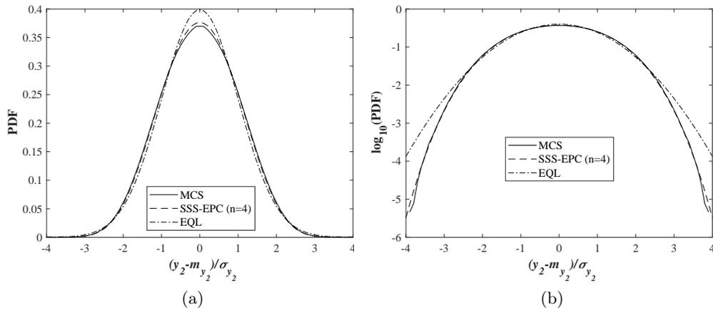
FIG. 12. (a) The PDFs of the deflection  $Y_2$  under partially distributed load over the whole beam. (b) The logarithm of PDFs of the deflection  $Y_2$  under partially distributed load over the whole beam.
