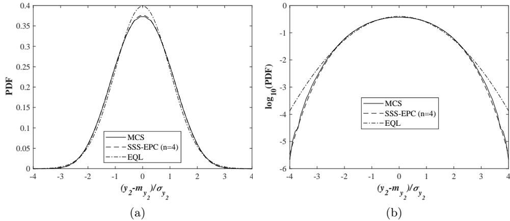
FIG. 4. (a) The PDFs of the deflection  $Y_2$  under uniformly distributed load over the whole beam. (b) The logarithm of PDFs of the deflection  $Y_2$  under uniformly distributed load over the whole beam.
