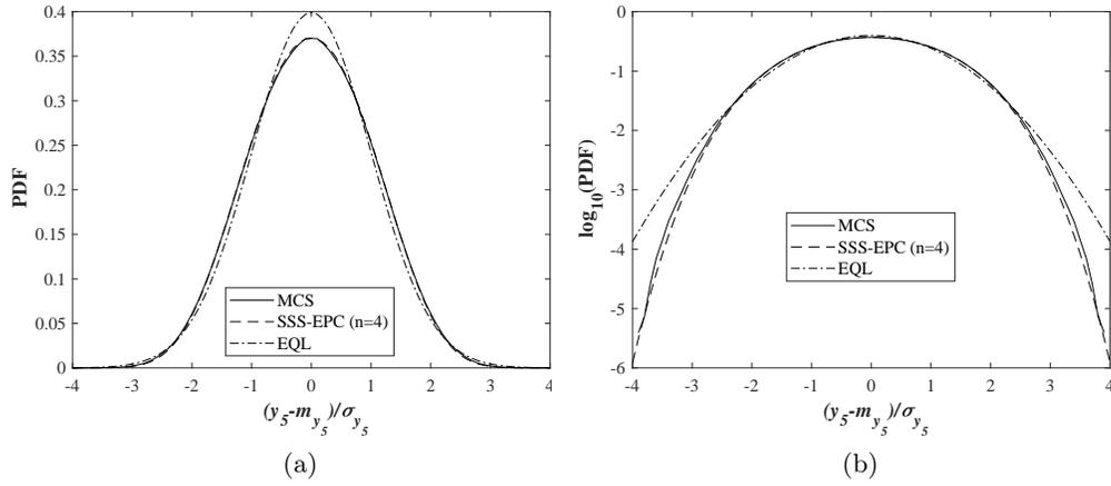
FIG. 15. (a) The PDFs of the deflection  $Y_5$  under partially distributed load over the whole beam. (b) The logarithm of PDFs of the deflection  $Y_5$  under partially distributed load over the whole beam.
