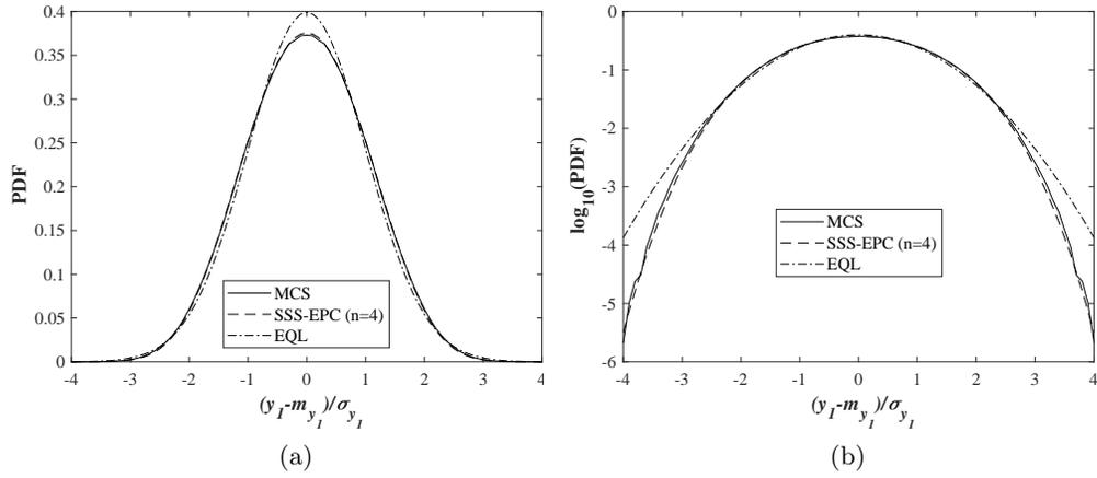
FIG. 3. (a) The PDFs of the deflection  $Y_1$  under uniformly distributed load over the whole beam. (b) The logarithm of PDFs of the deflection  $Y_1$  under uniformly distributed load over the whole beam.
