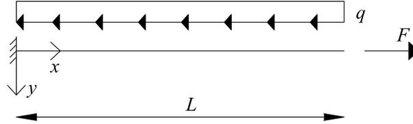
FIG. 3. Cantilever beam (bar type FE).
