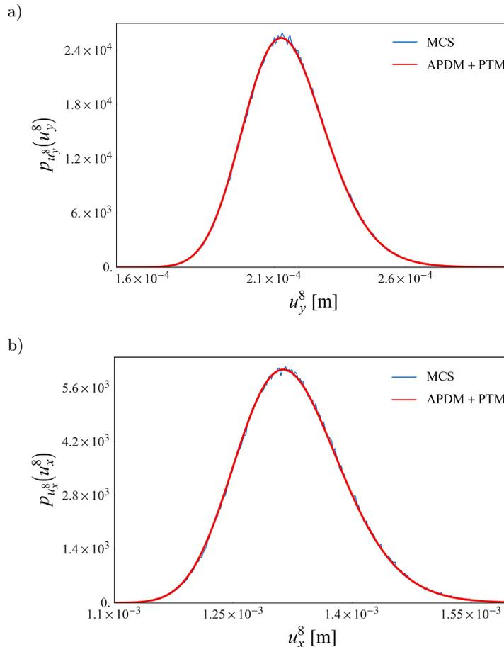
FIG. 10. PDF of the vertical (a) and horizontal (b) displacement of node 8. Uncorrelated random variables  $\alpha_i$ .
