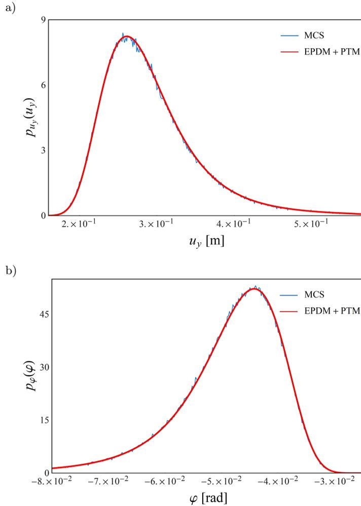
FIG. 7. PDF of the vertical displacement (a) and rotation (b) of the cantilever free end; correlated random variables  $\alpha_i$ .
