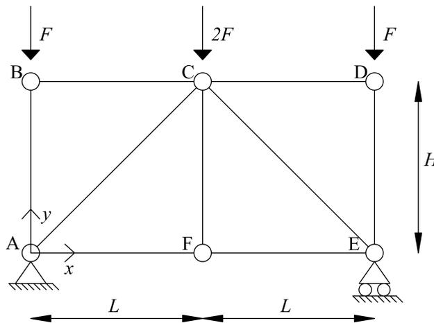
FIG. 1. The truss-structure.
