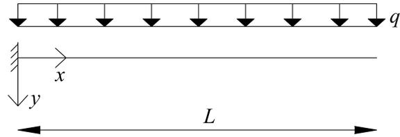
FIG. 5. Cantilever beam (beam-type FE).
