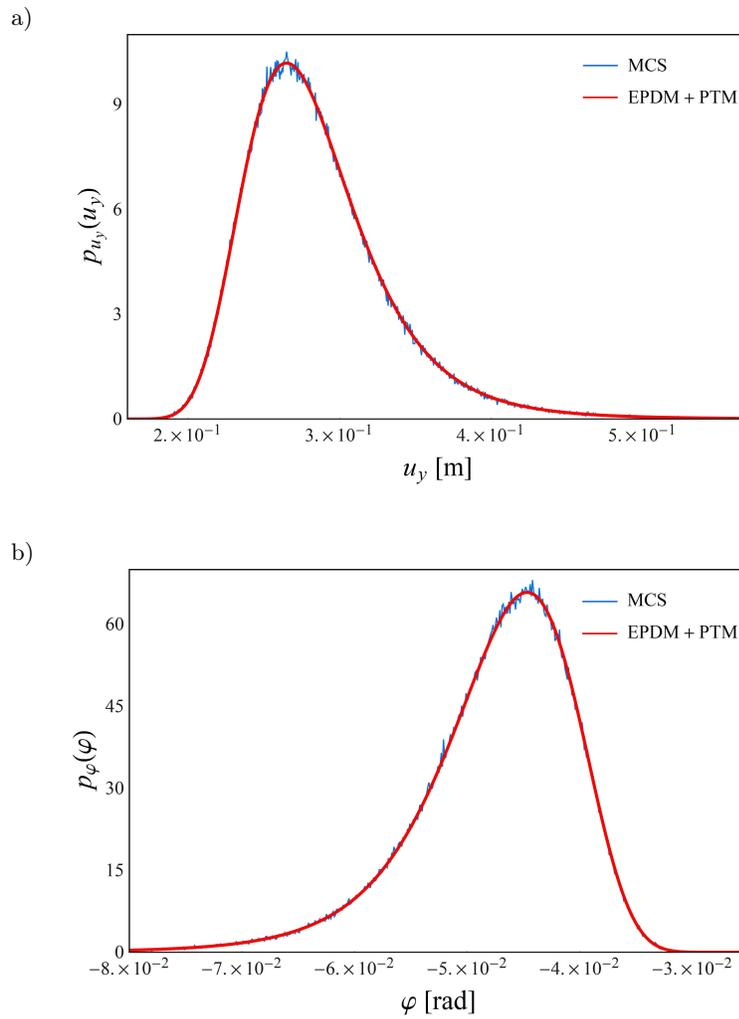
FIG. 6. PDF of the vertical displacement (a) and rotation (b) of the cantilever free end; uncorrelated random variables  $\alpha_i$ .
