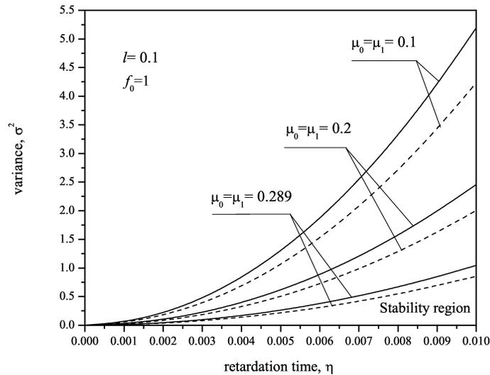
FIG. 3. Stability regions of a nanobeam for the Gaussian and harmonic process as a function of scale coefficients.
