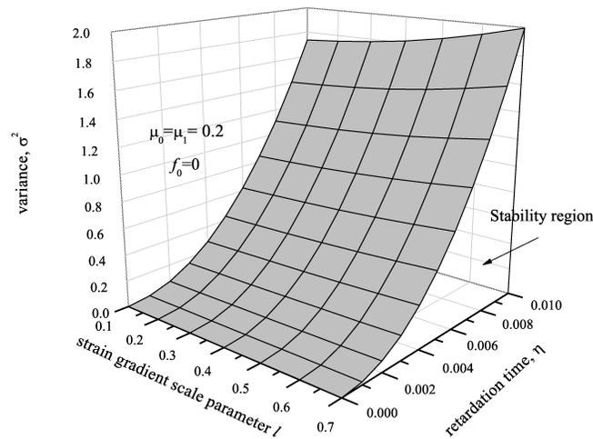
FIG. 7. Stability surface of a nanobeam for the harmonic process in the function of the strain gradient parameter.
