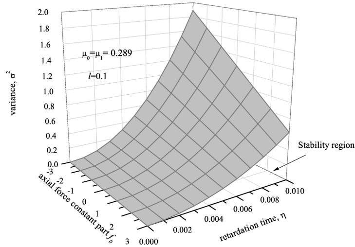
FIG. 4. Stability surface of a nanobeam for the Gaussian process in the function of the constant component of axial force.
