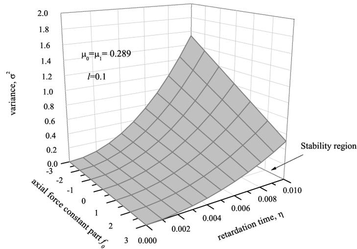
FIG. 5. Stability surface of a nanobeam for the harmonic process in the function of the constant component of axial force.
