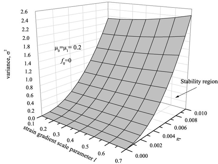
FIG. 6. Stability surface of a nanobeam for the Gaussian process in the function of the strain gradient parameter.
