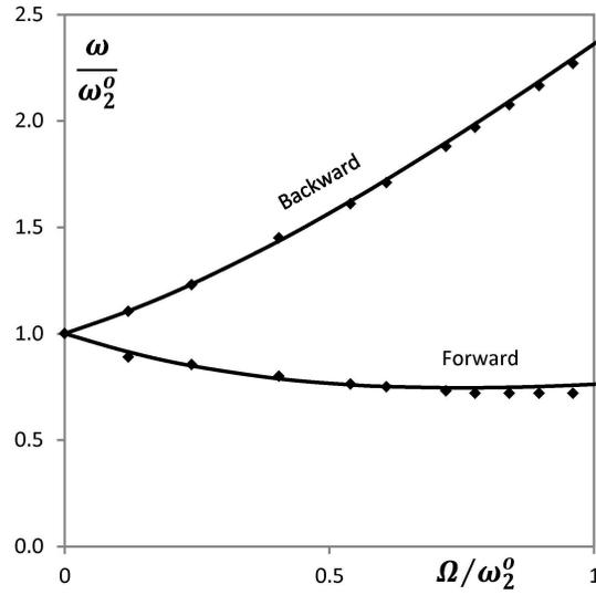
FIG. 7. Comparison of dimensionless natural frequencies of rotating thin ring,  $n = 2$ , — theoretical, Eq. (A17),  $\diamond$  measured, [15].
