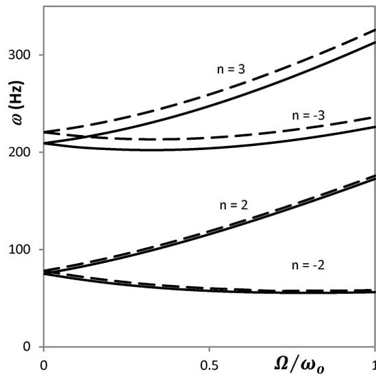
FIG. 6. Natural frequencies of rotating toroidal ring, in-plane vibrations, — FEM, - - - analytical, (Table 5).
