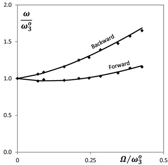
FIG. 8. Comparison of dimensionless natural frequencies of rotating thin ring,  $n = 3$ , — theoretical, Eq. (A17),  $\diamond$  measured, [15].
