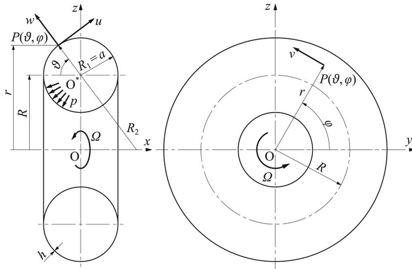
FIG. 1. Rotating toroidal shell, main dimensions and displacements.
