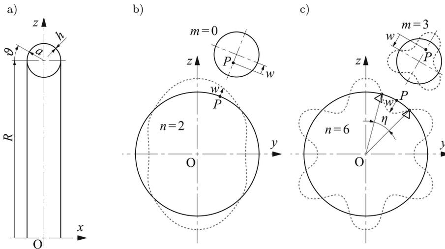
FIG. 2. Thin-walled toroidal ring.
