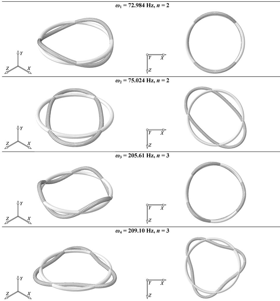
FIG. 4. Natural modes of thin-walled toroidal ring (Abaqus).
