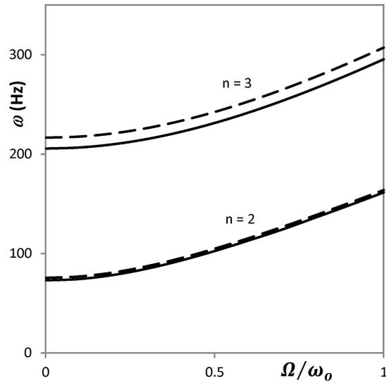
FIG. 5. Natural frequencies of rotating toroidal ring, out-of-plane vibrations, — FEM, - - - analytical, (Table 5).
