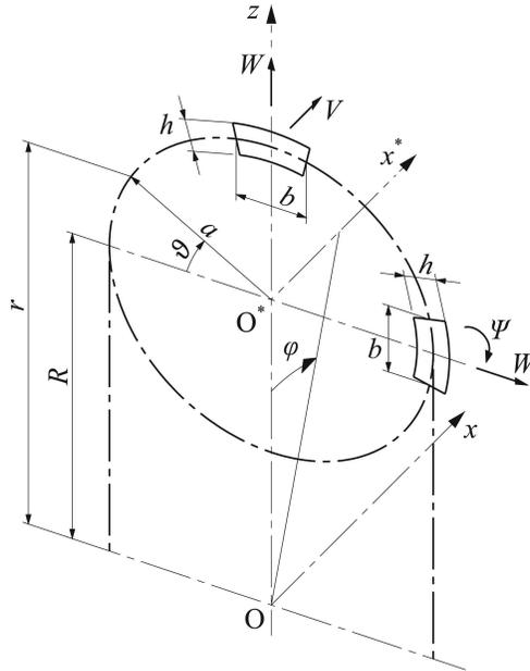
FIG. 3. Toroidal shell segments as rings.
