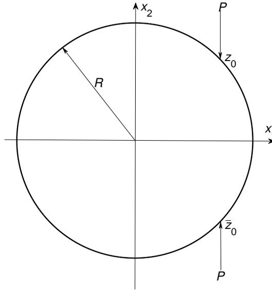
FIG. 1. A circular disk of radius  $R$  with two equal and opposite vertical forces  $P$  being applied at  $z = z_0$  and  $z = \bar{z}_0$  on its surface.
