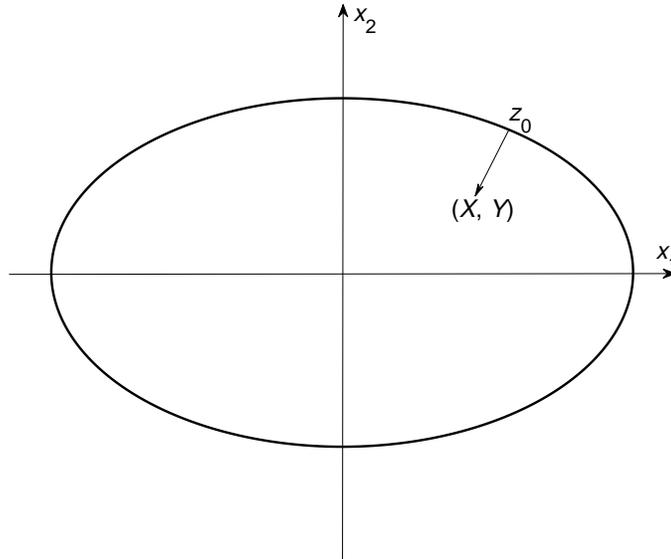
FIG. 3. An unbounded region weakened by an elliptical hole.
