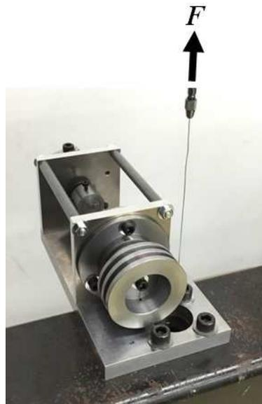
FIG. 3. Torsion testing device operated by tension tester.
