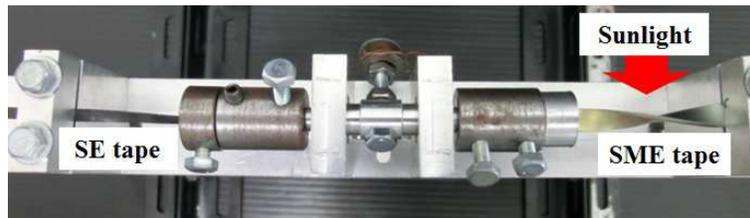
FIG. 8. Photograph of driving part in reciprocating rotary element of solar-powered blind.
