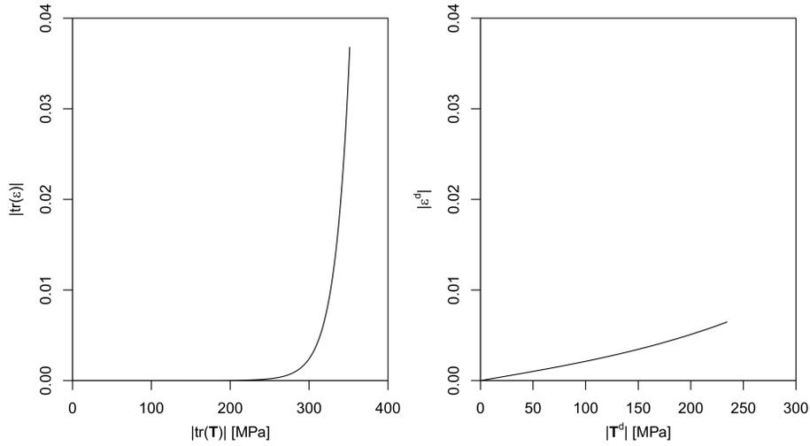
FIG. 9. Bulk and shear response (4.1) of the model (3.1)–(3.2) for *Ti-30Nb-12Zr* alloy.
