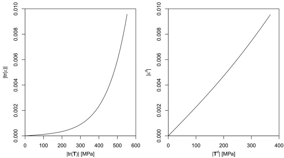
FIG. 7. Bulk and shear response (4.1) of the model (3.1)–(3.2) for *Ti-30Nb-10Ta-5Zr* alloy.
