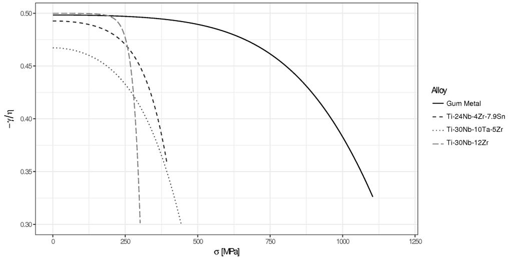
FIG. 13. The ratio  $-\gamma/\eta$  (4.2) for all alloys under the assumption  $|s - 2| > |q - 2|$ .
