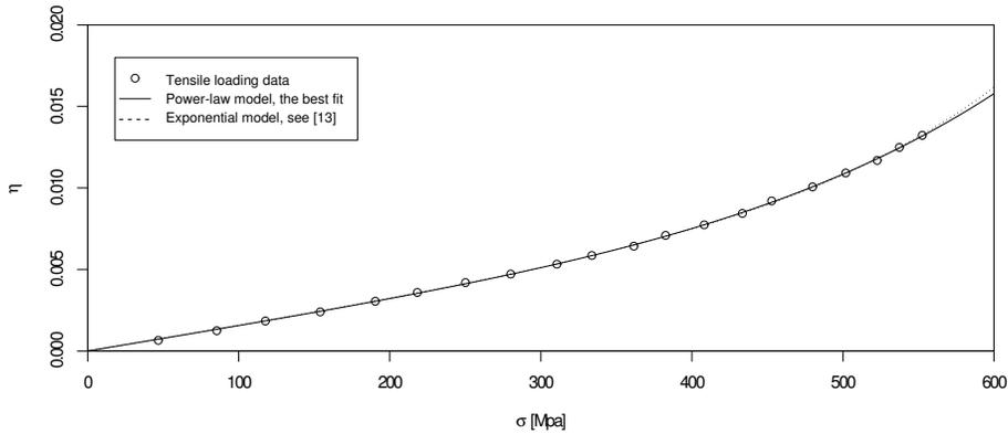
FIG. 3. Plot of the best fit for the model (3.5) compared with the exponential model (2.9) for *Ti-30Nb-10Ta-5Zr*, see [13].
