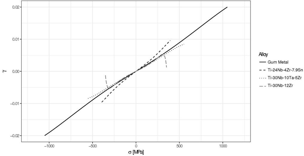
FIG. 12. Transversal strain  $\gamma$  under the assumption  $|s - 2| < |q - 2|$ .
