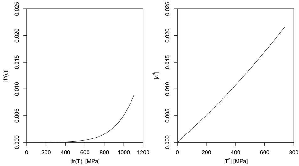
FIG. 6. Bulk and shear response (4.1) of the model (3.1)–(3.2) for Gum Metal.
