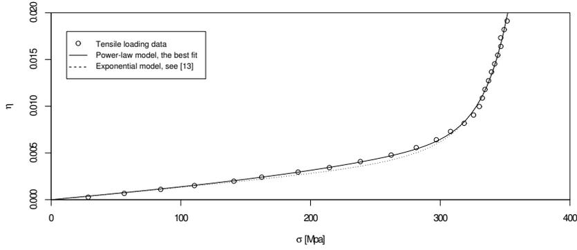
FIG. 5. Plot of the best fit for the model (3.5) compared with the explicit exponential model (2.9) for  $Ti-30Nb-12Zr$ , see [13].
