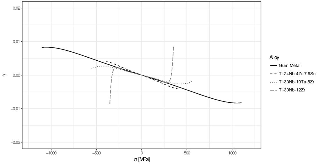
FIG. 11. Transversal strain  $\gamma$  for all alloys under the assumption  $|s - 2| > |q - 2|$ .
