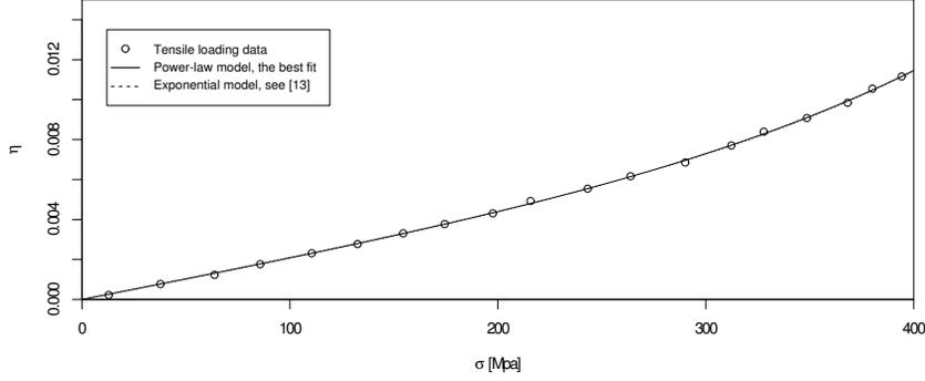
FIG. 4. Plot of the best fit for the model (3.5) compared with the explicit exponential model (2.9) for  $Ti-24Nb-4Zr-7.9Sn$ , see [13].
