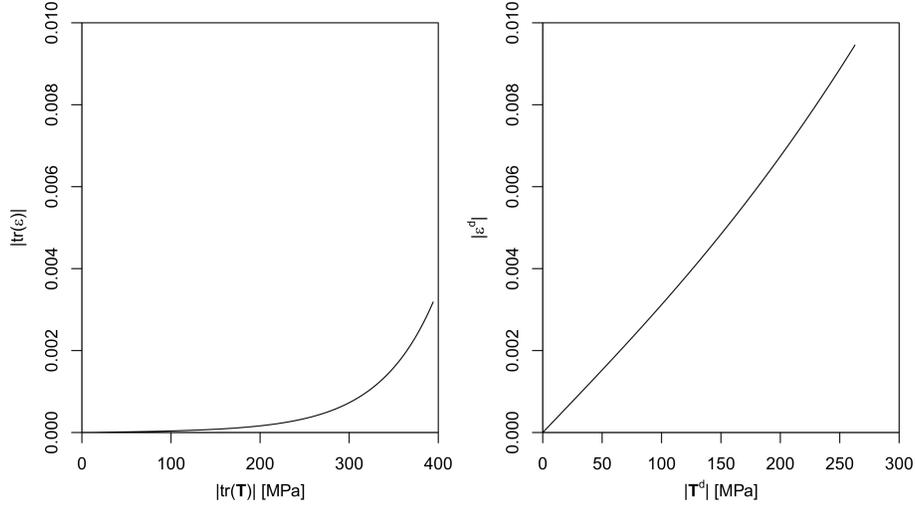
FIG. 8. Bulk and shear response (4.1) of the model (3.1)–(3.2) for *Ti-24Nb-4Zr-7.9Sn* alloy.
