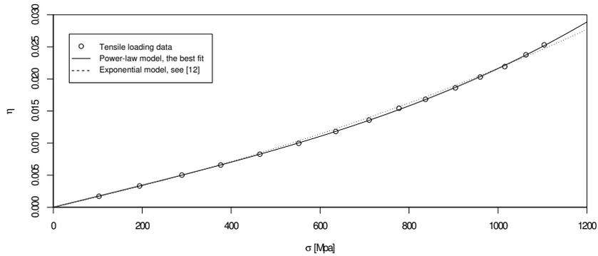
FIG. 2. Plot of the best fit for the model (3.5) compared with the exponential model (2.4) for Gum Metal, see [12].
