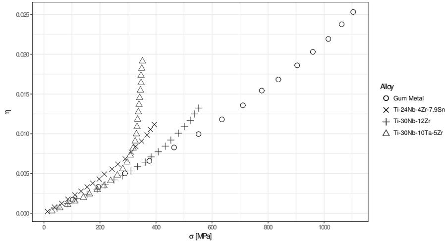
FIG. 1. Stress strain response to tensile loading of considered titanium alloys in the elastic regimen.
