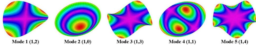
**FIG. 4.** The first five natural modes of simply supported (SS), clamped (C) and free (F) circular plate.
