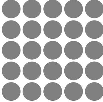
FIG. 1. Section perpendicular to the unidirectional cylinders.
