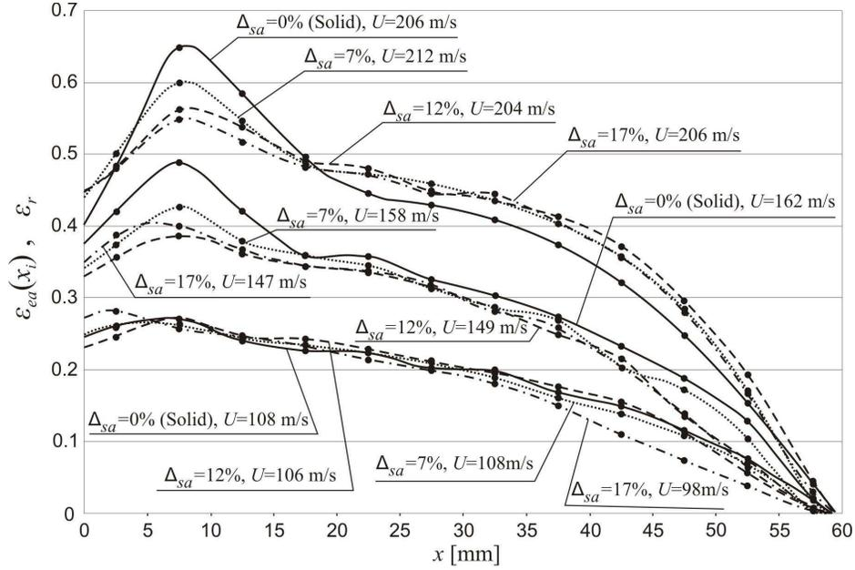
FIG. 2. Interpolation of the discrete values of strain  $\varepsilon_{ea}(x_i)$  along the samples deformed during Taylor DIE, where  $x$  is Lagrangian coordinate.
