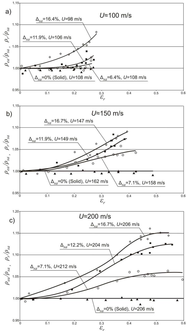
FIG. 5. Relative density – LECS dynamic curves for porous copper.
