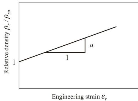
FIG. 6. Relative density versus compressive engineering strain [8].
