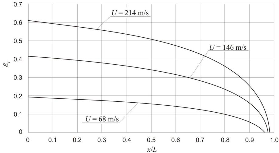
FIG. 3. Theoretical distribution of compressive current strain  $\varepsilon_r$  in the solid copper rod after Taylor impact test, without allowing for the friction force [9].
