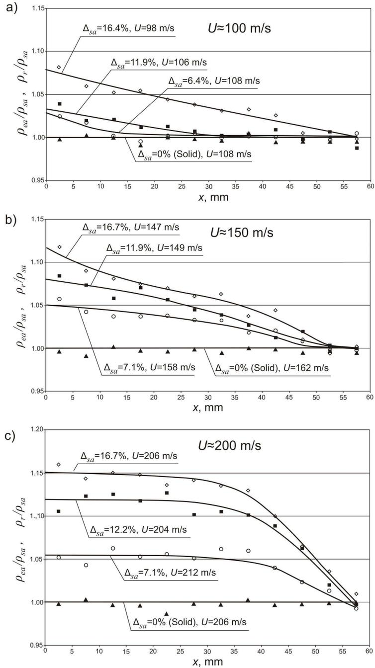
FIG. 4. Approximation of discrete values of ratio  $\rho_{ea}(x_i)/\rho_{sa}$  along deformed samples during Taylor DIE, where  $x$  is Lagrangian coordinate.
