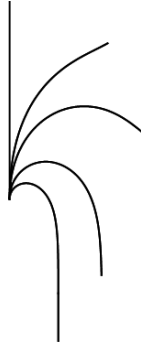
FIG. 3. Effect of tip load on deformation ( m = 4 , c = 0.5 , \gamma = 0 ). From top: p < 1.029 , 1.5, 2, 10, 50.
