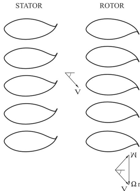
FIG. 1. Velocity triangle in an axial turbine.
