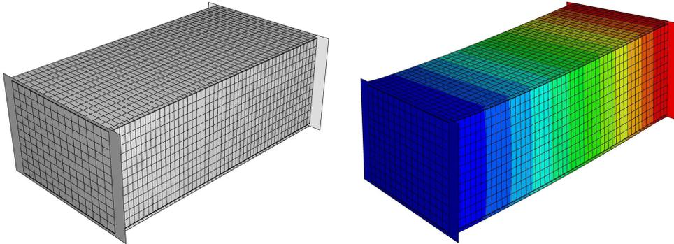
FIG. 3. Numerical model of the beam.
