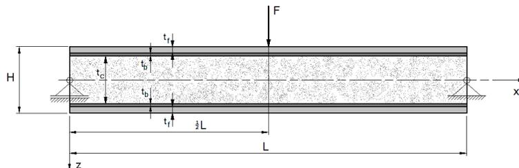
FIG. 1. Scheme of the loaded beam.
