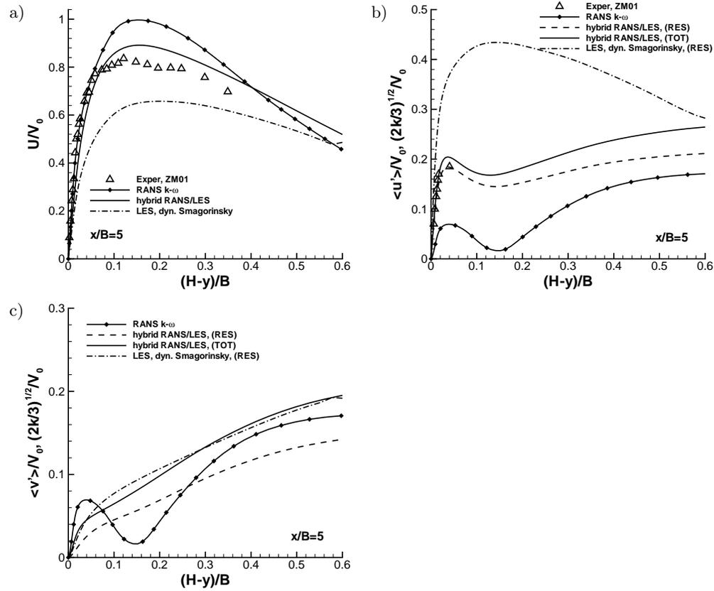
FIG. 7. Profiles of a) mean streamwise velocity, b) streamwise fluctuating and c) wall-normal fluctuating velocity components for plane impinging jet simulation at  $H/B = 2$ ,  $Re = 10000$  at distance  $x/B = 5$  from the symmetry plane.
