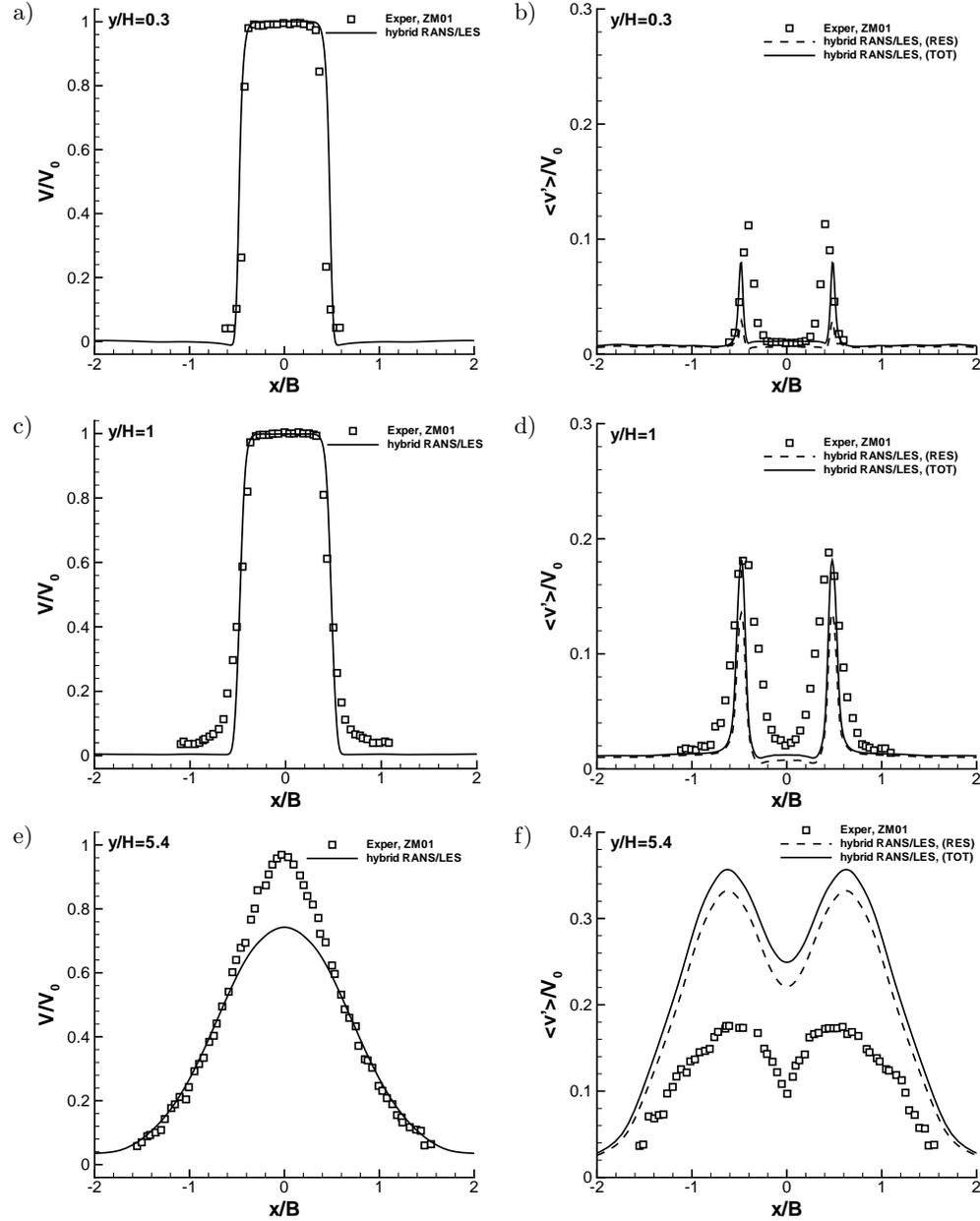
FIG. 3. Profiles of mean  $y$ -velocity (a, c, e) and r.m.s. of fluctuating  $y$ -velocity component (b, d, f) for simulation of the plane impinging jet at  $H/B = 9.2$ ,  $Re = 20000$  at various distances from the jet exit: a, b)  $y/H = 0.3$ , c, d)  $y/H = 1$ , e, f)  $y/H = 5.4$  and comparison with experiment (free jet). The resolved and total (resolved+modelled) velocity fluctuations are denoted by RES and TOT, respectively.
