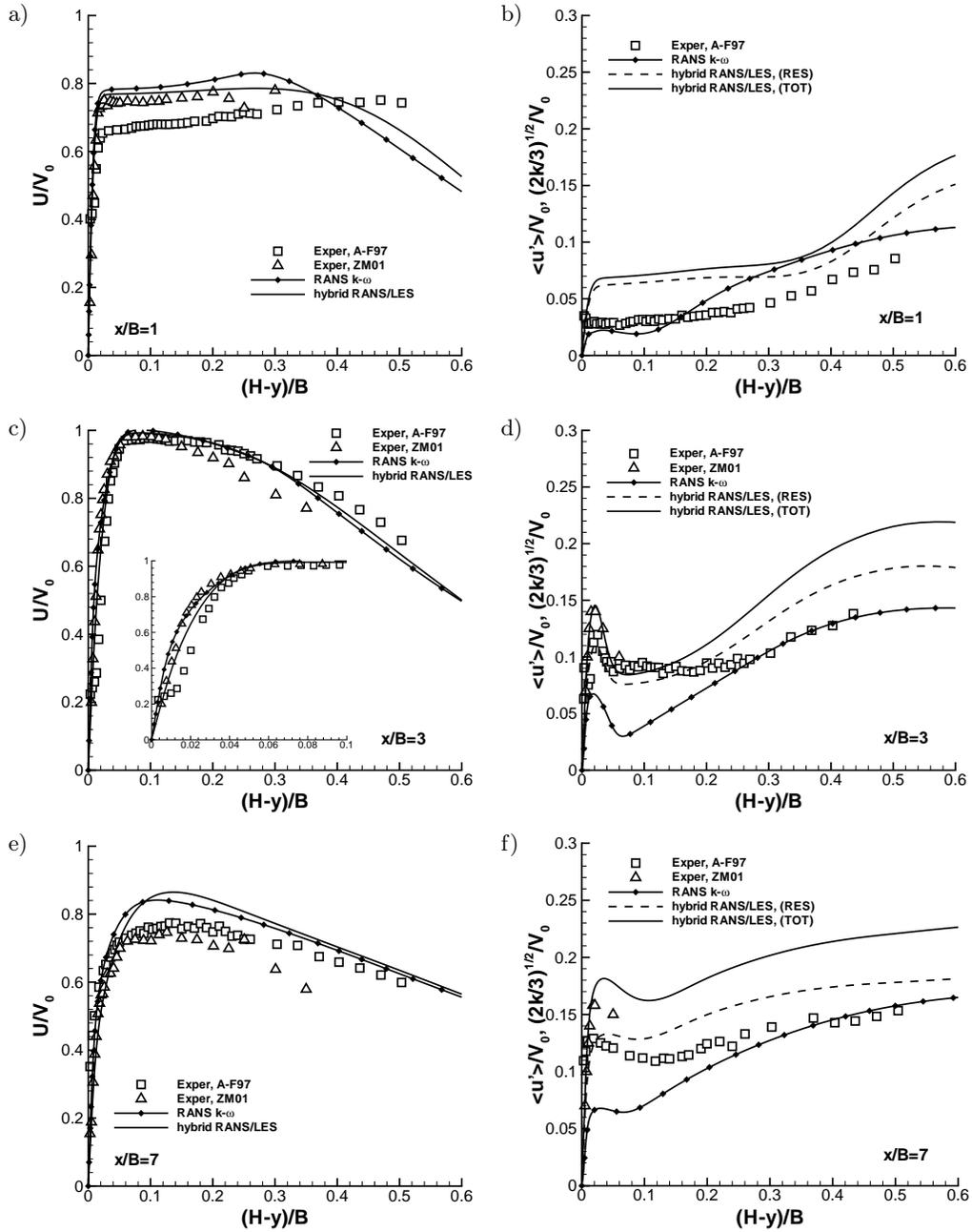
FIG. 13. Profiles of mean streamwise velocity (a, c, e) and r.m.s. of streamwise fluctuating velocity component (b, d, f) for simulation of the plane impinging jet at  $H/D = 4$ ,  $Re = 18000$  at various distances from the symmetry plane: a, b)  $x/B = 1$ ; c, d)  $x/B = 3$  and e, f)  $x/B = 7$ . In case of the hybrid model the resolved and total (resolved+modelled) fluctuations are denoted by RES and TOT, respectively.
