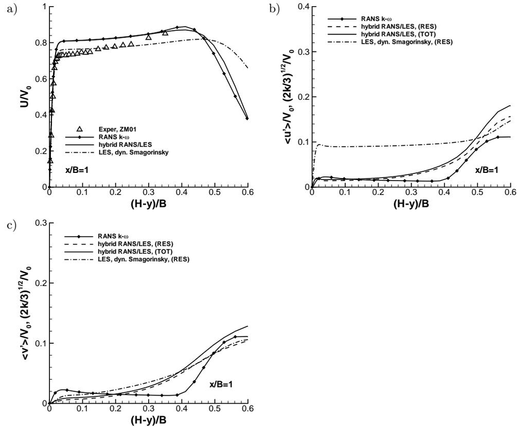
FIG. 5. Profiles of a) mean streamwise velocity, b) streamwise fluctuating and c) wall-normal fluctuating velocity components for plane impinging jet simulation at  $H/D = 2$ ,  $Re = 10000$  at distance  $x/B = 1$  from the symmetry plane.
