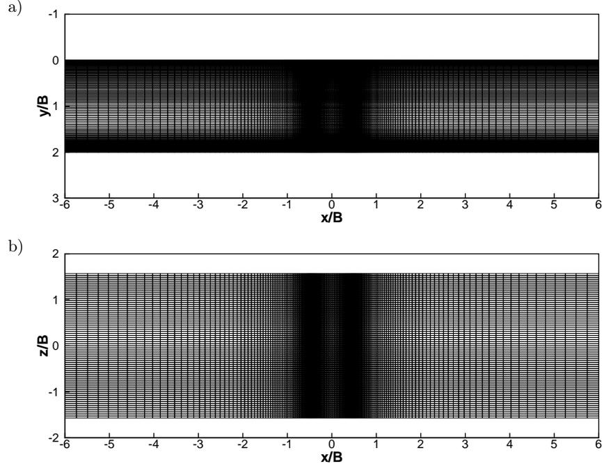
FIG. 2. View of the computational mesh: a) in the  $x$ - $y$  plane and b) in the  $x$ - $z$  plane (impingement plate) for simulation with the hybrid RANS/LES model ( $H/B = 2$ ).
