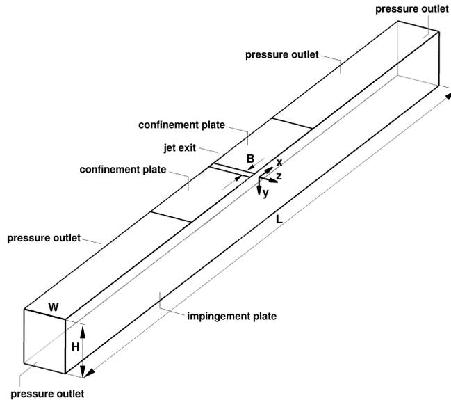
FIG. 1. Sketch of computational domain, coordinate system and boundary conditions for plane impinging jet simulation at  $H/B = 4$ . Periodic conditions are imposed in the  $z$ -direction.
