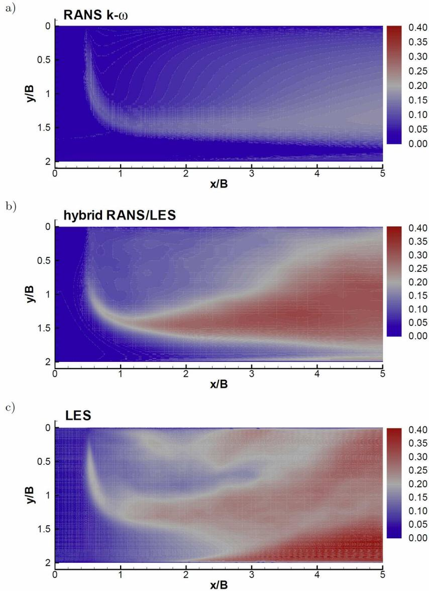
FIG. 9. Contour plots of time-averaged r.m.s. of fluctuating velocity component  $\langle u' \rangle / V_0$  in the  $x$ - $y$  plane obtained with a) the RANS  $k$ - $\omega$ , b) the hybrid RANS/LES (2.5 M cells) and c) the LES (15.1 M cells) models. In case of the hybrid and LES models the resolved fluctuations are shown. In RANS the fluctuating velocity means  $(2k/3)^{1/2} / V_0$ .
