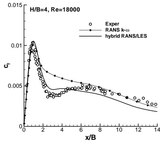
FIG. 14. Skin friction coefficient for  $H/B = 4$ ,  $Re = 18000$ .
