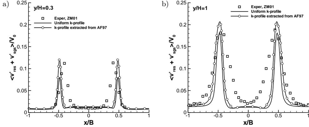
FIG. 4. Profiles of fluctuating  $y$ -velocity component at distance a)  $y/H = 0.3$  and b)  $y/H = 1$  from the jet exit for simulation of the plane impinging jet at  $H/B = 9.2$ ,  $\text{Re} = 20\,000$  with uniform and variable inlet profile of turbulent kinetic energy.
