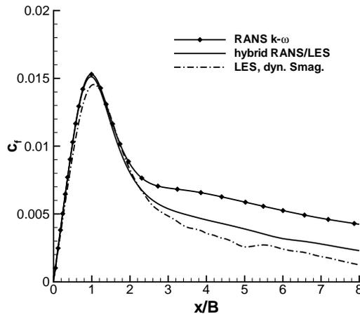
FIG. 10. Skin friction coefficient for  $H/B = 2$ ,  $Re = 10\,000$ .
