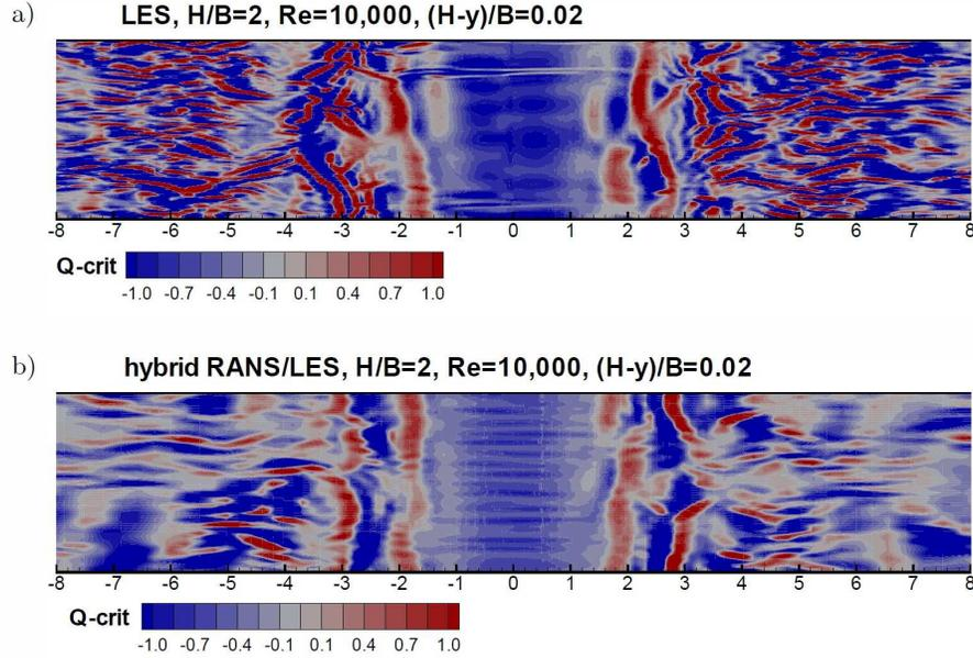
FIG. 11. Contour plots of Q-criterion in the  $x$ - $z$  plane at distance  $(H - y)/B = 0.02$  from the impingement plate obtained with a) LES (15.1M cells) and b) hybrid RANS/LES model (2.5M cells).
