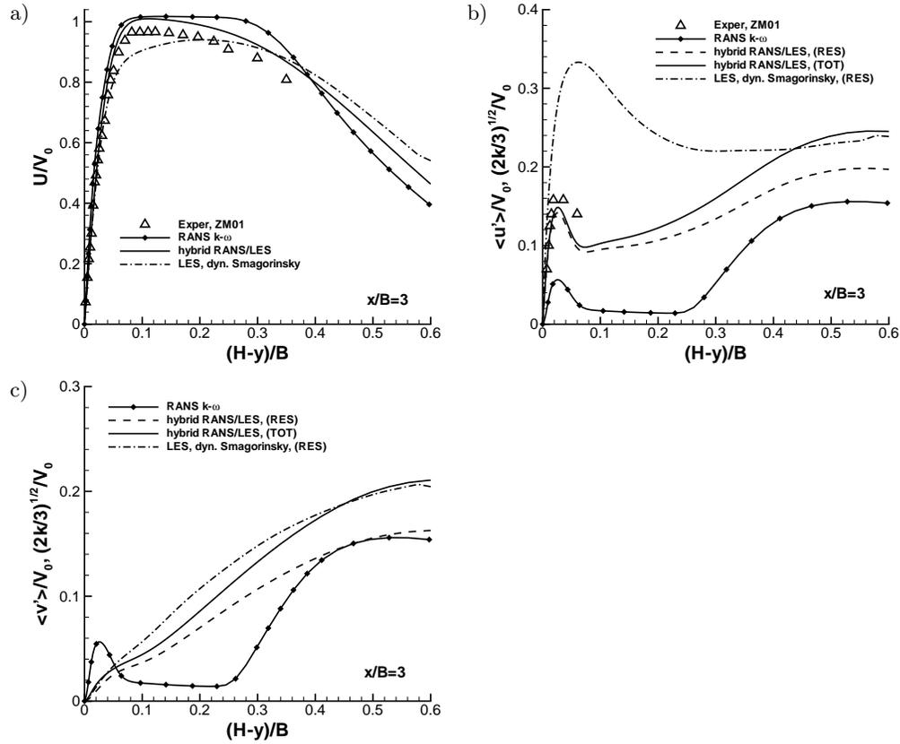
FIG. 6. Profiles of a) mean streamwise velocity, b) streamwise fluctuating and c) wall-normal fluctuating velocity components for plane impinging jet simulation at  $H/B = 2$ ,  $Re = 10000$  at distance  $x/B = 3$  from the symmetry plane.
