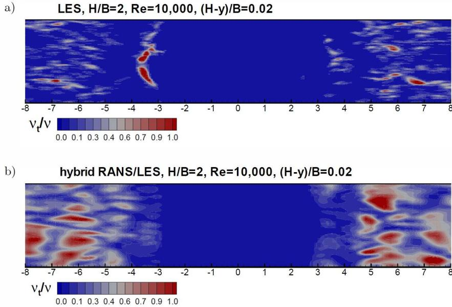
FIG. 12. Contour plots of ratio of modelled to molecular viscosity in the  $x$ - $z$  plane at distance  $(H - y)/B = 0.02$  from the impingement plate obtained with a) LES (15.1M cells) and b) hybrid RANS/LES model (2.5M cells).
