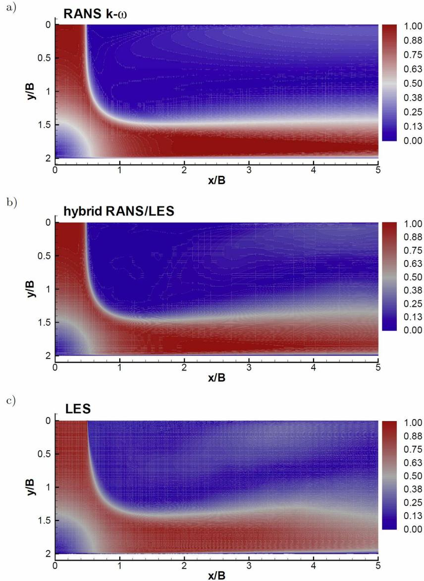
FIG. 8. Contour plots of time-averaged velocity magnitude  $|U|/V_0$  in the  $x$ - $y$  plane for  $H/B = 2$ ,  $Re = 10000$  with a) the RANS  $k-\omega$ , b) the hybrid RANS/LES (2.5 M cells) and c) the LES (15.1 M cells) models.
