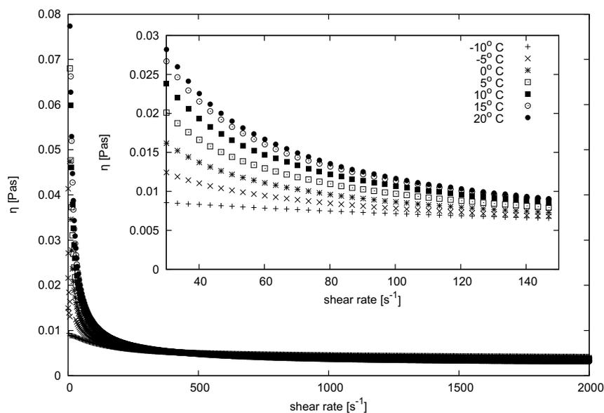
FIG. 5. Dependence of dynamic viscosity of 10 wt.% concentration of  $\text{MgAl}_2\text{O}_4$  in ethyl alcohol for various temperatures.
