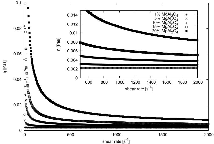
FIG. 6. Dependence of dynamic viscosity of  $\text{MgAl}_2\text{O}_4$  in ethyl alcohol on concentration at  $0^\circ\text{C}$ .
