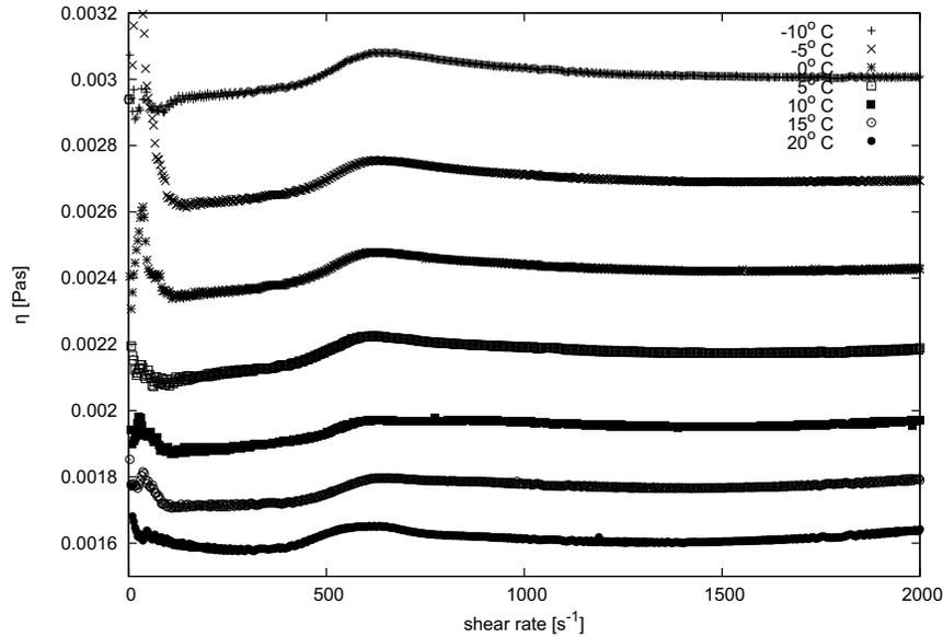
FIG. 2. Results of dynamic viscosity measurements of suspension of 10 wt.%  $Y_2O_3$  in ethylen in various temperature.
