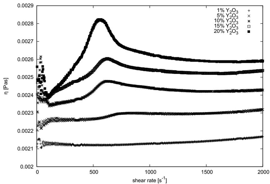
FIG. 4. Dependence of dynamic viscosity of the shear rate for various concentrations  $Y_2O_3$  in ethyl alcohol at 0°C.
