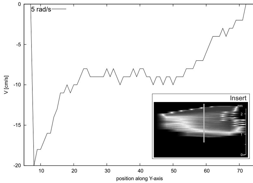
FIG. 3. Distribution of velocity in 10 wt.%  $Y_2O_3$  in ethyl alcohol at rotor speed of 5.0 rad/s. Insert presents velocity map inside examined sample.
