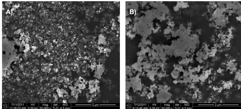
FIG. 1. Images of ceramic nanopowders taken with the SEM microscope: A) magnesium-aluminum spinel ( $MgAl_2O_4$ ), B) yttrium oxide ( $Y_2O_3$ ).
