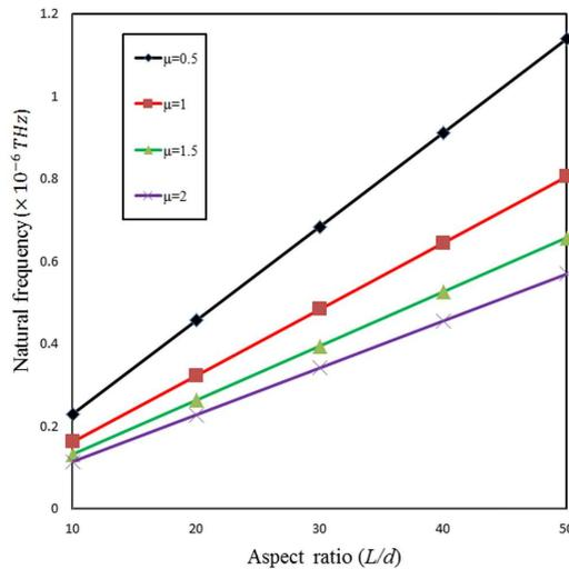
FIG. 4. Variation of natural frequency with aspect ratio  $L/d$  for different nonlocal parameters ( $K_W = 10^3 \text{ N/m}^2, m = 1$ ).
