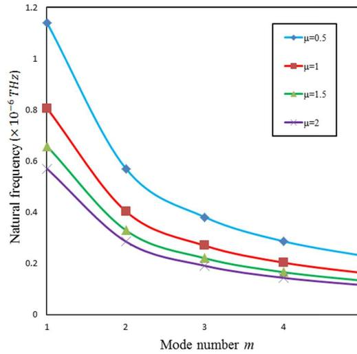
FIG. 5. Effect of mode number on natural frequency for different nonlocal parameters  $\mu$  ( $K_W = 10^3$  N/m<sup>2</sup>  $L/d = 50$ ).
