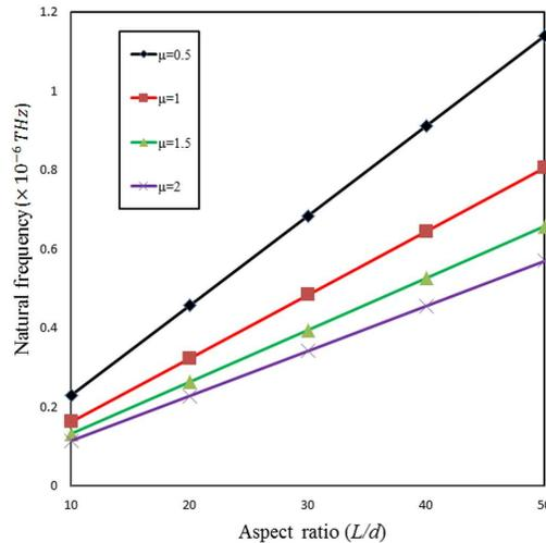
FIG. 2. Change of natural frequency with aspect ratio  $L/d$  for different change in nonlocal parameter.
