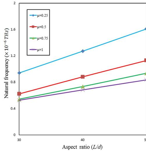
FIG. 9. Effect of nonlocal parameter  $\mu$  on natural frequency with different aspect ratios  $L/d$  ( $K_w = K_G = 0$ ,  $m = 1$ ,  $\theta = 50^\circ$  K).
