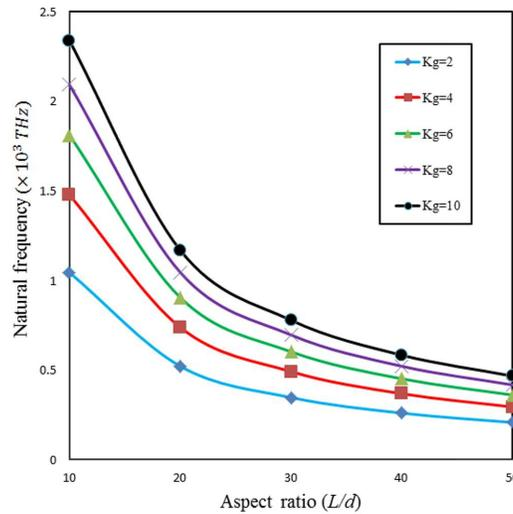
FIG. 12. Effect of aspect ratio  $L/d$  and Pasternak's foundation  $K_G$  on frequency of a SWCNT ( $K_W = 10^2 \text{ N/m}^2$ ,  $\theta = 50^\circ \text{ K}$ ,  $m = 1$ ,  $\mu = 0$ ).
