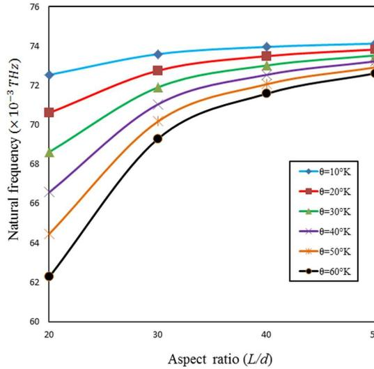
FIG. 11. Variation of natural frequency with temperature for different aspect ratio  $L/d$  and high Winkler's modulus  $K_W$  ( $\mu = 1$ ,  $K_G = 0$ ,  $m = 1$ ,  $K_W = 10^7$  N/m<sup>2</sup>).
