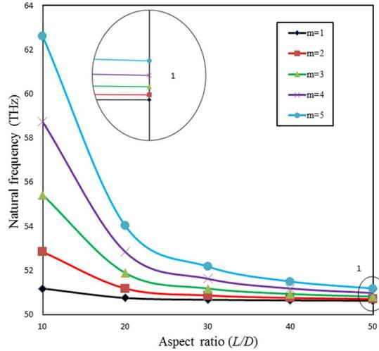
FIG. 1. Variation of natural frequency with aspect ratio  $L/d$  for different change in mode number  $m$  for SWCNT ( $K_W = K_G = \bar{N} = 0$ ).
