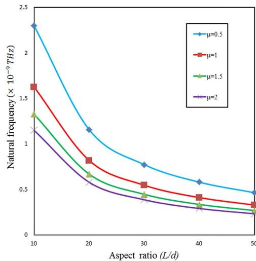
FIG. 13. The omission of rotary inertia  $m_2$  and its effect on natural frequency for different nonlocal parameters.
