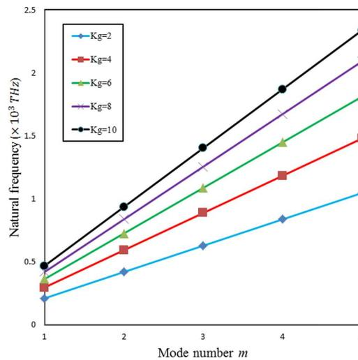
FIG. 7. The natural frequency of a SWCNT with different mode number  $m$  and shear modulus  $K_G$  ( $K_W = 10^2$  N/m<sup>2</sup>,  $\mu = 0.5$ ,  $L/d = 50$ ).
