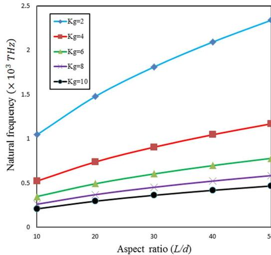
FIG. 6. The effect of shear modulus parameter  $K_G$  on natural frequency of a SWCNT for different aspect ratios  $L/d$  ( $K_W = 10^2$  N/m<sup>2</sup>,  $m = 1$ ,  $\mu = 0.5$ ).
