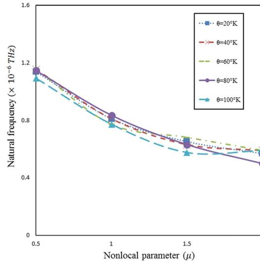
FIG. 8. Effect of temperature on frequency of a SWCNT with different nonlocal parameter  $\mu$  ( $L/d = 50$ ,  $K_G = K_W = 0$ ,  $m = 1$ ).
