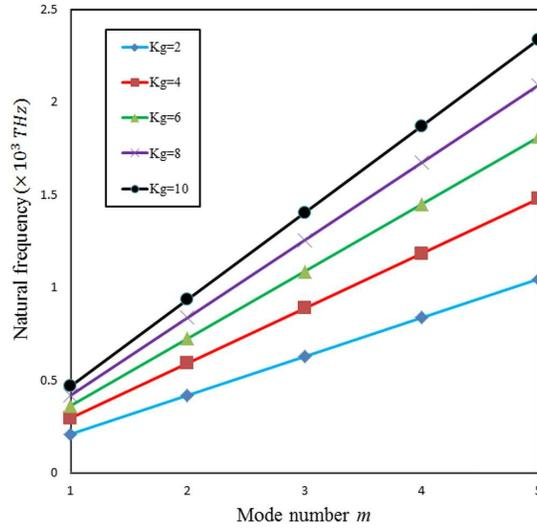
FIG. 10. Effect of mode numbers on natural frequency for different shear modulus parameter  $K_G$  ( $\mu = 0.5$ ,  $L/d = 50$ ,  $K_W = 10^2$  N/m<sup>2</sup>,  $\theta = 50^\circ$  K).
