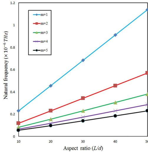
FIG. 3. Mode number effect on natural frequency of a SWCNT for different aspect ratio  $L/d$  and  $\mu = 0.5$ .
