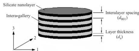
FIG. 6. Schematic continuum representation for the hierarchical structure of intercalated nanoclay.
