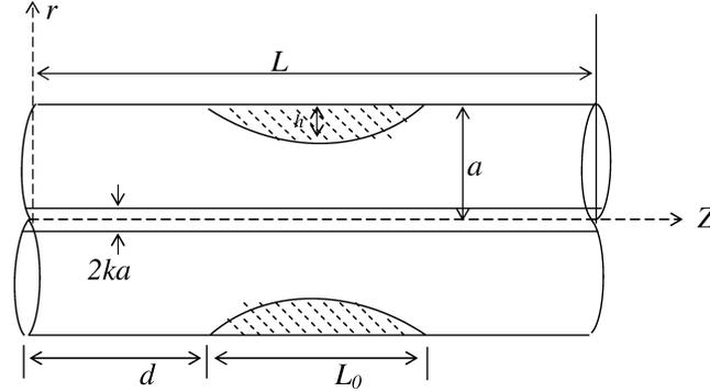
FIG. 1. Schematic diagram of catheterized stenosed artery.
