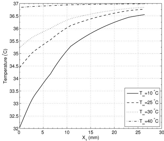
FIG. 9. Temperature variation on the papillary axis for different ambient convection coefficients ( $h_{\infty} = 10 \text{ Wm}^{-2}\text{K}^{-1}$ ).
