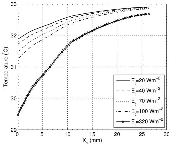
FIG. 7. Temperature variation on the papillary axis for different evaporation rates.
