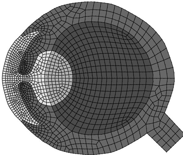
FIG. 3. Hybrid finite elements for human eye model.
