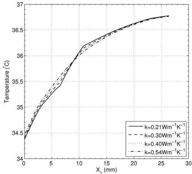
FIG. 10. Temperature variation on the papillary axis for different lens thermal conductivity.
