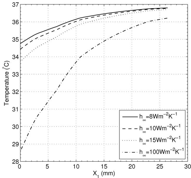
**FIG. 8.** Temperature variation on the papillary axis for different ambient convection coefficients ( $T_{\infty} = 25^{\circ}\text{C}$ ).
