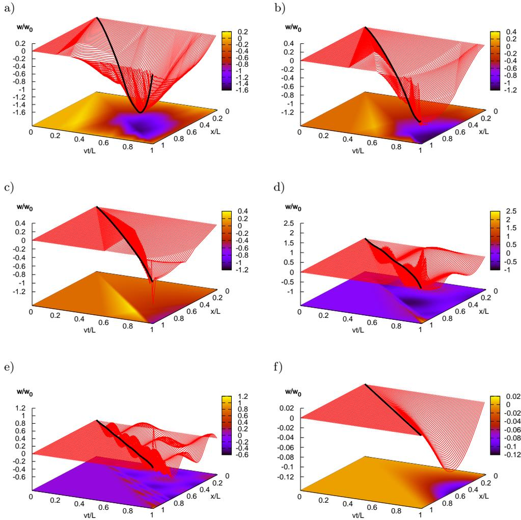
FIG. 7. Simulation of the Timoshenko beam under the moving inertial point at the speed: a)  $v = 0.2$ , b)  $v = 0.4$ , c)  $v = 0.6$ , d)  $v = 0.7$ , e)  $v = 0.9$  and f)  $v = 1.0$  ( $c_1 = 0.63$ ,  $c_2 = 1.00$ ).
