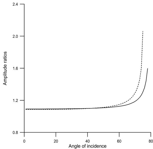
FIG. 6. Variations of amplitude ratios of refracted thermal waves with the angle of incidence in presence (solid curve) and in absence (dotted curve) of initial stresses.
