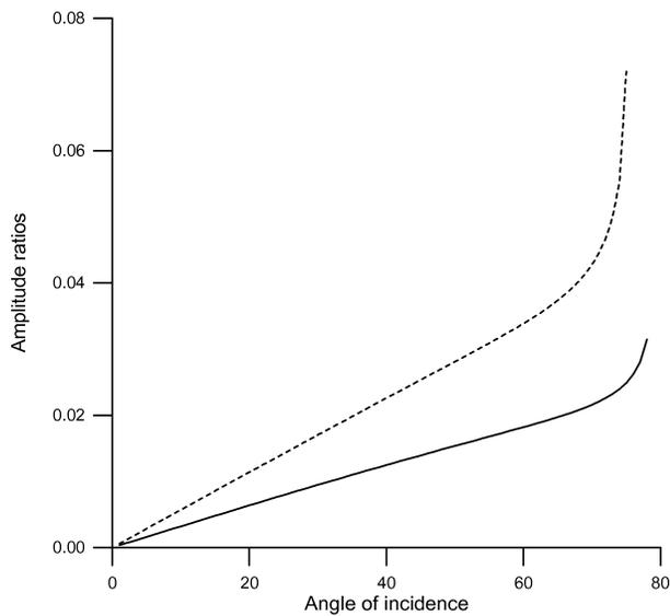
FIG. 7. Variations of amplitude ratios of refracted SV waves with the angle of incidence in presence (solid curve) and in absence (dotted curve) of initial stresses.
