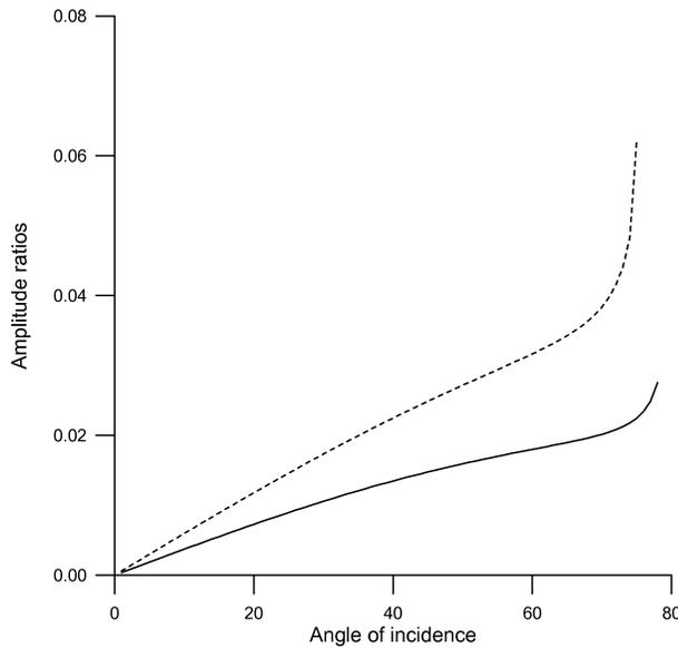
FIG. 4. Variations of amplitude ratios of reflected SV waves with the angle of incidence in presence (solid curve) and in absence (dotted curve) of initial stresses.
