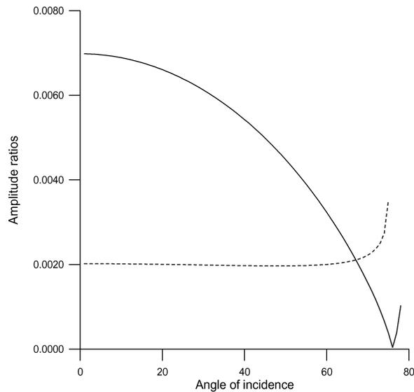
FIG. 2. Variations of amplitude ratios of reflected P waves with the angle of incidence in presence (solid curve) and in absence (dotted curve) of initial stresses.
