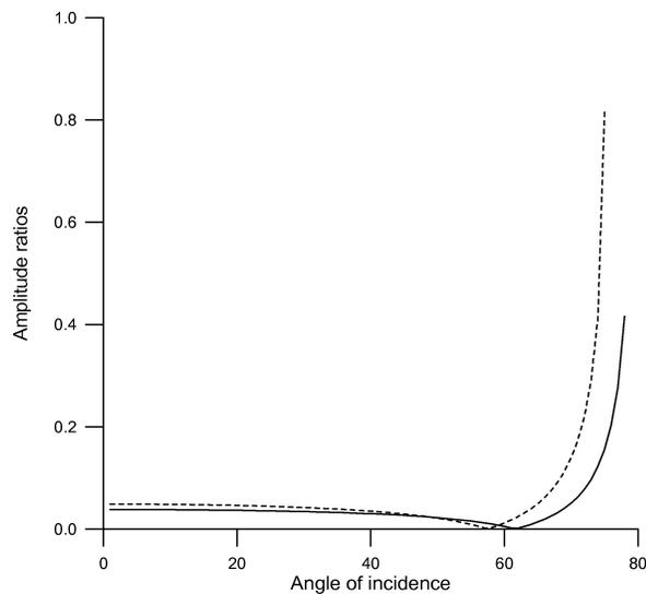
FIG. 3. Variations of amplitude ratios of reflected thermal waves with the angle of incidence in presence (solid curve) and in absence (dotted curve) of initial stresses.
