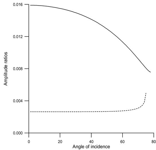
FIG. 5. Variations of amplitude ratios of refracted P waves with the angle of incidence in presence (solid curve) and in absence (dotted curve) of initial stresses.
