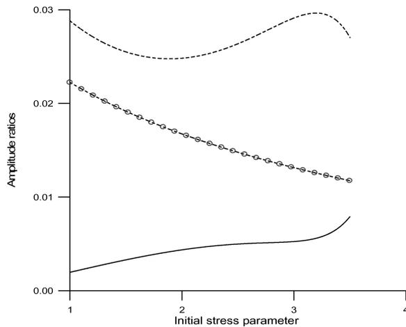
FIG. 8. Variations of amplitude ratios of reflected P wave (solid curve), reflected thermal (dotted curve) and reflected SV wave (dotted curve with circles) with the initial stress parameter  $\eta$ .
