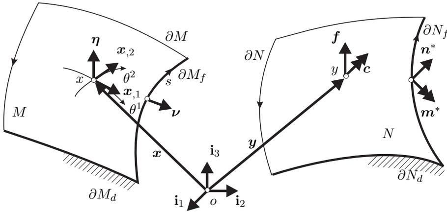
FIG. 1. Shell kinematics.
