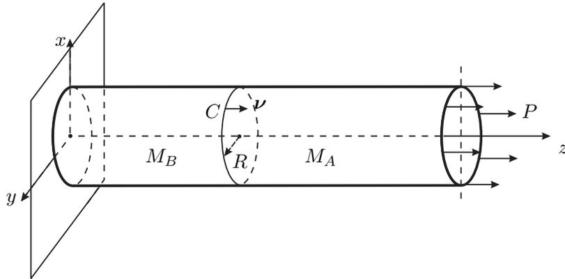
FIG. 3. Tension of the two-phase thin-walled tube.
