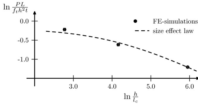
FIG. 14. Relationship between calculated normalized concrete strength  $\ln \sigma = \ln[PL/(f_t h^2 t)]$  and ratio  $\ln(h/l_c)$  compared to the size effect law by Bažant (BAŽANT and PLANAS [4]) for constant values of tensile strength.
