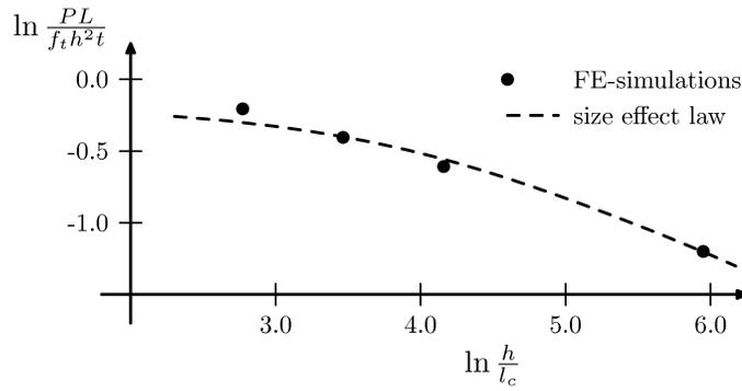
FIG. 10. Relationship between the calculated normalized concrete strength  $\ln \sigma = \ln[PL/(f_t h^2 t)]$  and ratio  $\ln(h/l_c)$ , compared to the size effect law by Bažant (BAŽANT and PLANAS [4]) for constant values of tensile strength.
