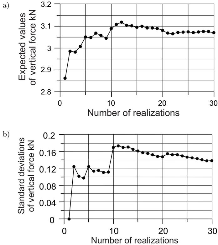
FIG. 16. Small size beam with random distribution of tensile strength ( $h = 8$  cm) using a direct Monte Carlo method with 30 samples: maximum vertical force with expected values (a) and standard deviation (b) ( $\lambda_{x_1} = 1.0$  1/m,  $\lambda_{x_2} = 3.0$  1/m,  $s_{f_t} = 0.424$  MPa)
