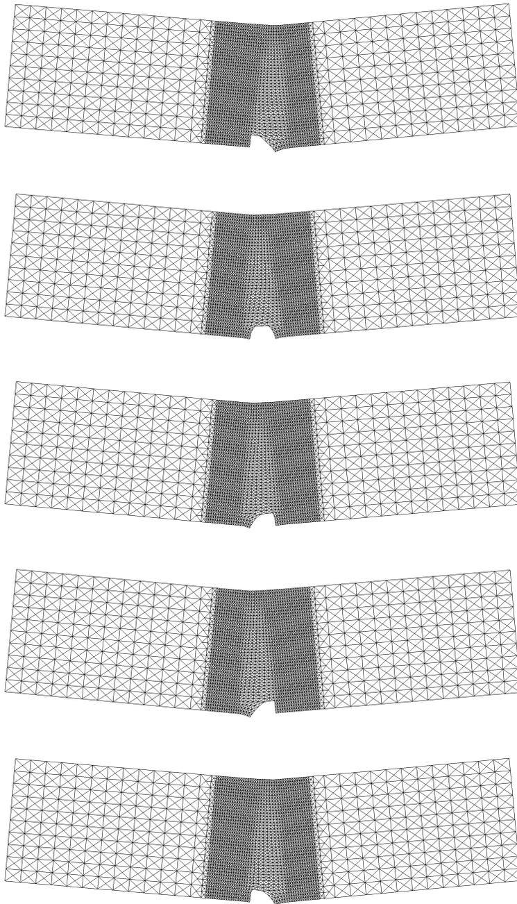
FIG. 15. Five arbitrary deformed FE meshes for a small size beam ( $h = 8$  cm)  $u/h = 0.25\%$  with random distribution of tensile strength ( $\lambda_{x_1} = 1.0$  1/m,  $\lambda_{x_2} = 3.0$  1/m.  $s_{ft} = 0.424$  MPa).
