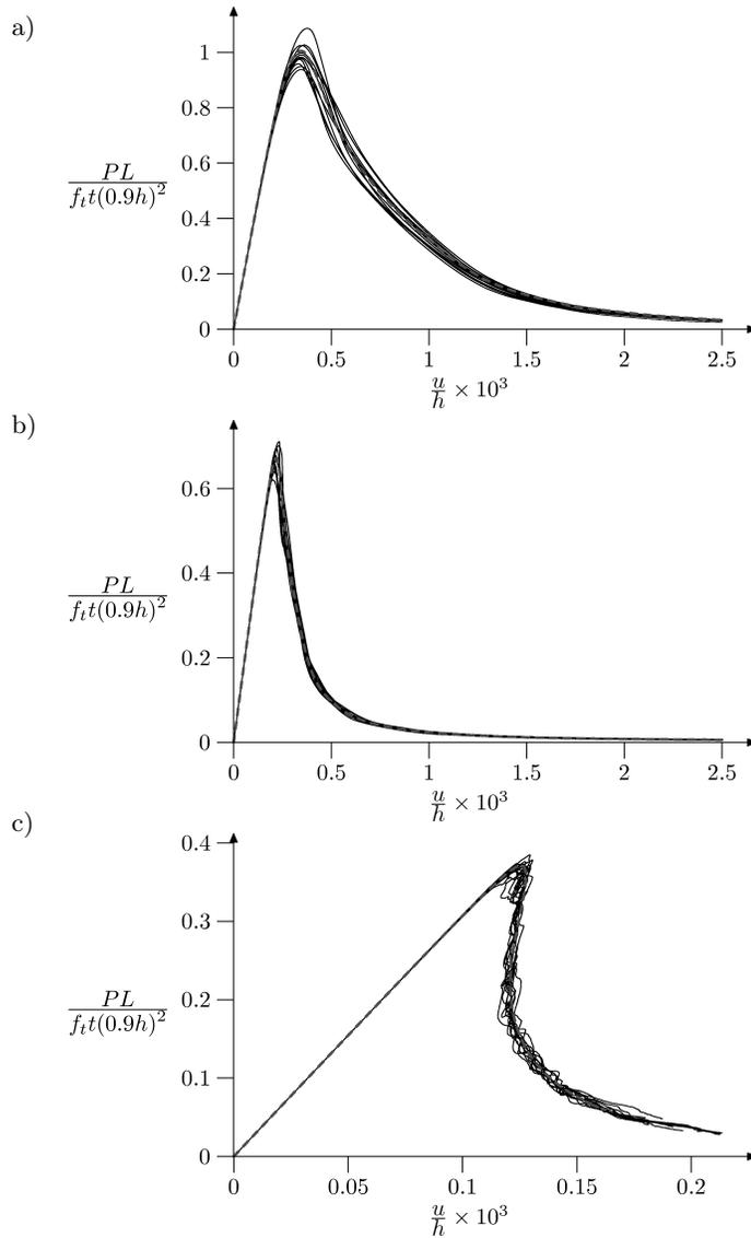
FIG. 12. Normalized force-displacement curves in the case of deterministic (dashed lines) and random calculation (solid lines) for 3 notched beams under three-point bending: a) small size beam ( $h = 8$  cm), b) large size beam ( $h = 32$  cm), c) very large size beam ( $h = 192$  cm) ( $\lambda_{x_1} = 1.0$  1/m,  $\lambda_{x_2} = 3.0$  1/m,  $s_{f_t} = 0.424$  MPa).
