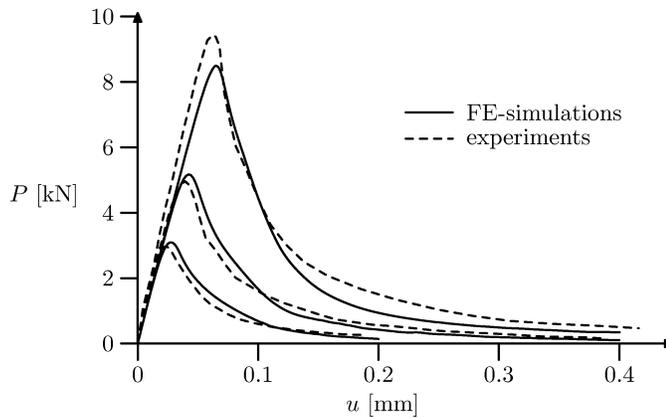
FIG. 11. The load-displacement curves from FE-calculations with constant values of tensile strength compared to the experiments by LE BELLEGO *et al.* [30]:  $h = 8$  cm,  $h = 16$  cm and  $h = 32$  cm.
