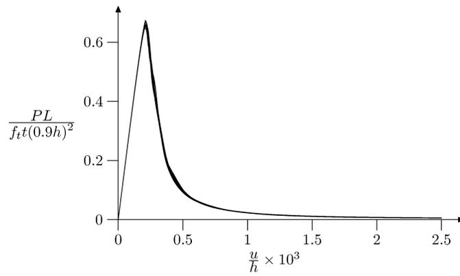
FIG. 17. Normalized force-displacement curves with and random distribution of tensile strength for notched small beam under three-point bending ( $h = 8$  cm) for smaller correlation length ( $\lambda_{x_1} = 10.0$  1/m,  $\lambda_{x_2} = 10.0$  1/m,  $s_{f_t} = 0.424$  MPa)
