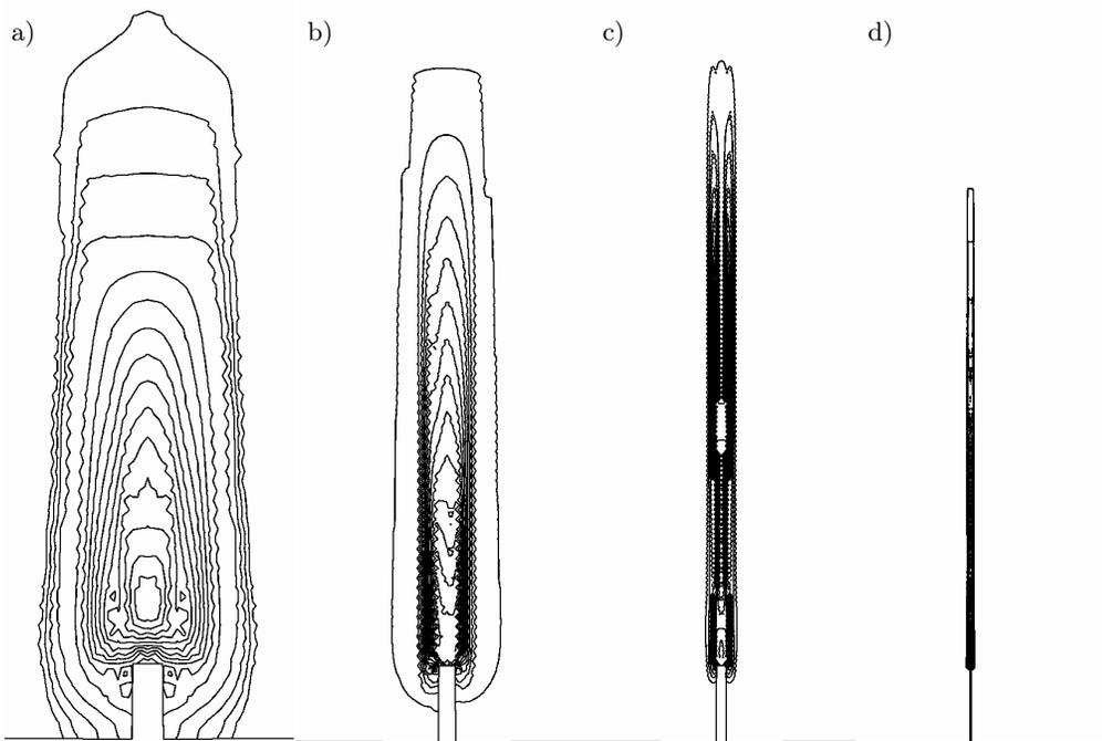
FIG. 9. Calculated contours of non-local softening parameter  $\bar{k}$  above the notch for three-point bending of small (a), medium (b), large (c), and very large (d) concrete beam (constant values of tensile strength).
