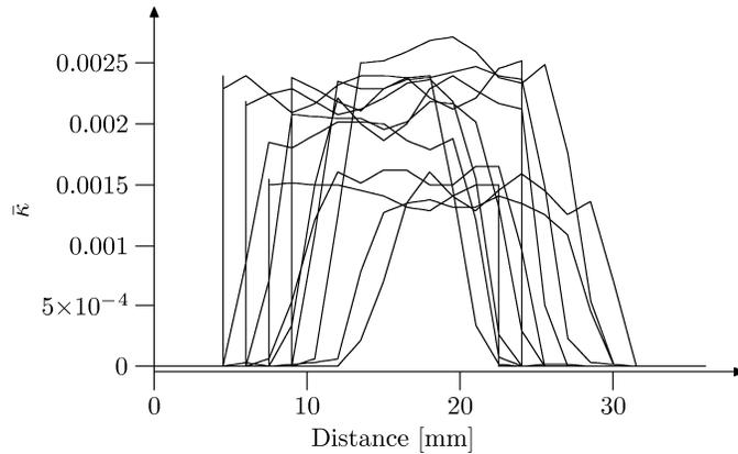
FIG. 18. Distribution of non-local softening parameter random distribution of tensile strength for notched small beam under three-point bending ( $h = 8$  cm) for small correlation length ( $\lambda_{x_1} = 10.0$  1/m,  $\lambda_{x_2} = 10.0$  1/m,  $s_{f_t} = 0.424$  MPa)
