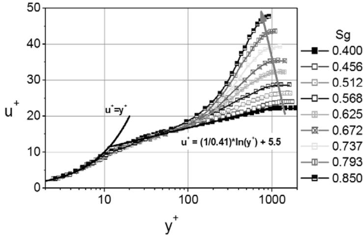
FIG. 6. Mean velocity profiles in TBL under APG conditions in universal coordinates.
