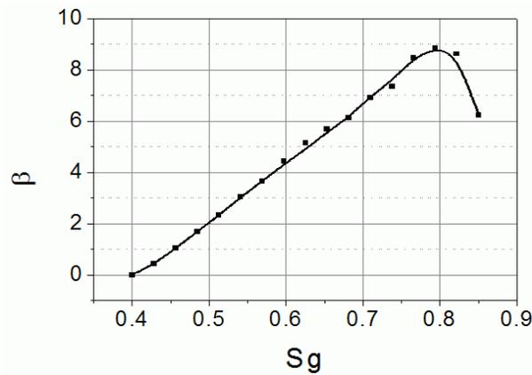
FIG. 8. Distribution of Clauser pressure parameter  $\beta$  calculated acc. to Eq. (2.4) along the measuring region of TBL.
