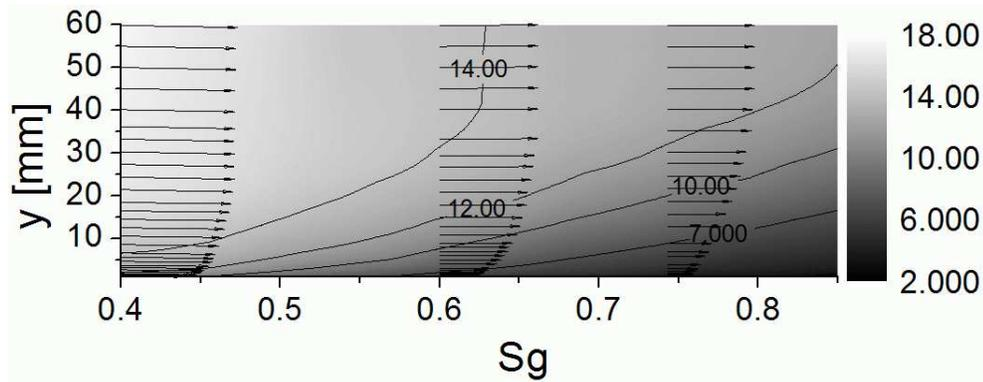
FIG. 4. Evolution of mean velocity field along the flat plate at APG region.
