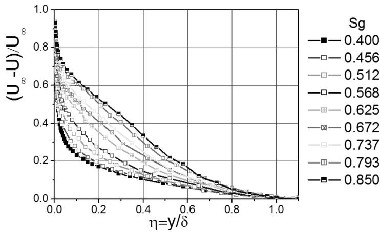
FIG. 9. Mean velocity profile in TBL under APG conditions in George-Castillo (outer) scaling acc. to Eq. (2.6).
