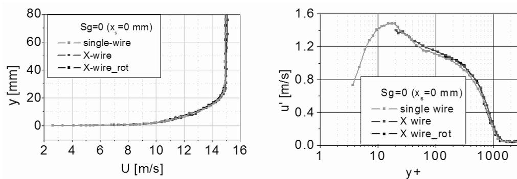
FIG. 3. The comparison of mean velocity (a) and rms of velocity fluctuations (b), measured with single and XC-wire probes at the inlet plane  $S_g = 0.62$ .
