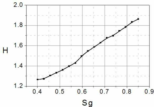
FIG. 5. Downstream evolution of shape parameter at APG region.
