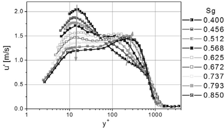
FIG. 14. Evolution of longitudinal velocity fluctuations along the flat plate at APG region.
