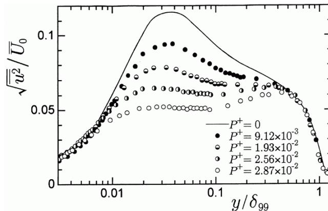
FIG. 15. Evolution of longitudinal velocity fluctuations at APG region obtained in [18]; solid line for ZPG.
