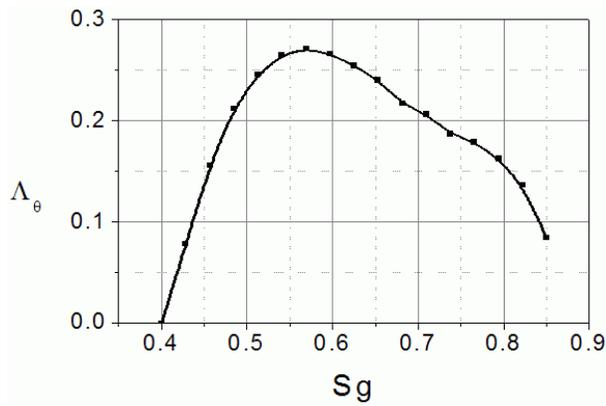
FIG. 11. Distribution of pressure parameter  $\Lambda_\theta$  calculated acc. to Eq. (2.11) along the measuring region of TBL.
