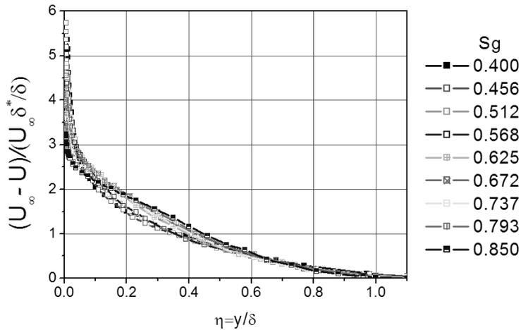
FIG. 12. Mean velocity profile in outer TBL region at APG conditions in Zagarola-Smits (outer) scaling acc. to Eq. (2.12).
