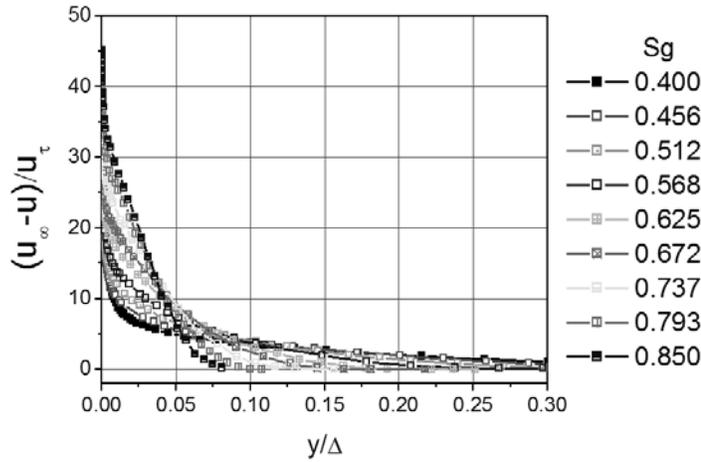
FIG. 7. Mean velocity profile in TBL under APG conditions in von Kármán scaling acc. to Eq. (2.3).
