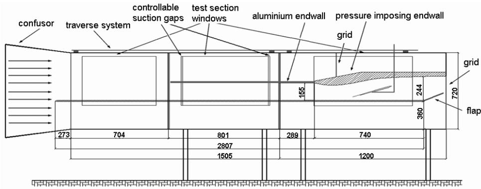
FIG. 1. Schematic view of the wind tunnel and measuring test section.
