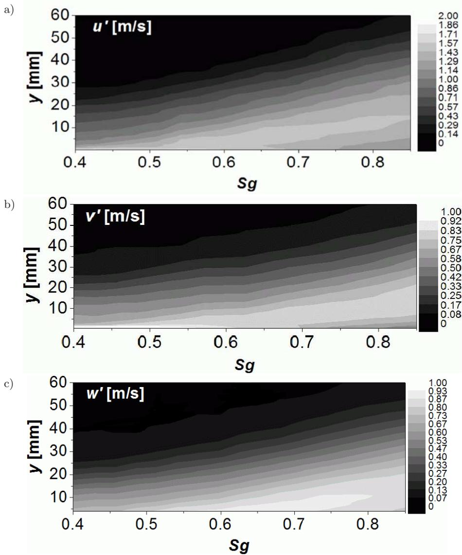
FIG. 13. Evolution of longitudinal (a), transversal (b) and normal (c) velocity fluctuations along the flat plate in APG region.
