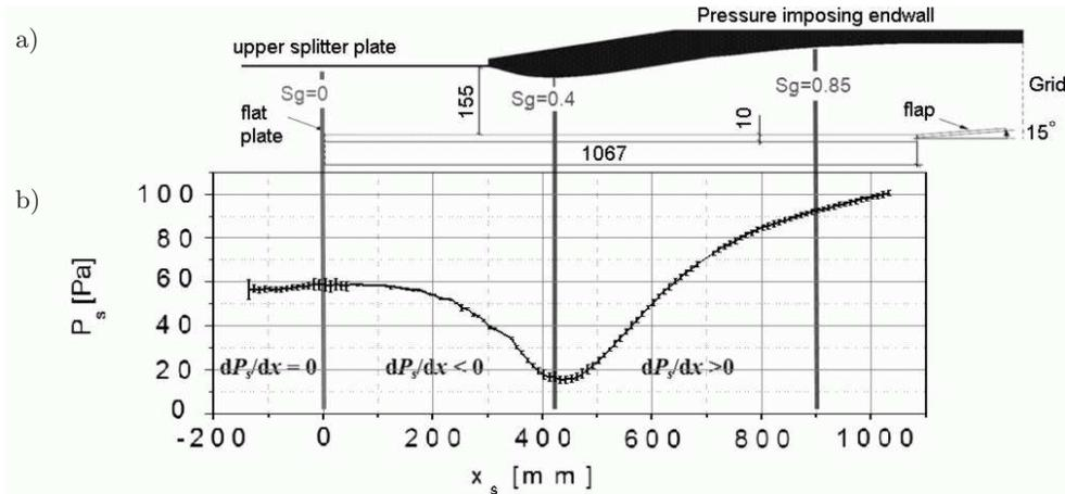
FIG. 2. The shape of upper wall (a) and the corresponding static pressure distribution (b) along the flat plate.
