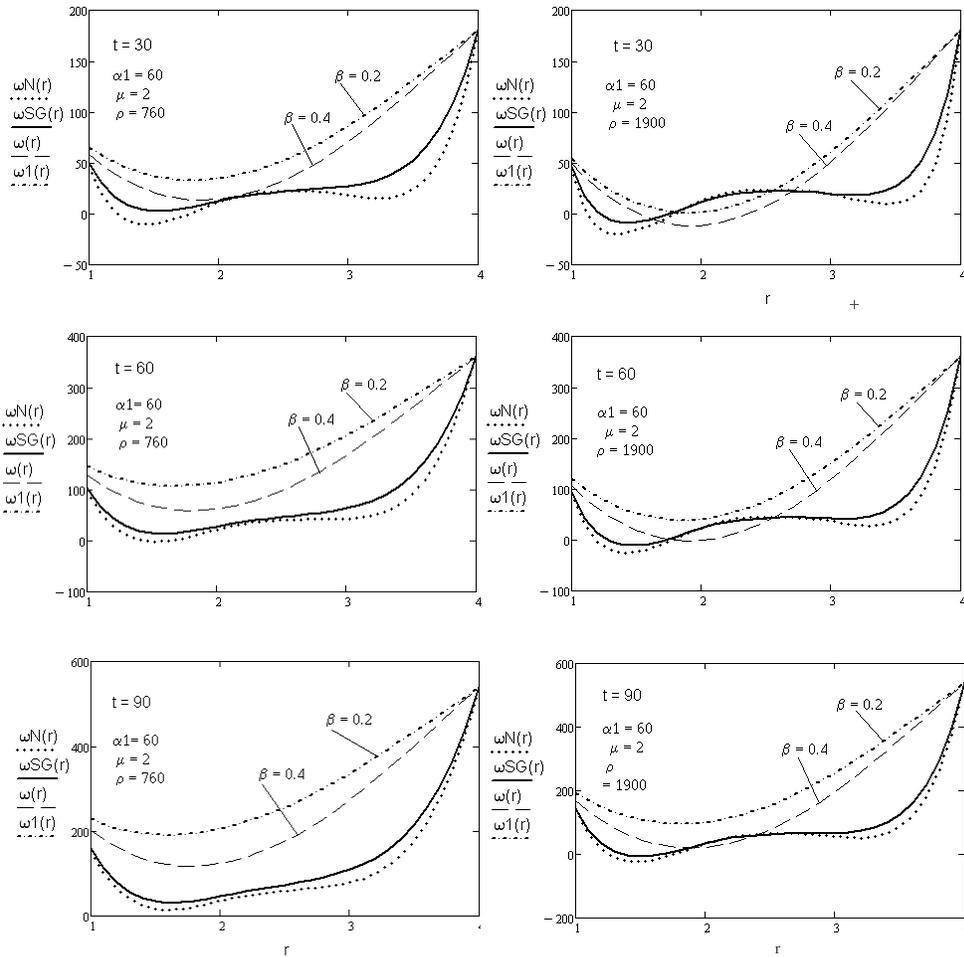
FIG. 6. Velocity profiles for different values of coefficients  $\rho$  and  $\beta$ .
