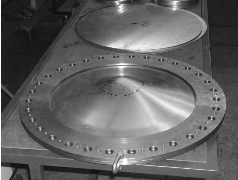
FIG. 3. Inelastic form of a snapped-through aluminium plate
