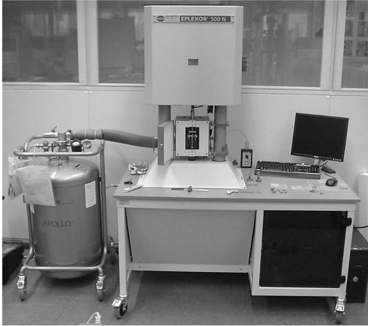
FIG. 1. Dynamic mechanical analysis system, Eplexor 500, GABO.
