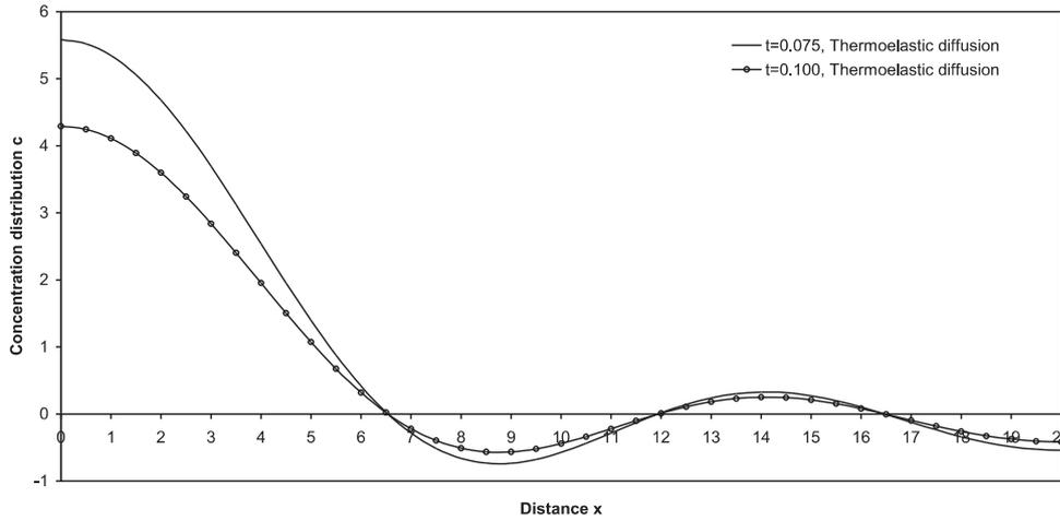
FIG. 4. Distribution of concentration  $c$  (due to normal load) versus distance.
