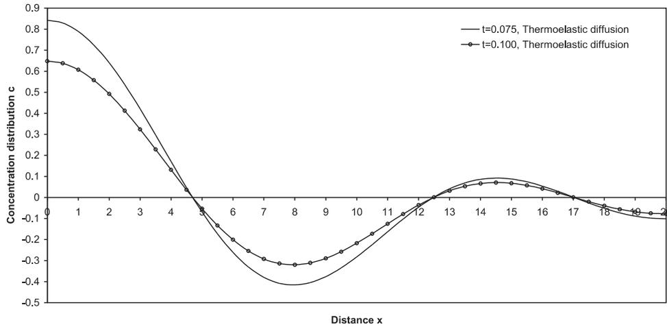
FIG. 8. Distribution of concentration  $c$  (due to tangential load) versus distance.
