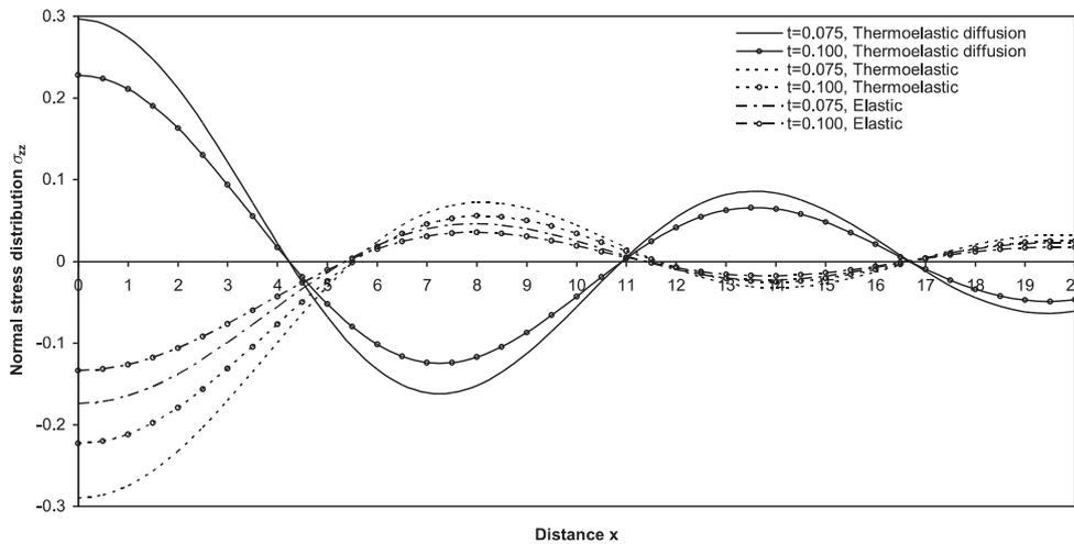
FIG. 2. Distribution of normal stress  $\sigma_{zz}$  (due to normal load) versus distance.
