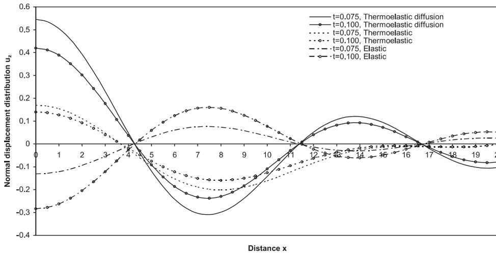
FIG. 5. Distribution of normal displacement  $u_z$  (due to tangential load) versus distance.
