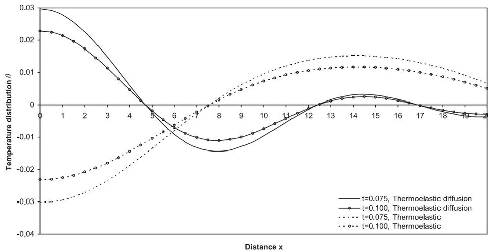
FIG. 7. Distribution of temperature  $\theta$  (due to tangential load) versus distance.
