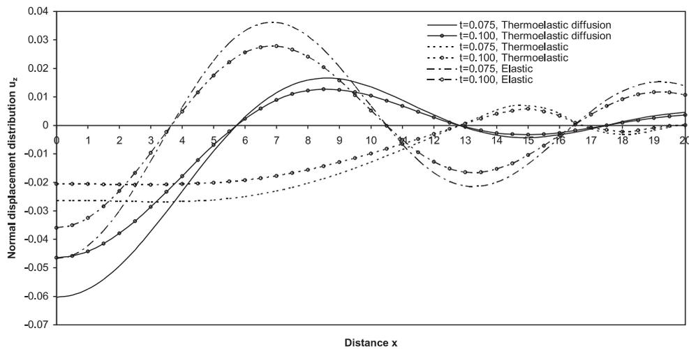
FIG. 1. Distribution of normal displacement  $u_z$  (due to normal load) versus distance.
