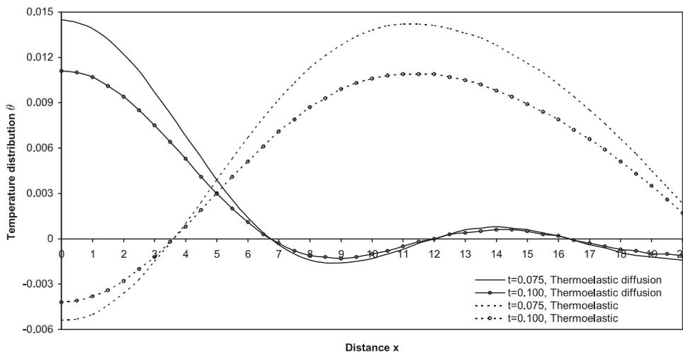
FIG. 3. Distribution of temperature  $\theta$  (due to normal load) versus distance.
