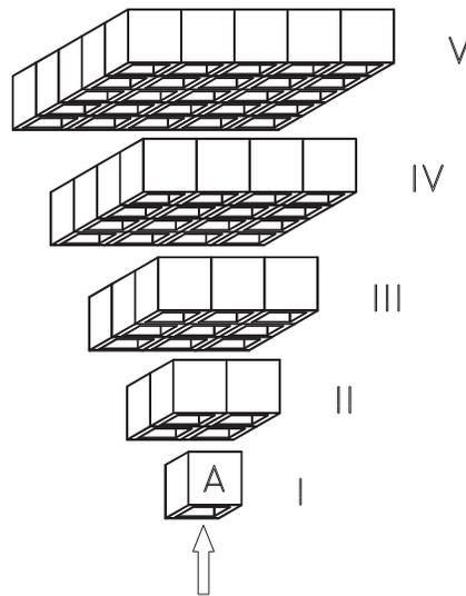
FIG. 16. Assumed system of finite cells for the analysis of migration of a single cavity  $A$  towards the upper surface of the bulk cf. Fig. 15.
