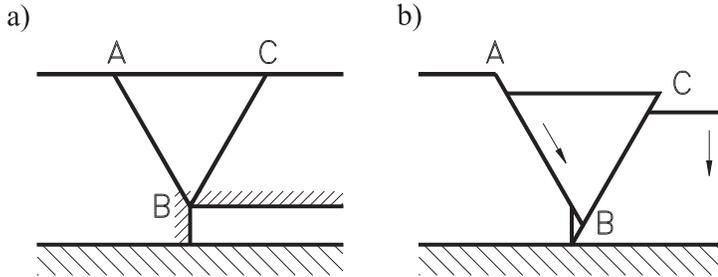
FIG. 1. Simple mechanism of terrain subsidence; a) initial configuration, b) configuration after the right-hand segment of the bedrock has been moved downwards.
