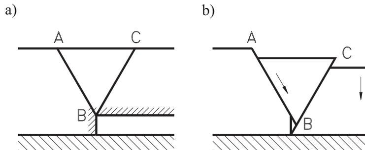
FIG. 3. Simple mechanism of terrain subsidence caused by underground exploitation;
