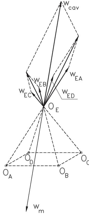
FIG. 21. Procedure of determining the displacement vector  $\mathbf{w}_m$  of granular medium, caused by three-dimensional migration of cavities.
