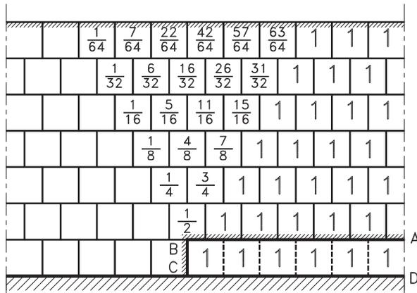
FIG. 12. The assumed system of finite cells for the analysis of the terrain subsidence. The initial long cavity  $A - B - C - D$  has been divided into six cells, each of a unit volume. Numbers in particular cells indicate what portion of a unit cavity has passed through each cell in the migration process towards the upper surface.
