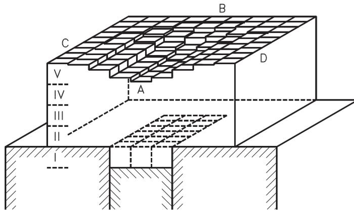
FIG. 18. Calculated subsidence of the upper surface of the bulk caused by tectonic displacement of a long narrow portion of the bedrock. The empty space formed by the end part of the displaced bedrock has been divided into 18 cells, each of a unit volume.
