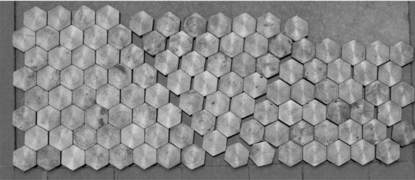
FIG. 5. Experimental simulation of the deformation mode shown in Fig. 3; a) – initial configuration of coins located on the glass plate in horizontal position, b) – final configuration after the plate was inclined with respect to horizontal position.
