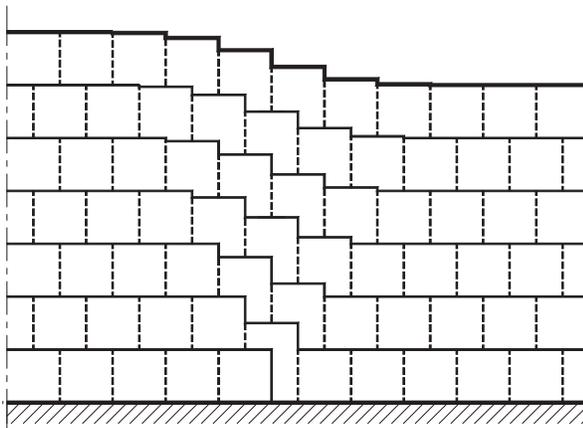
FIG. 13. Stepwise approximation of the terrain subsidence in the case shown in Fig. 12.
