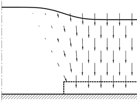
FIG. 14. Calculated displacements of the granular medium after migration of the cavity  $A - B - C - D$  towards the upper surface of the medium.
