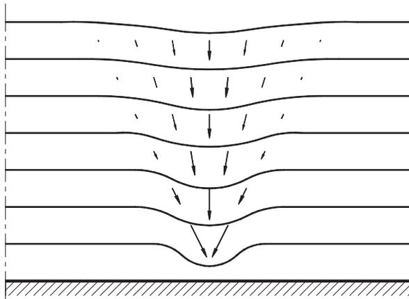
FIG. 11. Calculated displacements of granular medium after migration of a unit cavity, located initially as shown in Fig. 8.
