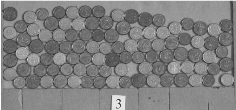
FIG. 6. Experimental simulation of the gravity walk of the particles of a granular medium; a) initial configuration of coins of different diameters located on a glass plate in its horizontal position, b) final configuration after the blocking strip at the bottom has been removed and the plate has been inclined with respect to the initial horizontal position.
