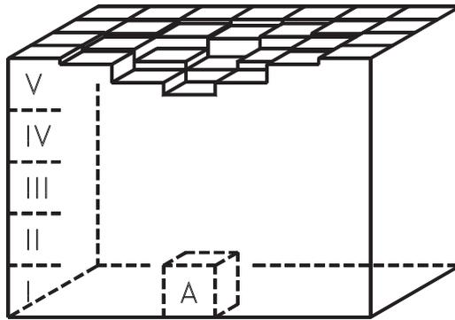
FIG. 15. Stepwise approximation of the deformation of the upper surface of a granular medium caused by migration of cavity  $A$  of unit volume. Vertical displacements have been enlarged five times. The frontal part of the bulk has not been shown.
