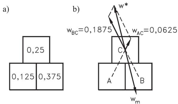
FIG. 10. Procedure of determining the displacement vector  $w_m$  of a granular medium caused by the migration of a cavity upwards.
