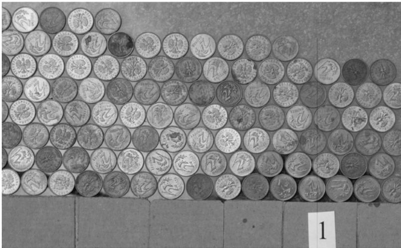
FIG. 4. Experimental simulation of the deformation mode shown in Fig. 3; a) initial configuration of coins located on the glass plate in horizontal position, b) final configuration after the plate was inclined with respect to horizontal position.
