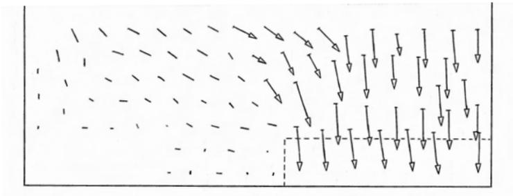
FIG. 7. Measured displacements of coins simulating particles of a granular medium in the test shown in Fig. 6.
