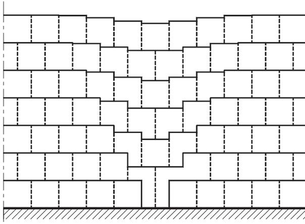
FIG. 9. Stepwise approximation of the deformation mode, caused by migration upwards of the unit cavity at the bottom.
