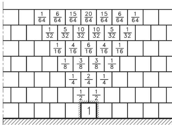
FIG. 8. The assumed system of finite cells for the analysis of migration of a unit cavity at the bottom according to an assumed, simple stochastic rule. Numbers in cells indicate which fraction of the cavity passed through the cell.
