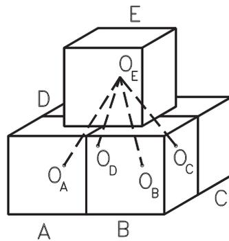
FIG. 20. Local configuration of five cells taken from the assumed system of finite cells for calculation of the displacement vector.
