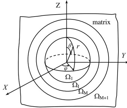
FIG. 1. A spherical inhomogeneity with multi-shells embedded in an infinite medium.
