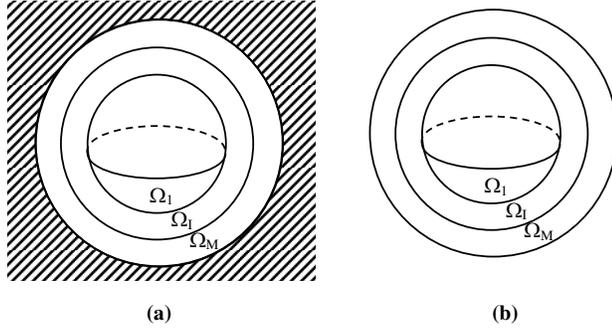
FIG. 2. A spherical inhomogeneity containing multi-shells with fixed exterior boundary (a) and traction-free exterior boundary (b).
