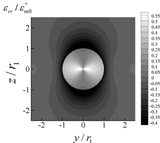
FIG. 6. Strain distribution in a non-uniform spherical QD embedded in an infinite matrix with a constant interface stress  $\sigma_0^s = 1\text{N/m}$ .
