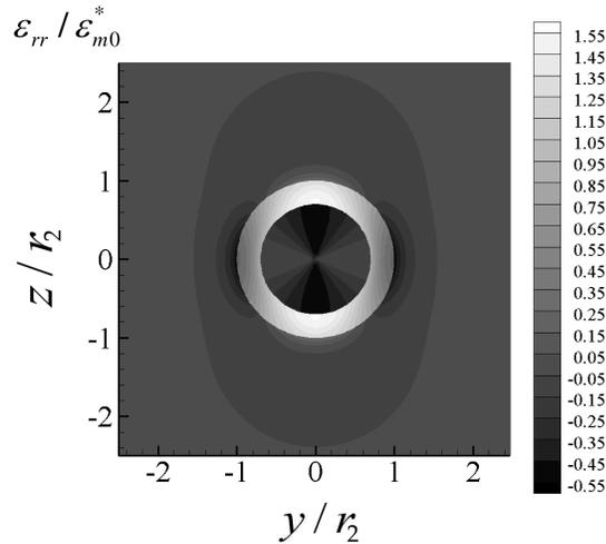
FIG. 5. Strain distribution in a spherical uniform nano-onion with one shell ( $M = 2$ ) embedded in an infinite matrix with a constant interface stress  $\sigma_0^s = 1\text{N/m}$ .
