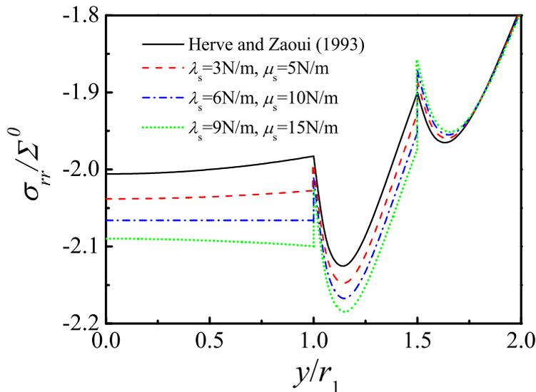
FIG. 4. Stress distribution in a spherical uniform nano-particle with one shell ( $M = 2$ ) embedded in an infinite matrix for different values of interface moduli  $\lambda_s$  and  $\mu_s$ .
