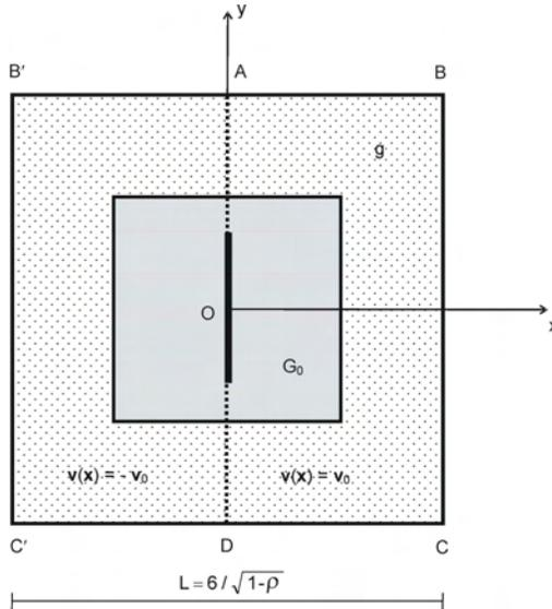
FIG. 9. Velocity field to determine  $K_R(g, \rho)$ .
