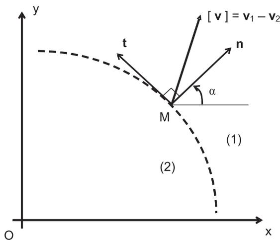
FIG. 6. Discontinuity of displacement velocity  $[\mathbf{v}]$ .
