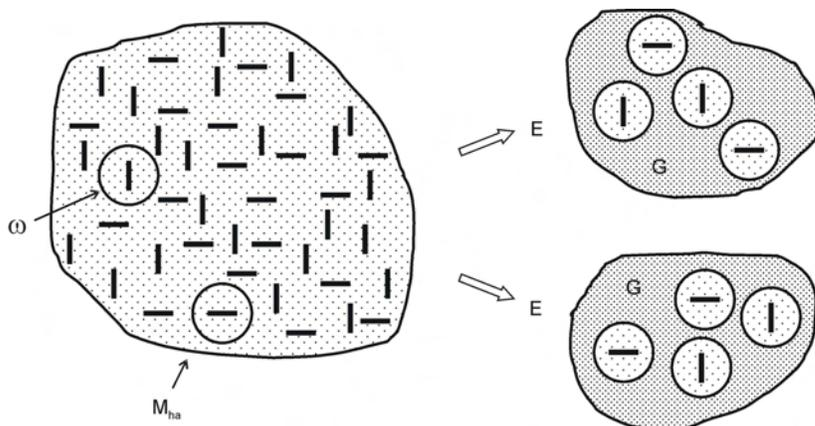
FIG. 1. Choice of inclusions representative of the heterogeneous material  $M_{ha}$  and examples of samples  $E$ .
