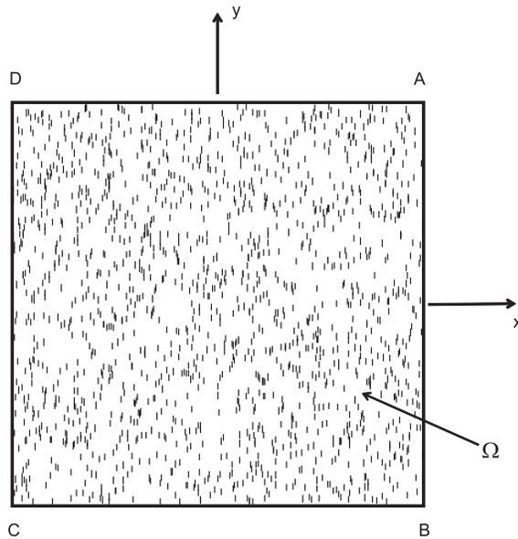
FIG. 8. A square sample composed of the defect material (comprising 1600 segments).
