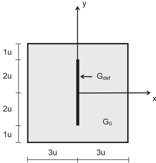
FIG. 7. Microstructure  $\mu_s$  characterizing the defect material.
