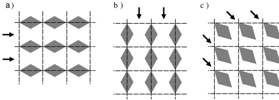
FIG. 1. Tetragonal architecture of porous medium with rotary rhomboidal fibers. Configurations of fibers for transport process in the main (a, b) and diagonal (c) directions of the pore space.
