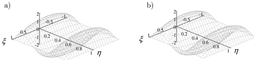
FIG. 9. Diagrams of the dimensionless intrinsic microvibration amplitude for  $\Omega = 1.1$ ,  $\Gamma = 20$  and  $f(\xi) = 0.5\sqrt{1-\xi^2}$  (Fig. 9a),  $f(\xi) = 0.5\sqrt{1-\xi^6}$  (Fig. 9b).
