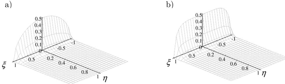
FIG. 5. Diagrams of the dimensionless intrinsic microvibration amplitude for  $\Omega = 0$ ,  $\Gamma = 20$  and  $f(\xi) = 0.5\sqrt{1-\xi^2}$  (Fig. 5a),  $f(\xi) = 0.5\sqrt{1-\xi^6}$  (Fig. 5b).
