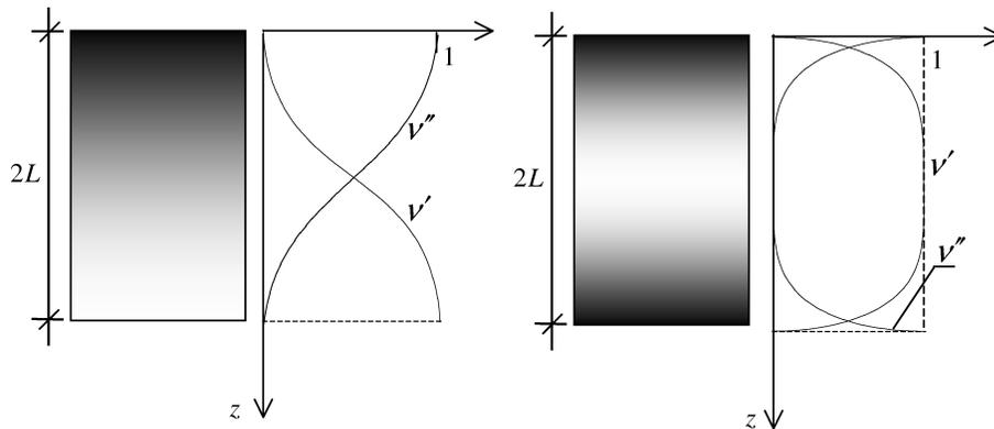
FIG. 3. Diagrams of mean volume fractions  $\nu', \nu''$  of lamina materials for two FGL solids.
