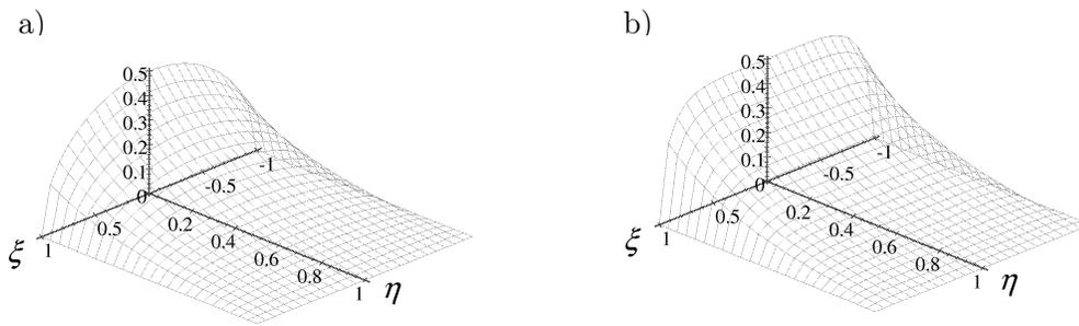
FIG. 7. Diagrams of the dimensionless intrinsic microvibration amplitude for  $\Omega = 0.99$ ,  $\Gamma = 20$  and  $f(\xi) = 0.5\sqrt{1-\xi^2}$  (Fig. 7a),  $f(\xi) = 0.5\sqrt{1-\xi^6}$  (Fig. 7b).
