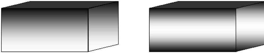
FIG. 1. Fragments of two FGL solids from the macroscopic point of view with different distributions of the effective material characteristics.
