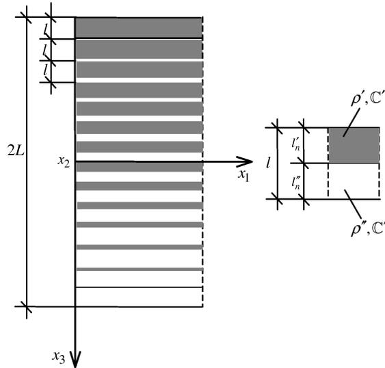
FIG. 2. A cross-section of the FGL solid and a fragment of its  $n$ -th layer.
