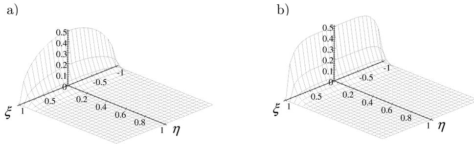
FIG. 6. Diagrams of the dimensionless intrinsic microvibration amplitude for  $\Omega = 0.01$ ,  $\Gamma = 20$  and  $f(\xi) = 0.5\sqrt{1-\xi^2}$  (Fig. 6a),  $f(\xi) = 0.5\sqrt{1-\xi^6}$  (Fig. 6b).
