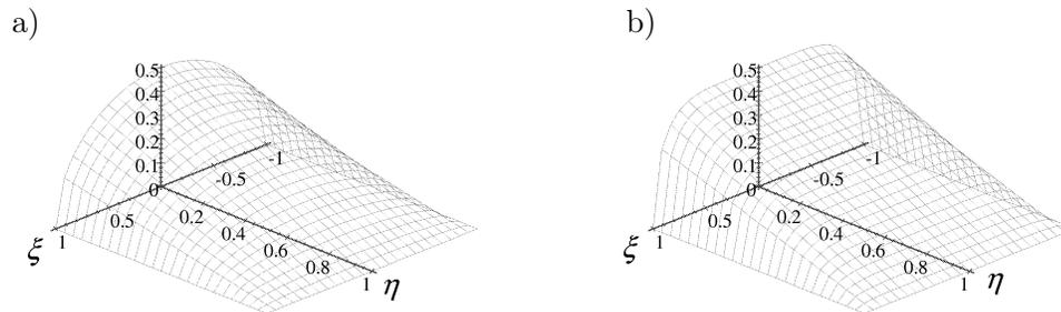
FIG. 8. Diagrams of the dimensionless intrinsic microvibration amplitude for  $\Omega = 1$ ,  $\Gamma = 20$  and  $f(\xi) = 0.5\sqrt{1-\xi^2}$  (Fig. 8a),  $f(\xi) = 0.5\sqrt{1-\xi^6}$  (Fig. 8b).
