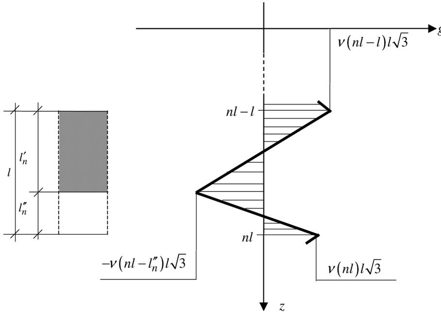
FIG. 4. A diagram of the fluctuation shape function in the  $n$ -th layer.
