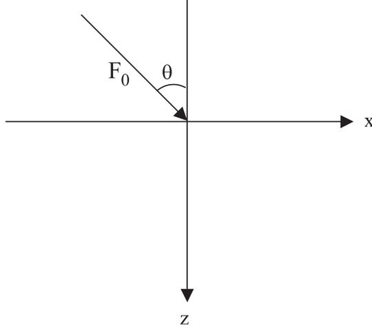
FIG. 1. Inclined load over a thermoelastic half-space with voids.
