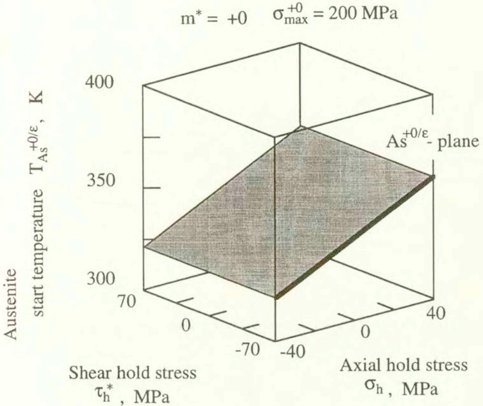
FIG. 9. Austenite start plane after tensile pre-stressing.
