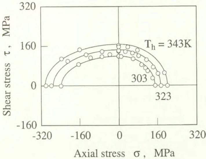
FIG. 2. Martensite start stresses during proportional loading; martensite start curves.
