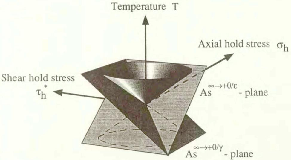
FIG. 26. Austenite start cone in stress-temperature space.
