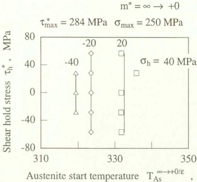
FIG. 16. Effect of shear hold stress on austenite start temperature after successive pre-stressing  $m^* = \infty$  and  $m^* = +0$ .
