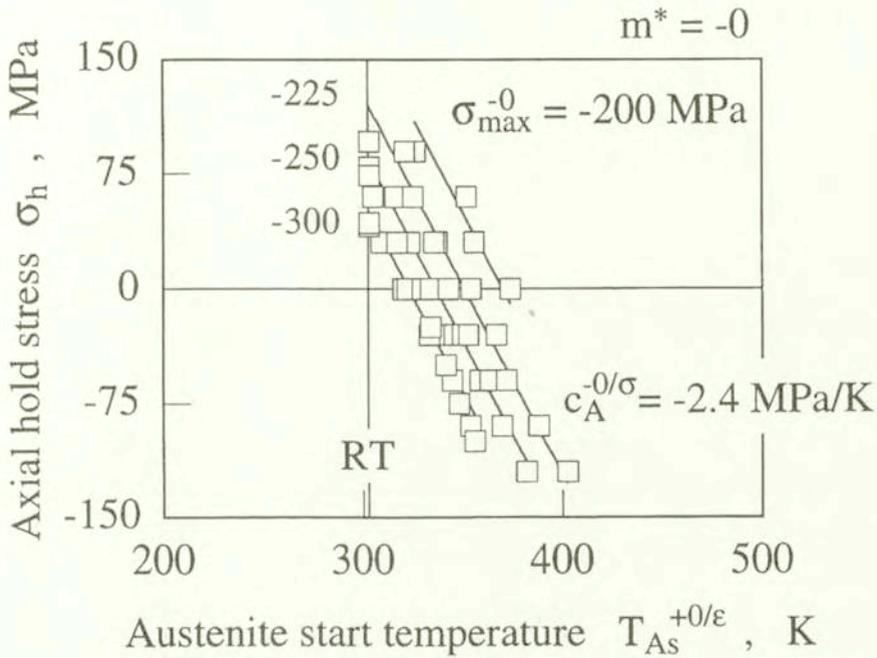
FIG. 6. Austenite start lines after compressive pre-stressing.
