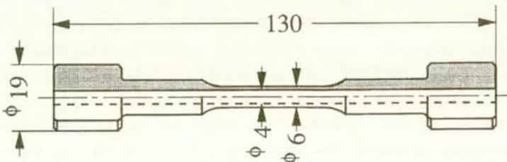
FIG. 1. Test specimen.
