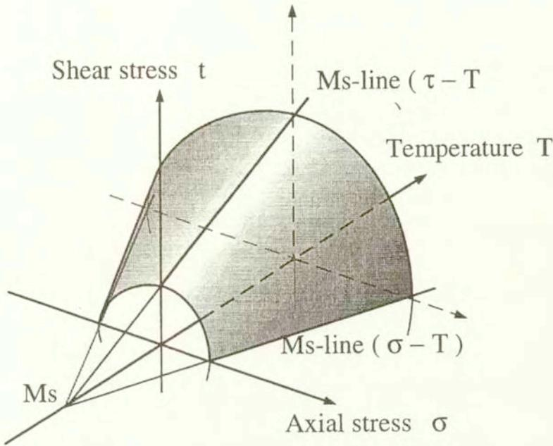
FIG. 4. Martensite start cone in stress-temperature space (Schematic).
