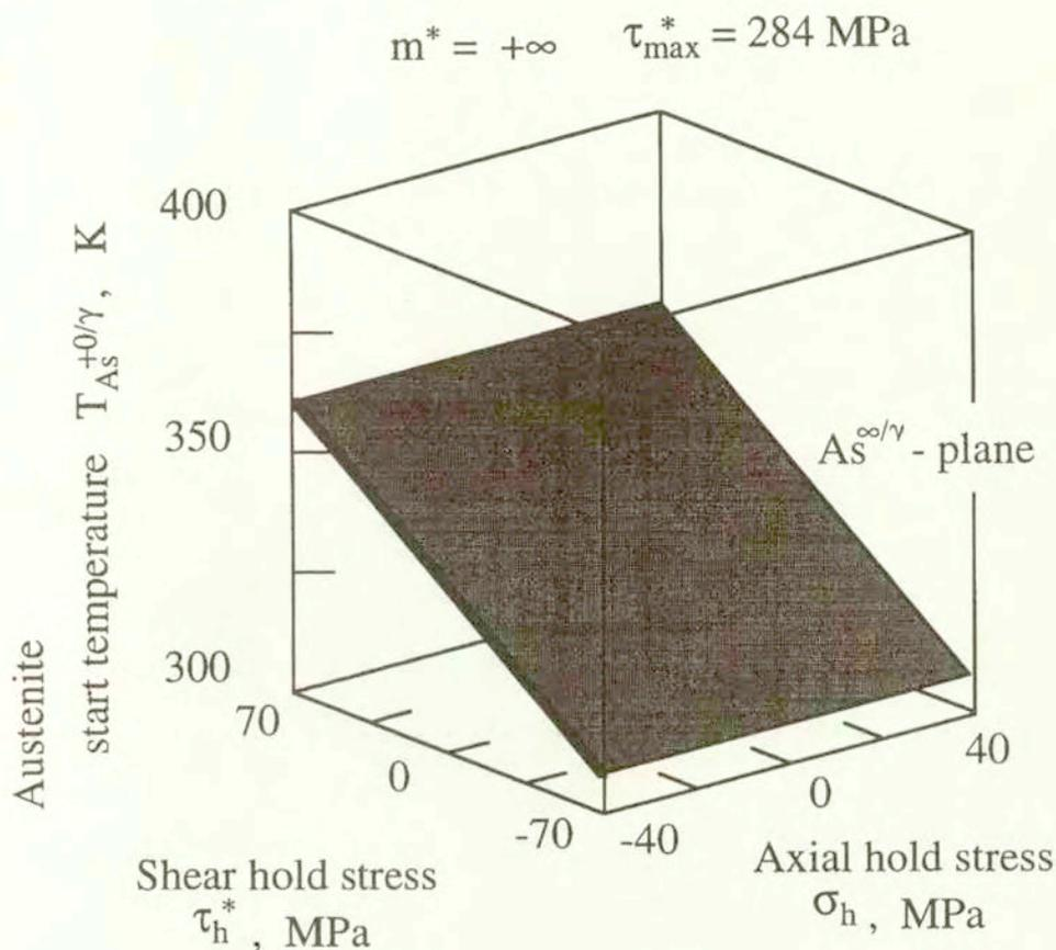
FIG. 12. Austenite start plane after shear pre-stressing.
