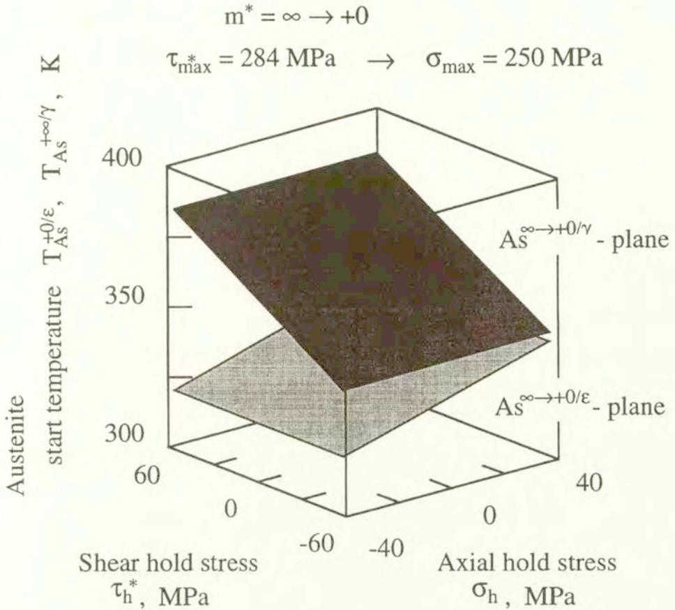
FIG. 19. Austenite start planes after successive pre-stressing  $m^* = \infty$  and  $m^* = +0$ :  $As^{\infty \rightarrow +0/\epsilon}$ -plane is lower in location than  $As^{\infty \rightarrow +0/\gamma}$ -plane.
