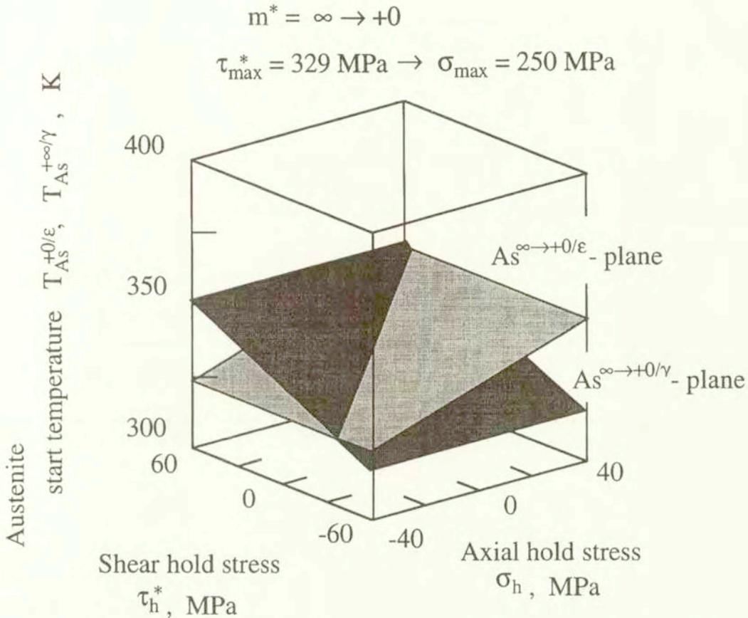
FIG. 22. Austenite start planes after successive pre-stressing  $m^* = -\infty \rightarrow m^* = +0$ :  $As^{\infty \rightarrow +0/\gamma}$  -plane translates down, and intersects with  $As^{\infty \rightarrow +0/\epsilon}$  -plane.
