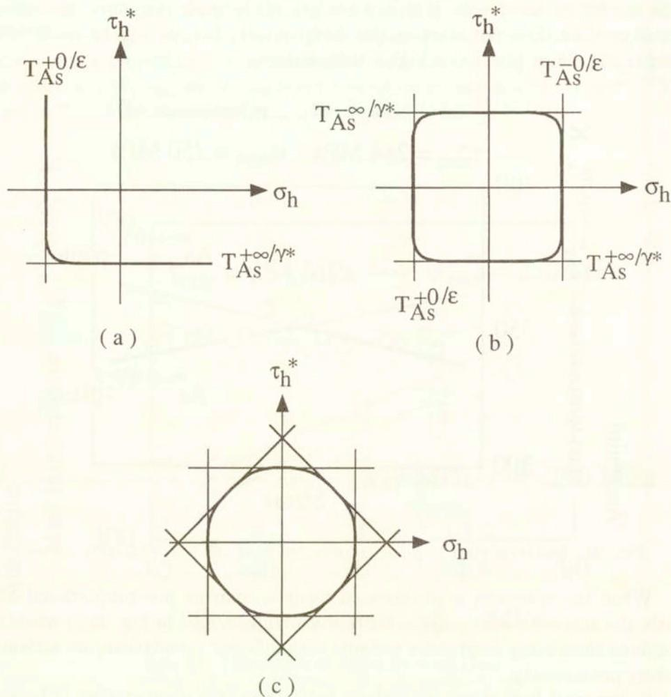
FIG. 25. Austenite start condition on stress plane.
