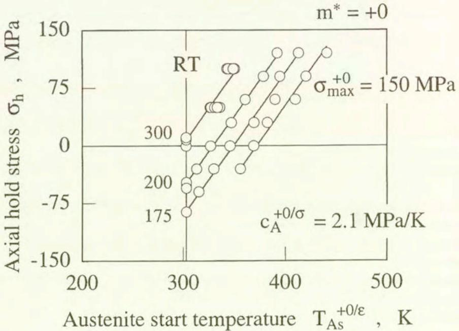
FIG. 5. Austenite start lines after tensile pre-stressing.
