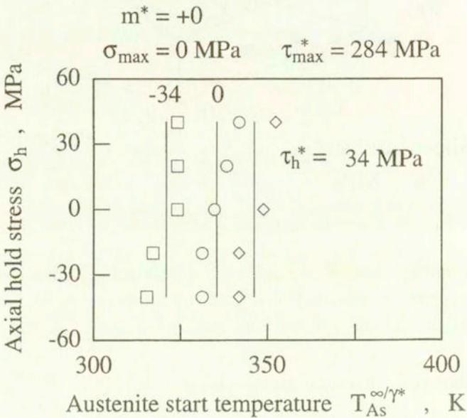
FIG. 11. Effect of axial hold stress on austenite start temperature: case of shear pre-stressing.
