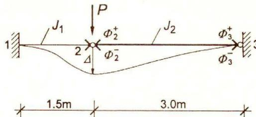
FIG. 1. Slackened beam with clearance hinges.
