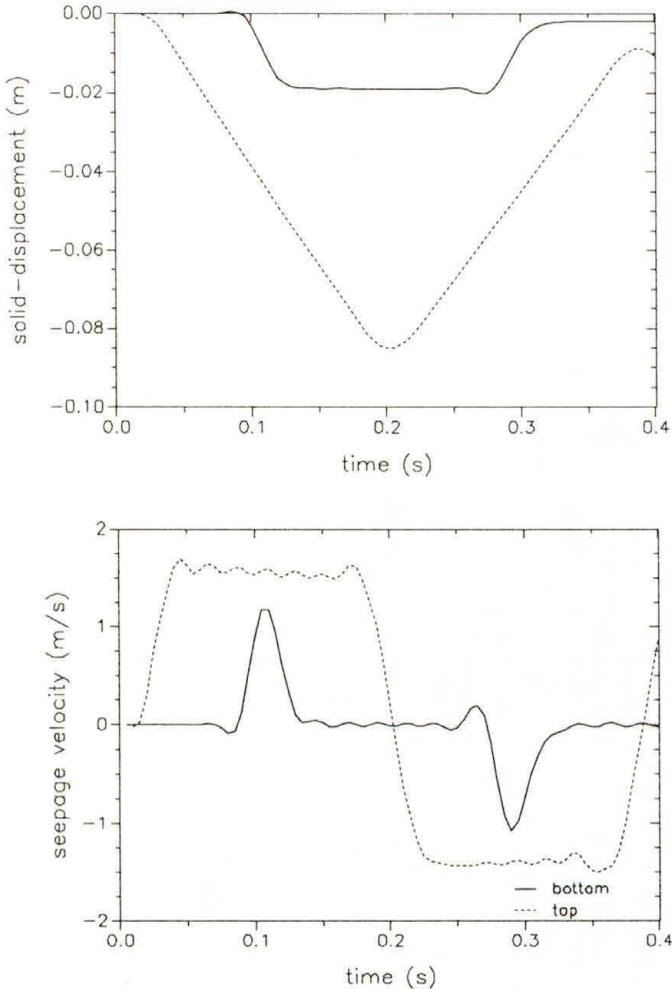
FIG. 5. Solid displacement and seepage velocity versus time.
