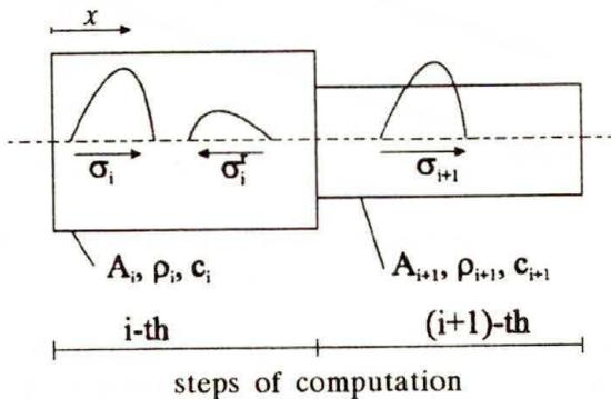
FIG. 10. Partial reflection at the element boundary.
