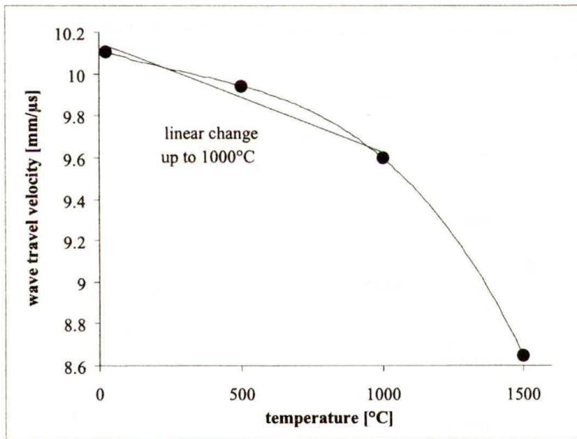
FIG. 6. Temperature dependence of the wave velocity.
