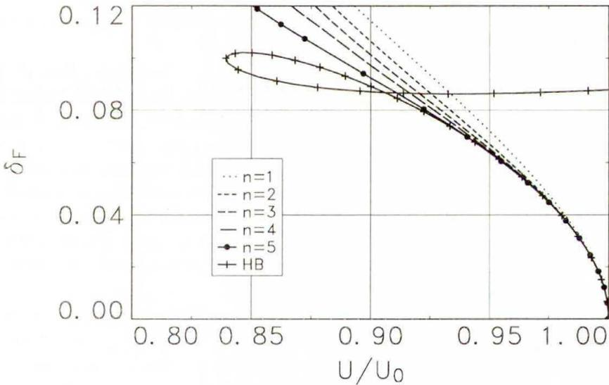
FIG. 7. Flap limit cycle amplitude (antisymmetric flutter).
