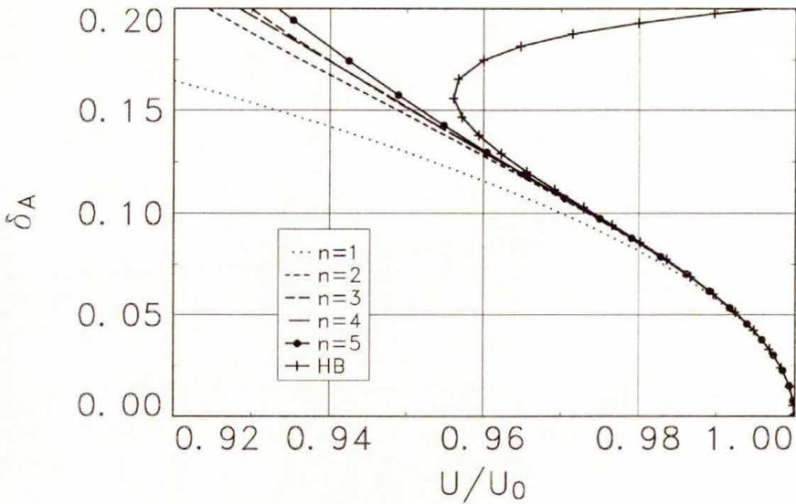
FIG. 4. Aileron limit cycle amplitude (symmetric flutter).
