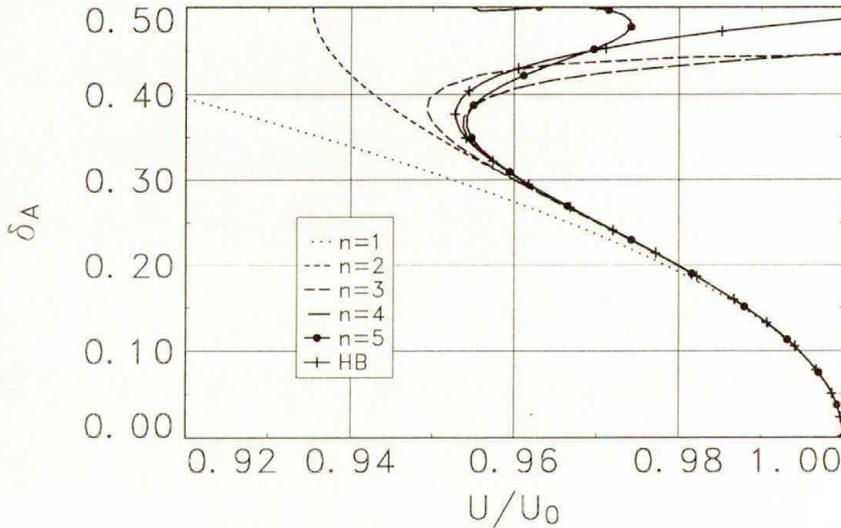
FIG. 12. Aileron limit cycle amplitude (antisymmetric flutter).
