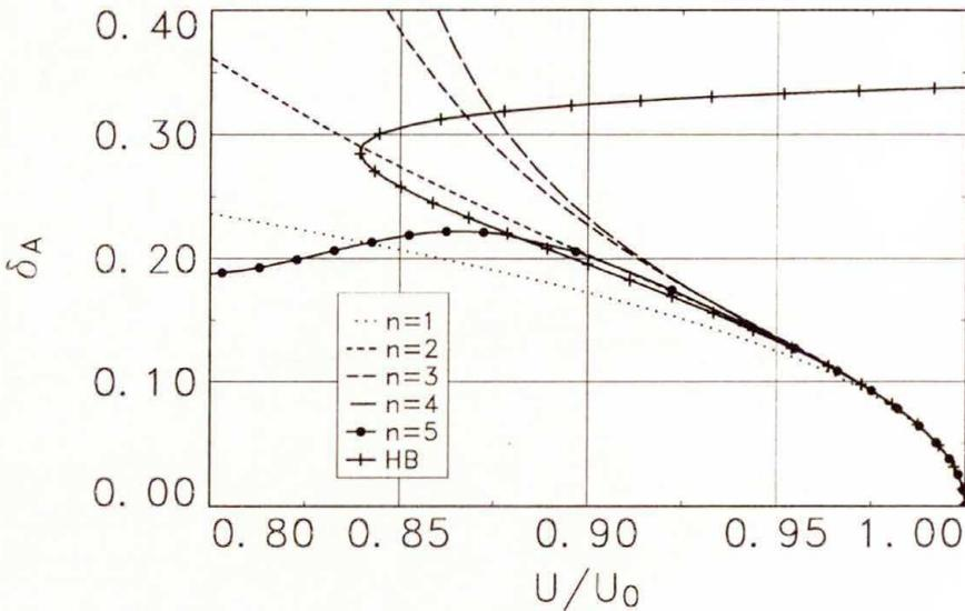
FIG. 8. Aileron limit cycle amplitude (antisymmetric flutter).
