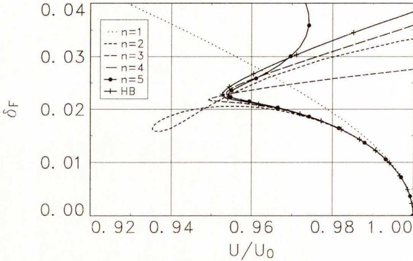
FIG. 11. Flap limit cycle amplitude (antisymmetric flutter).
