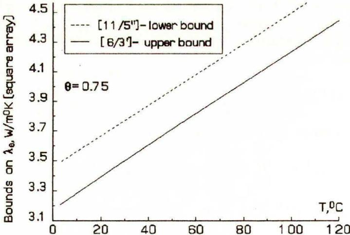
FIG. 8. Upper and lower bounds on the effective conductivity for square array of cylinders (epidian 53,  $\lambda_1 = 0.21 + 0.005T$ ), embedded in a matrix (steel 15NiCuMoNb5,  $\lambda_2 = 37.25 + 0.048T$ ), cf. [44].
