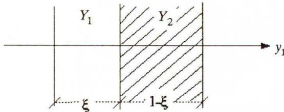
FIG. 1. Basic cell for two-phase layered composites.
