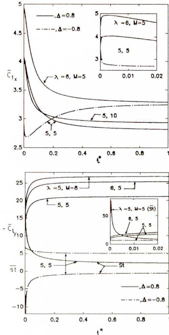
FIG. 3. Effects of rotation ( $\lambda$ ), and magnetic parameter ( $M$ ) on skin frictions and heat transfer ( $\bar{C}_{f_x}$ ,  $-\bar{C}_{f_y}$ ,  $\bar{St}$ ) for  $f_w = 0$ ,  $\omega = 0.5$  and  $g_w = 1.4$ ; (unsteadiness due to impulsive change in wall enthalpy).
