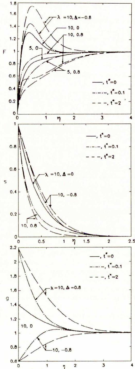
FIG. 5. Effects of rotation ( $\lambda$ ) and time ( $t^*$ ) on the velocity and enthalpy ( $F, s, g$ ) profiles for  $M = 5$ ,  $f_w = 0.0$ ,  $g_w = 1.4$  and  $\omega = 0.5$ ; (unsteadiness due to impulsive change in wall enthalpy).
