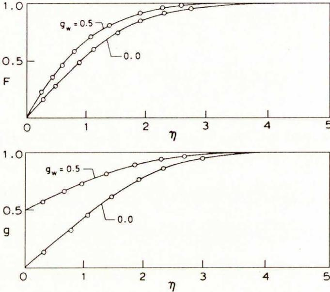
FIG. 2. Comparison of velocity ( $F$ ) and enthalpy ( $g$ ) profiles with the results of VIMALA and NATH [10] for  $t^* = 0$ ,  $Pr = 0.72$ ,  $\omega = 1$ ,  $f_w = 0$ ,  $\lambda = 0$ ,  $M = 0$ ;  $\circ$  results due to Ref. [10]; — present study.
