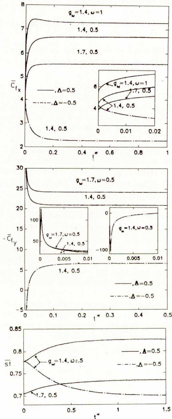
FIG. 6. Effects of wall enthalpy ( $g_w$ ) and viscosity-index ( $\omega$ ) on skin frictions and heat transfer ( $\bar{C}_{f_x}$ ,  $-\bar{C}_{f_y}$ ,  $\bar{St}$ ) for  $f_w = 0$ ,  $M = 5$  and  $\lambda = 6$ ; (unsteadiness due to impulsive change in rotation).
