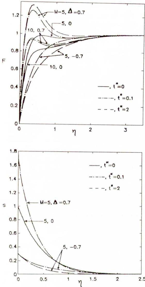
FIG. 7. Effects of magnetic parameter ( $M$ ) and time ( $t^*$ ) on the velocity ( $F, s$ ) profiles for  $f_w = 0, g_w = 1.4, \lambda = 7$  and  $\omega = 0.5$ ; (unsteadiness due to impulsive change in rotation).
