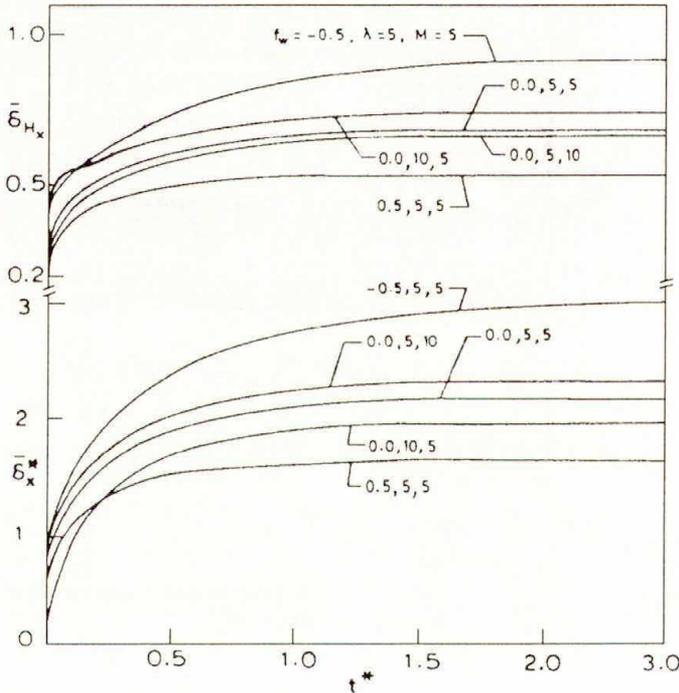
FIG. 4. Effects of mass transfer ( $f_w$ ), rotation ( $\lambda$ ), and magnetic parameter ( $M$ ) on displacement and enthalpy thickness  $[\delta_x^*, \delta_{H_x}]$  for  $\Delta = 0.8$ ,  $\omega = 0.5$  and  $g_w = 1.4$ ; (unsteadiness due to impulsive increase in wall enthalpy).
